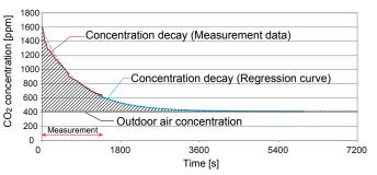
Fig. 27 CALCULATION OF LOCAL MEAN AGE OF AIR BASED ON MEASURED CO2 CONCENTRATION
