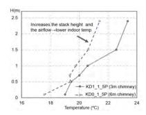
Fig. 17 SHORT-TERM MEASUREMENTS : IMPACT OF CHIMNEY HEIGHT ON INDOOR AIR TEMPERATURE.
