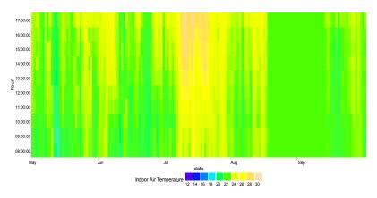
Fig. 19 indoor air temperature heatmap Room B294  $$\rm May-September\ 2013$
