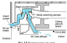
Fig.13 SCHEMATIC OF THE NV INLET DIFFUSER
