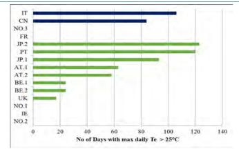
Figure 4: No of days with maximum daily external temperature above 25°C (Residential shown in Blue)
