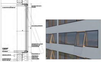
Fig. 9 Custom-Made top-hung projecting-out Windows, Source: Passivhaus Institut
