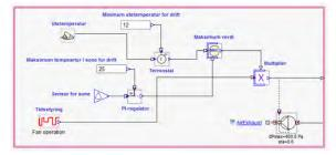
Fig. 10 EXHAUST VENTILATION CONTROL
