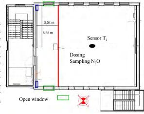
Fig. 17 Test set up tracer gas measurement
