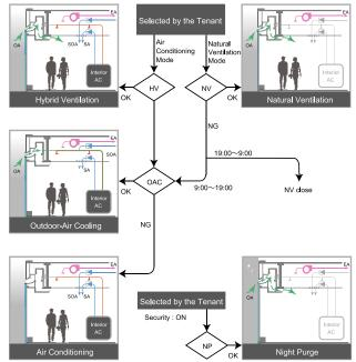
Fig. 18 AUTOMATED VENTILATOR AND AHU CONTROL FLOWCHART
