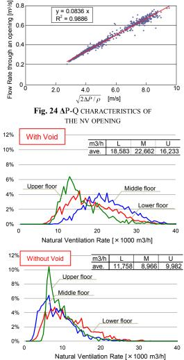
Fig. 25 HISTOGRAM OF THE NATURAL VENTILATION RATE FOR THE CASES WITH/WITHOUT THE VOIDS
