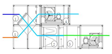
1.Fresh air 2.Filter 3.Surface Cooler 4.Exhaust fan 5.Air exhaust
