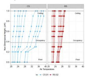
Fig. 22 STRATIFICATION IN EXISTING & RETROFIT BLDG
