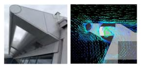
Fig. 23 DETAIL DESIGN STAGE SIMULATION: AIR FLOW OF EXHAUST OPENING
