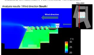
Fig. 22 DETAIL DESIGN STAGE SIMULATION: INDOOR THERMAL ENVIRONMENT FOR NATURAL VENTILATION
