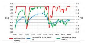
Fig. 14 TEMPERATURES VERSUS WINDOW OPENING
