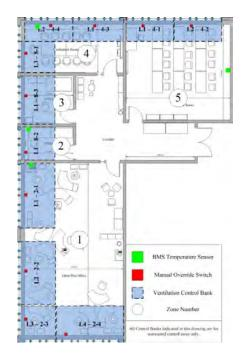
Fig. 12 AUTOMATED LOUVRE BANK CONTROL SECTIONS
