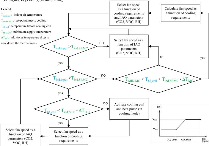
Fig. 11 CONTROL STRATEGY. BOTTOM RIGHT: VARIATION OF THE VOLUMETRIC FLOW RATE AS A FUNCTION OF CO2 CONCENTRATION LEVEL
