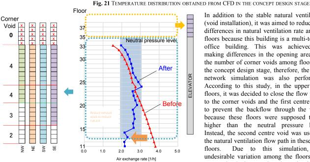
Fig. 22 CONCEPT DESIGN STAGE SIMULATION (FLOW NETWORK CALCULATION)
