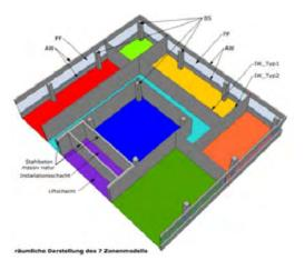
Fig. 12 DESIGN STAGE SIMULATION OF RETROFITED BUILDING USING DYNBIL, SOURCE: PASSIVHAUS INSTITUT.
