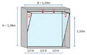
Fig. 18 Test set up and air velocity measurement (position of the sensors)
