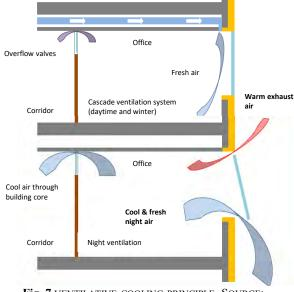
Fig. 7 ventilative cooling principle, Source: Passivhaus Institut, Edited: e7
