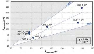
Fig. 13 Bulk Airflow rate results: measured vs simulated.
