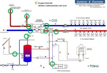
Fig. 7 SCHEME OF THE HVAC SYSTEM WITH MONITORING POINTS (GREEN CIRCLES)
