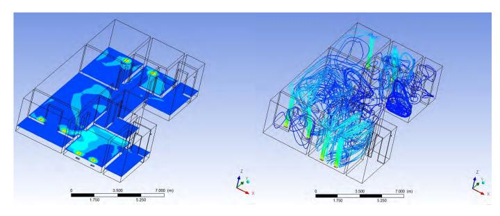
Fig. 13 Operation stage simulation: temperature field & Air distribution
