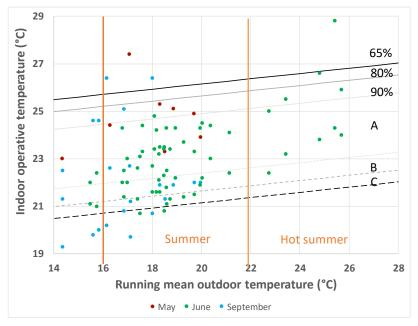
Fig. 25 EVALUATION ADAPTIVE TEMPERATURE LIMITS METHOD
