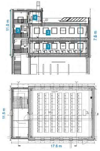
Fig 4. TOP IMAGE IS THE SECTION OF THE TWO LECTURE ROOMS. BOTTOM FIGURE IS THE FLOOR PLAN OF ONE LECTURE ROOM.
