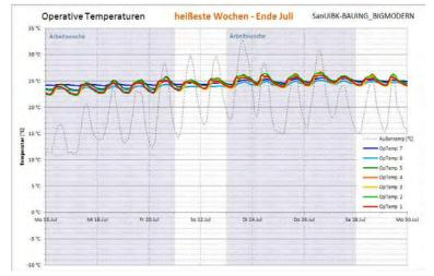
Fig. 14 ZONE TEMPERATURES DURING HOTTEST WEEKS IN JULY, RESULTS FROM DESIGN STAGE SIMULATION, SOURCE: PASSIVHAUS INSTITUT
