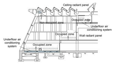
Fig. 19 AIR CONDITIONING FOR OCCUPIED ZONE OF ATRIUM
