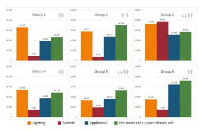
Fig. 7 DETAIL OF ENERGY CONSUMPTION OF DIFFERENT HOUSEHOLDS LIVING IN THE LIVING LAB (SKEIE, 2016)
