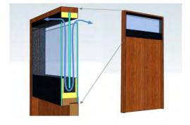
Fig. 8 CUSTOM-MADE AIRFLOW OPENINGS, SOURCE: PASSIVHAUS INSTITUT
