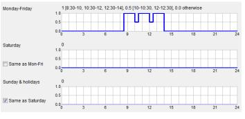
Fig. 18 TYPICAL HEATING AND COOLING SEASON OCCUPANCY PROFILES
