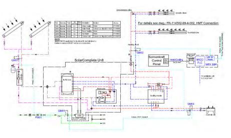
Fig.7 hydraulic scheme of heating and hot water system
