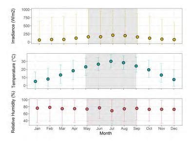
Fig.2 MEAN, MAXIMUM AND MINIMUM EXTERNAL CONDITIONS IN CHANGSHA
