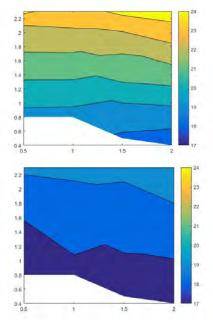
Fig. 20 air temperature profile in the room at the start (above) and after 60 min for cross ventilation
