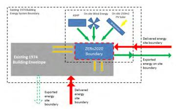
Fig.8 Schematic description of zero2020 testbed infrastructure
