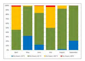
Fig. 16 PERCENTAGE OF OCCUPANCY HOURS ABOVE THRESHOLD VALUES FOR INTERNAL TEMPERATURES IN ROOM 701 DURING 2015
