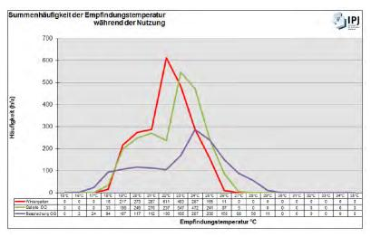
Fig. 15 CUMULATIVE FREQUENCY OF FELT TEMPERATURES DURING OCCUPANCY HOURS PER YEAR, RESULTS FROM DESIGN STAGE SIMULATION, SOURCE: IPJ INGENIEURBÜRO P. JUNG GMBH
