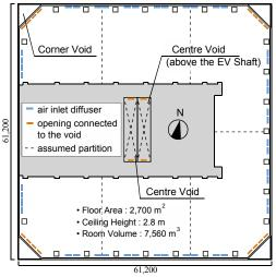
\*Slits are also provided at the ceiling to allow the air to flow into the centre void through plenum space. Fig.8 TYPICAL FLOOR PLAN OF TOWER B
