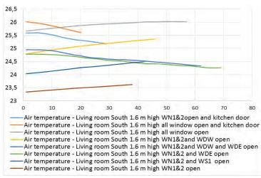
Fig. 15 INDOOR AIR TEMPERATURE IN SOUTHERN LIVING ROOM WITH NATURAL VENTILATION AS A FUNCTION OF TIME (MINUTES) LIVING LAB, TRONDHEIM, NORWAY
