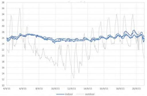
Fig. 15 INDOOR AND EXTERNAL AIR TEMPERATURE – 4<sup>TH</sup> -21<sup>ST</sup> SEPTEMBER 2015
