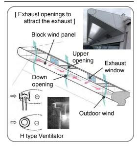
Fig. 17 SCHEMATIC DIAGRAM OF EXHAUST OPENING
