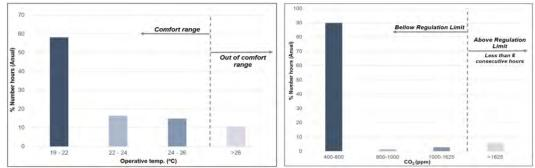
Fig. 14 Annual statistical analysis: indoor air temperature and  $\mathrm{CO}_2$  concentration
