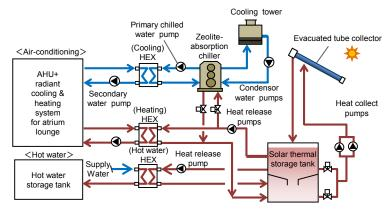
Fig. 8 MULTI-USE SOLAR HEATING AND COOLING SYSTEMS
