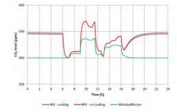
Fig. 21 Mean  $CO_2$ -level distribution in Agora for all three models throughout a day of synthetic summer climate.
