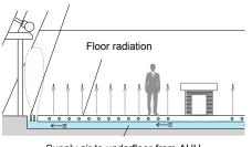
Supply air to underfloor from AHU Fig. 20 1F & 4F AIR CONDITIONING SYSTEM
