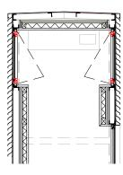
Fig. 8 CHIMNEY WITH OUTLET TOP HUNG WINDOWS
