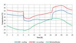
Fig. 20MEAN INDOOR TEMPERATURE DISTRIBUTION IN AGORA FOR ALL THREE MODELS THROUGHOUT A DAY OF SYNTHETIC SUMMER CLIMATE
