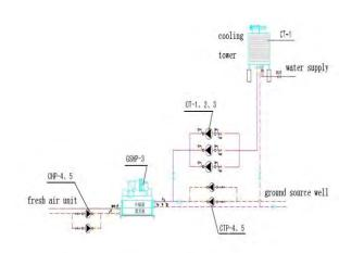
Fig. 6 PROCESS DIAGRAM OF FRESH AIR SYSTEM
