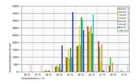
Fig. 13 TIME-WEIGHTED ZONE TEMPERATURES, DYNBIL, SOURCE: PASSIVHAUS INSTITUT.
