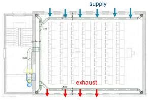
Fig. 9 PRINCIPLE OF NATURAL NIGHT VENTILATION
