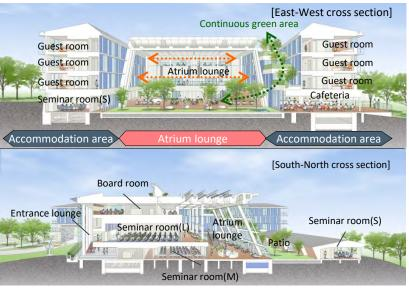
Fig 5. CROSS SECTION
