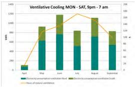
Fig. 20 Electricity consumption of VC SUPPORTING EXHAUST AIR VENTS
