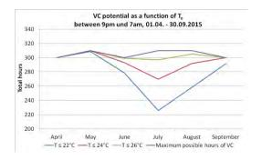
Fig. 15 POTENTIAL FOR VENTILATIVE COOLING IN INNSBRUCK IN 2015 IN RELATION TO EXTERNAL TEMPERATURE
