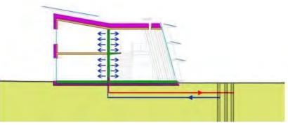
Fig.7 GEOTHERMAL HEATING AND COOLING THROUGH COMPONENT ACTIVATION, ARCHITEKTURBÜRO REINBERG ZTGMBH
