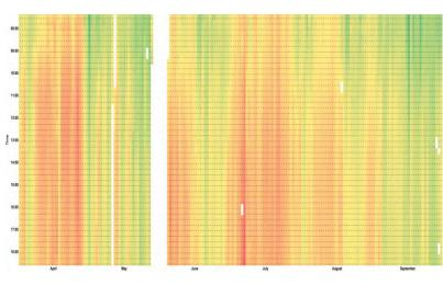
Fig. 17 INDOOR AIR TEMPERATURE PLOT IN R701 APRIL – SEPTEMBER 2015
