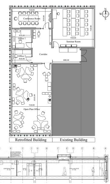
Fig 4. TOP OF IMAGE CONVEYS FLOOR PLAN OF RETROFITTED BUILDING. BOTTOM OF FIGURE ILLUSTRATES A SECTION OF THE BUILDING. The IEA project on ventilative cooling
