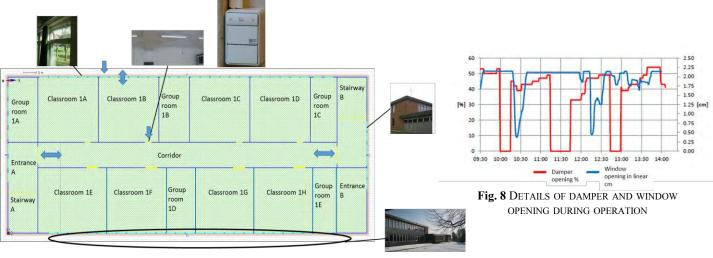
Fig. 9 Hybrid and natural Ventilation at Brunla. Motor controlled window and exhaust to a common corridor
