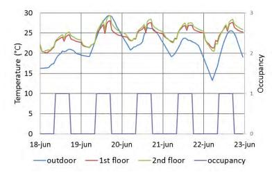
Fig. 16 INDOOR TEMPERATURES WITH NIGHT VENTILATION
