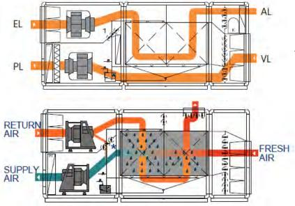
Fig. 10 Scheme of modular bypass and indirect evaporative cooling
