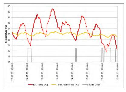
Fig. 18 INDOOR AIR TEMPERATURE PROFILE IN GALLERY, JULY 2015
