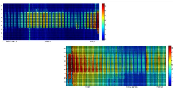
Carpet plots of building global electric consumption. The value are in kWh and refers to sampling time of 15 minutes
