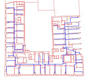
Lay-out of the refrigerant fluid tubes connecting the internal units.
