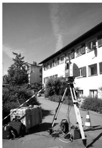
Figure 5: Laser scanning of a demonstration building (left). The measurements show a deformation of a façade of \pm 4 cm (right) that can hardly be detected by traditional measurement techniques.
