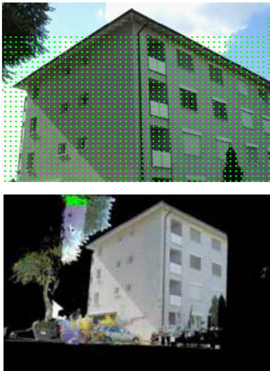
Figure 7. Visualisation of the scanning process (top) and photorealistic 3D-picture extracted from measured data (bottom).
