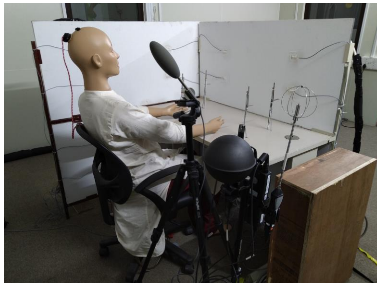
Figure 8. Laboratory experiment setup with a thermal mannequin, taken from Rawal et al. [79]
