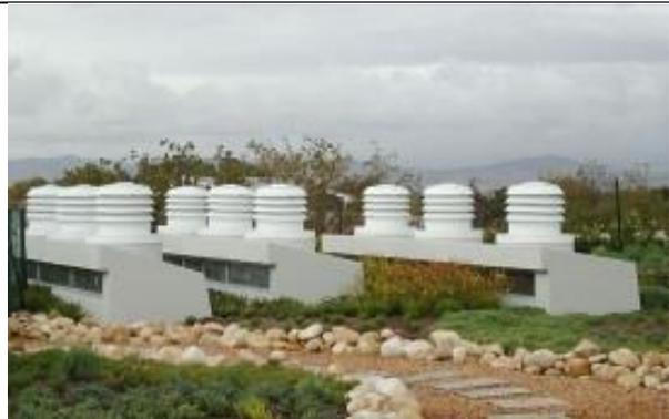
Figure 5.24. Prefab Airstract Ventilator utilizing Venturi effect. The casing is similar to the one of the windcatcher, but without inner sections. Passivent, GB. Source: [http://www.passivent.com/downloads/airstract\\_vents.pdf](http://www.passivent.com/downloads/airstract_vents.pdf)
