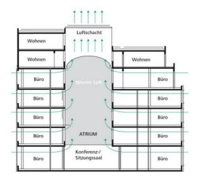
Figure 2-36: Natural ventilation via the atrium is used for night ventilation
