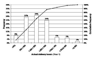
Figure 2-120: Frequency distribution of the building sample on the basis of the actual number of delivery hours for the first analysed heating season.
