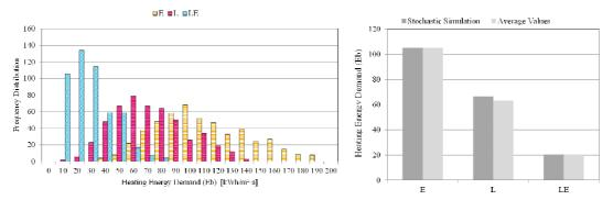
Figure 5-5: Frequency distribution of heating energy use calculated with a full building simulation and an probabilistic occupant model (left) with three different building envelopes(E=Existing building from 1970, L=Low energy house, LE=Lowest energy house). Analyzing the accuracy of the simplified model using the parameters identified with the buildings E and LE. The comparison of the case with Low energy house shows the accuracy of the model. [Experience 8]
