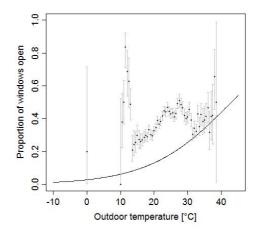
Figure 2-48: Influence of operative temperature on window opening in offices oriented to the east (summer) Figure 2-49: Influence of outdoor temperature on window opening in offices oriented to the east (summer)
