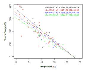
Figure 2-126: Total heat loss coefficient determined by energy signature from sub-sets of data for different levels of solar irradiation with fixed common point.(Building #3)
