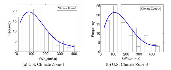
Figure 2-131: Frequency distribution and polynomial fitting plot of electricity use intensity of office building of climate zone 1 and 3 in the United States
