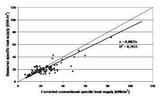
Figure 2-124: Comparison between the actual measured value and foreseen valued from  $QP_{s,c}$
