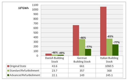
*Figure 2-140: Comparison between annual energy saving potential by applying a standard refurbishment and an advanced one to the Danish, German and Italian building stock.*
