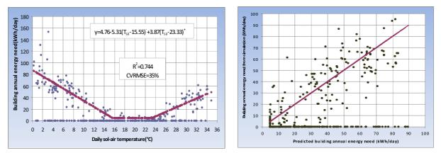
Figure 2-73: Left: Building annual energy need as a function of sol-air temperature and fit by baseline equation (5P) Right: Simulated vs predicted building annual energy need over the preretrofit period.
