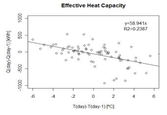
Figure 2-125: Plot for determining of  $C_{eff}$  (Building #7)
