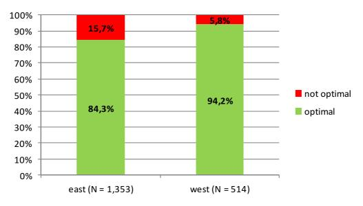
Figure 2-50: Percentages of optimal and not-optimal window opening (max. 127 minutes) based on calculations according to [9].
