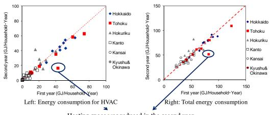
Heating space was reduced in the second year Figure 2-111: Comparison between the first year and the second year (Left: Energy consumption for HVAC; Right: Total Energy Consumption)
