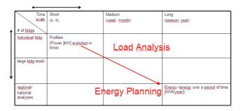
Figure 2-116. Building sample dimension vs Time frequency of energy consumptions (from hourly data to annual data)
