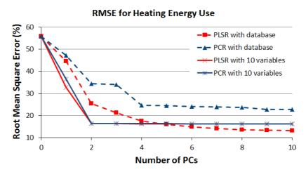
Figure 2-23: Accuracy of the heating energy use model for different amount of data and different methods
