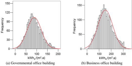
Figure 2-132: Normal distribution for electricity use intensity of office building in Japan
