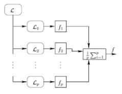
Figure 2-60: Bagging algorithm block diagram
