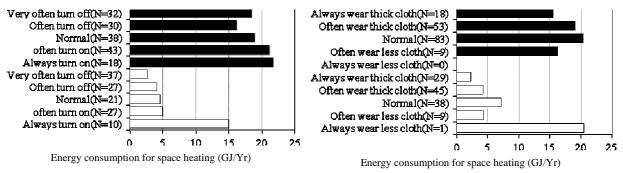
Figure 2-86: Relationship between energy consumption for space heating and usage condition of air-conditioner
