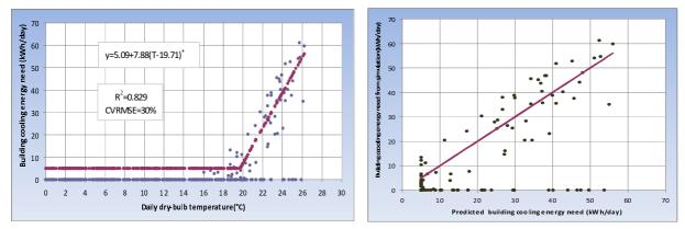
Figure 2-71: Left: Building cooling energy need as a function of dry-bulb air temperature and fit by baseline equation (3Pc) Right: Simulated vs predicted building cooling energy need over the preretrofit period.
