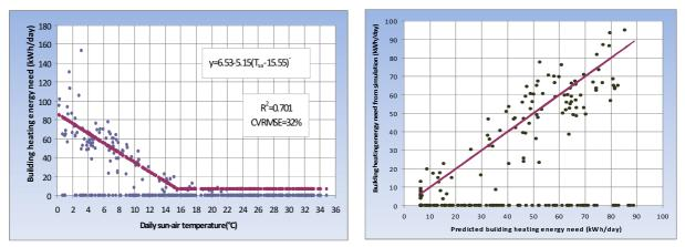
Figure 2-72: Left: Building heating energy need as a function of soil-air temperature and fit by baseline equation (3Ph) Right: Simulated vs predicted building heating energy need over the preretrofit period.
