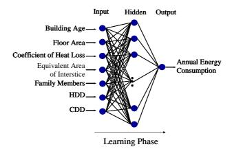
Figure 2-113: Input and output layers in neural network
