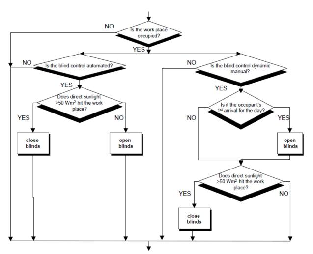
Figure 2-50: Control algorithms for manually controlled and automated blinds. Close blinds comes along with fully lowered blinds; the smallest slat angles are 00, 450 and 750 is chosen under which direct sunlight is fully blocked, [70], p. 28].
