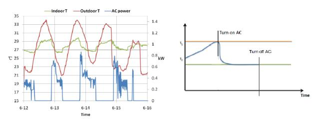
*Figure 2-38. Air conditioner operation: (a) indoor and outdoor temperature, and AC power; (b) turn-on and turn-off patterns*
