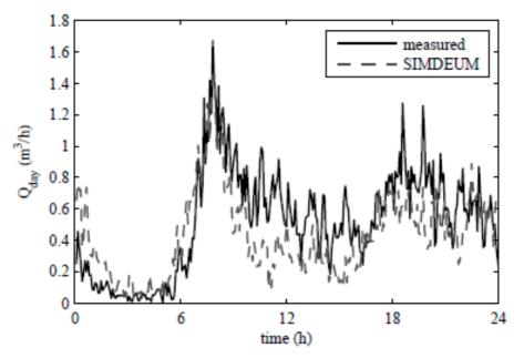
Figure 1-9: Residential water flow rate during the course of a day showing modeled and measured values based on 43 dwellings, Ref. [74].
