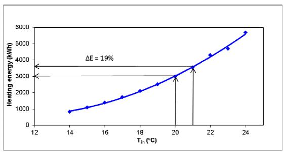
Figure 1-2: Increased sensitivity of heating energy for set point behavior. See Ref [5].
