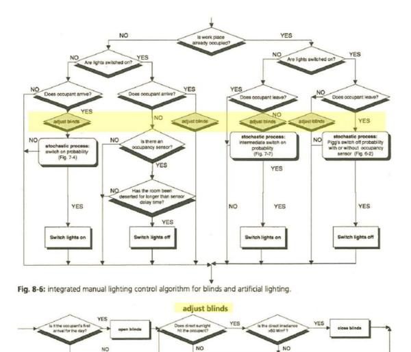
Figure 2-49: LIGHTSWITCH 2001 Model with integrated control algorithm for blinds, [[69], p. 26].
