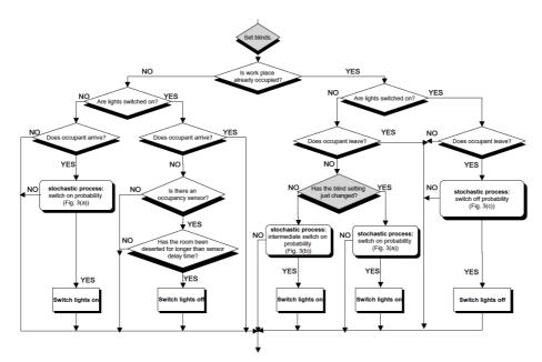
Figure 2-46. The Lightswitch-2002 algorithm for electric lighting and blinds.
