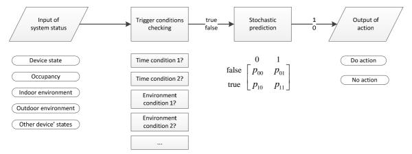
Figure 2-20. Schematic diagram of actions with trigger conditions
