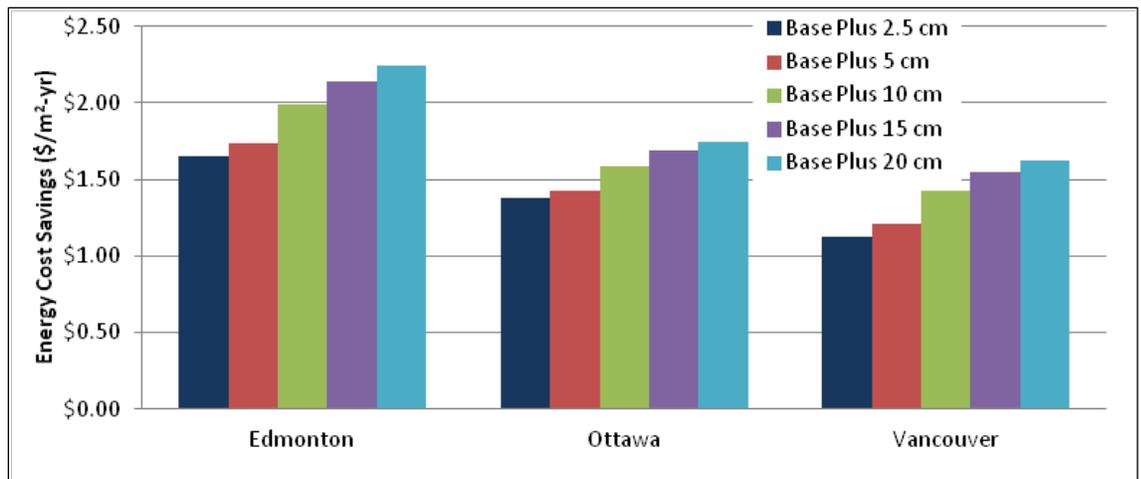
Figure 4.9. Energy cost savings for wall insulation and reduced infiltration over the Standard 90.1-1989 baseline - Canadian locations.
