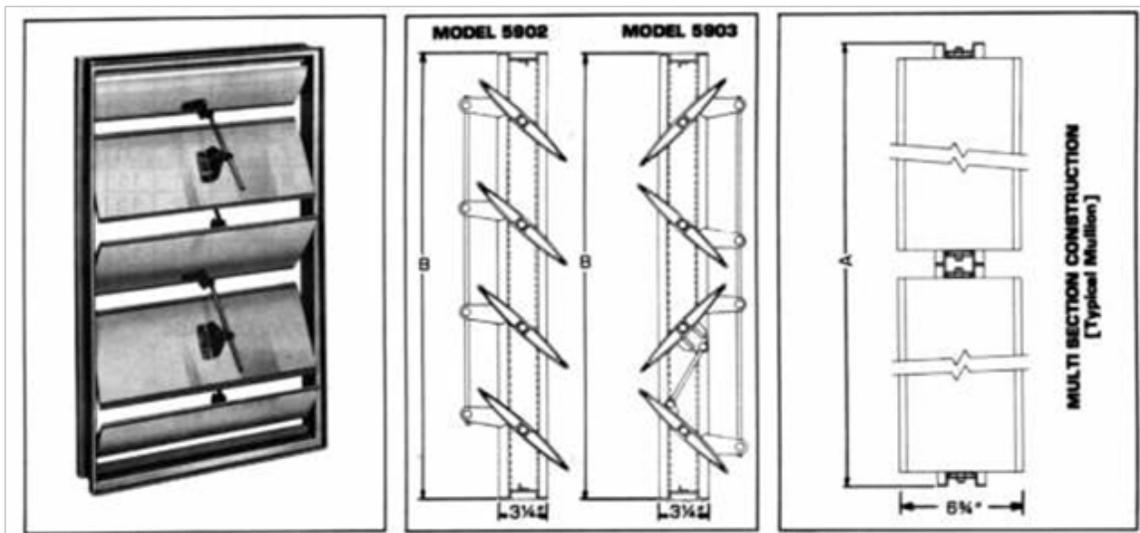
Figure 6.67. HVAC control dampers.
