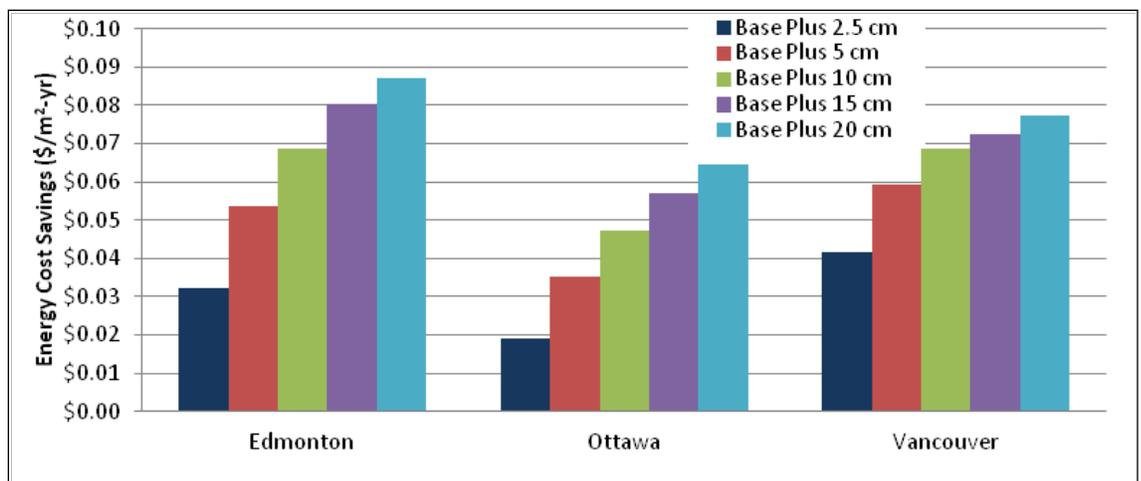
Figure 4.20. Energy cost savings for increased roof insulation and reduced infiltration over the Standard 90.1-1989 baseline – Canadian locations.
