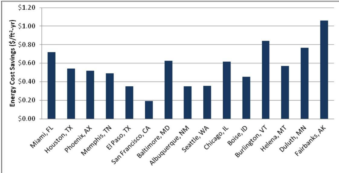
Figure 4.71. Annual energy cost savings for DOAS with radiant heating and cooling.
