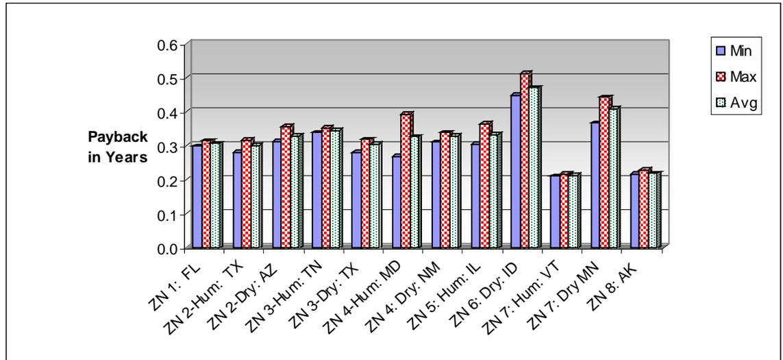
Figure 6.86. Estimated payback for 10% reduction in electric equipment use.
