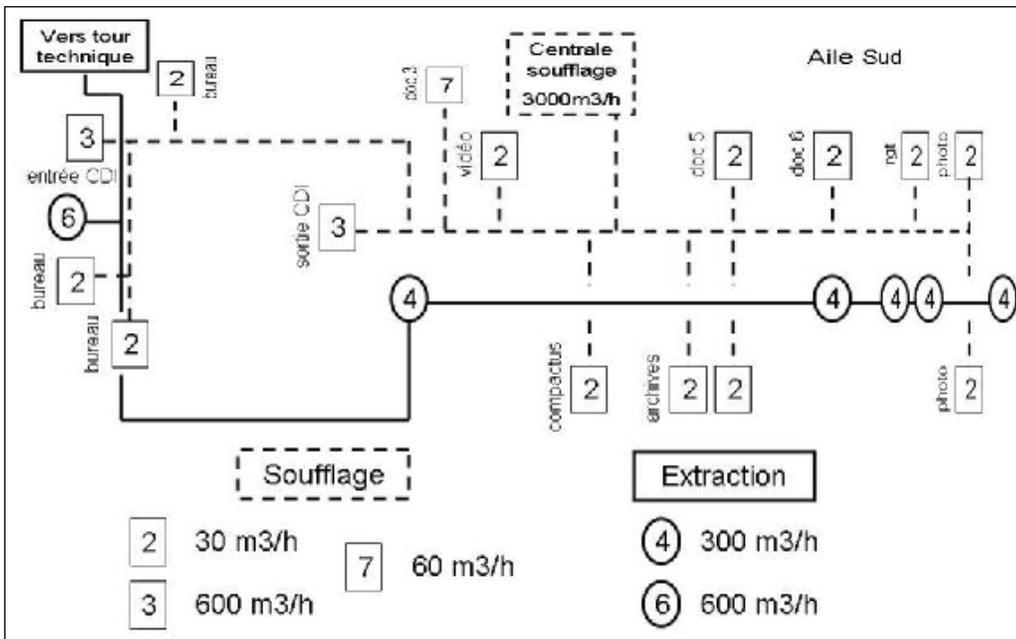
**Figure 7.86. Ventilation system configuration (first floor south).**
