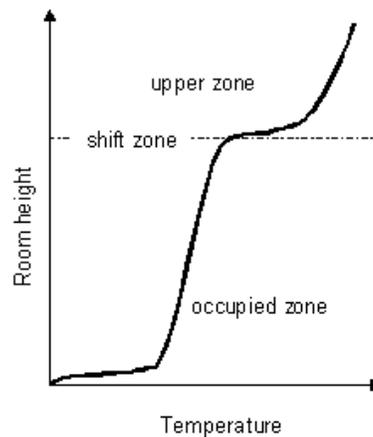
Figure 6.21. Graph illustrating temperature stratification resulting from the use of displacement air distribution.
