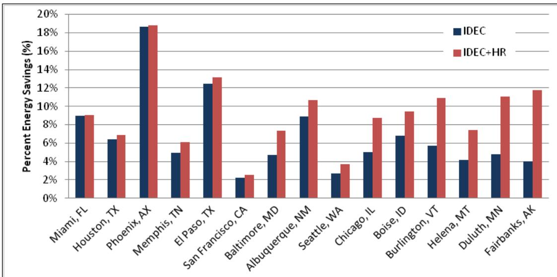
**Figure 4.153. Percent energy savings for indirect evaporative cooling and indirect evaporative cooling with heat recovery.**
