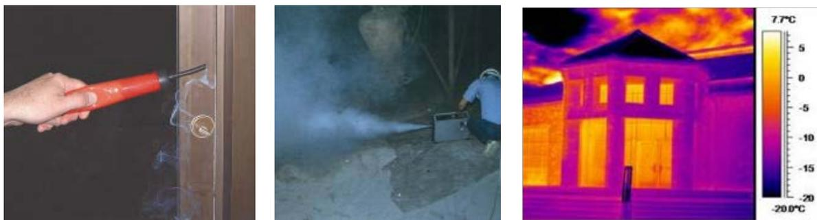
**Figure 6.118.** Smoke pencil (left) and theatrical fog (center) for leakage pathways; infrared thermography (right) for heat.
