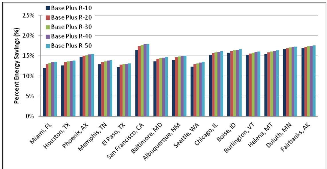
Figure 4.15. Percent energy savings for increased roof insulation and reduced infiltration over the Standard 90.1-1989 baseline.
