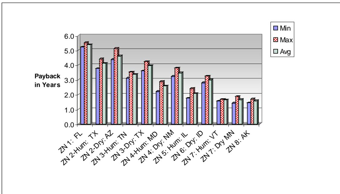
Figure 6.101. Estimated payback for 20% reduction in air flow rate.
