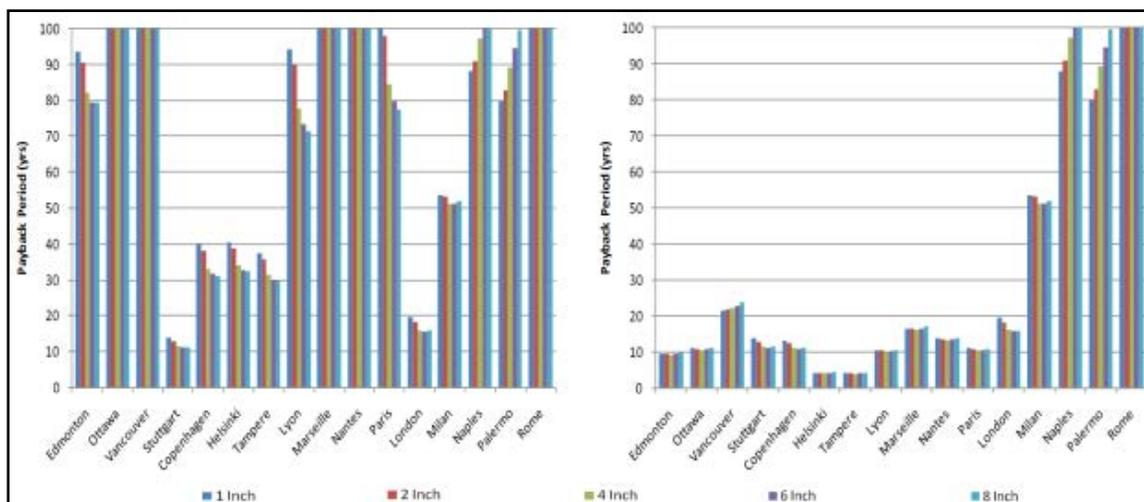
**Figure 6.177. SPB period for baselines 1 (left) and 2 (right) with drainage system installation – international sites.**
