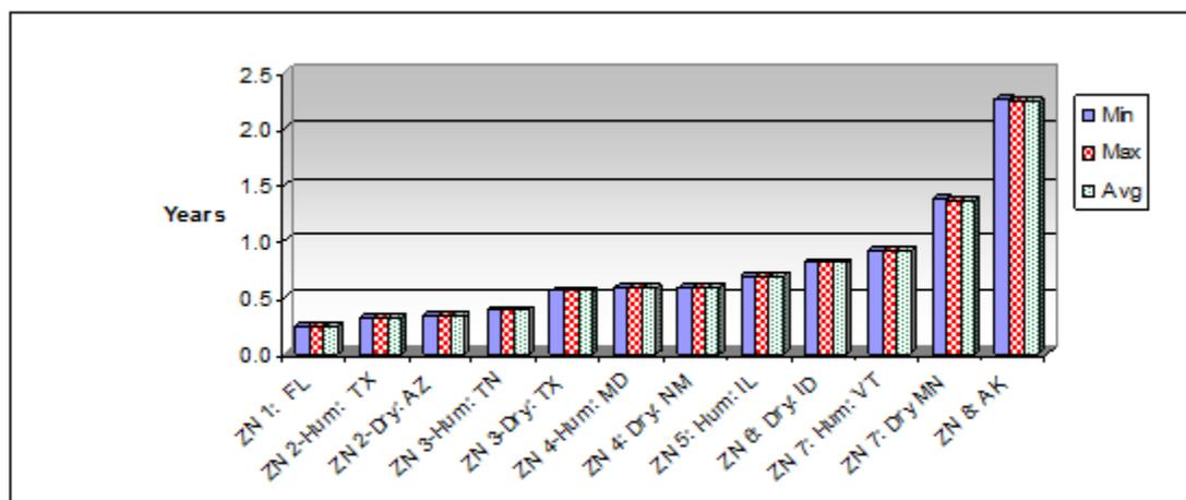
Figure 6.7. Estimated payback based on \$1.00/sq ft cool roof cost premium for high, medium and low energy rates.
