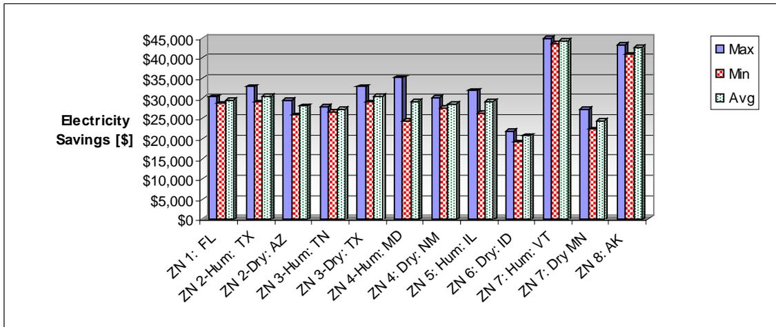
Figure 6.88. Estimated electric savings for a 10% reduction in electric equipment use.
