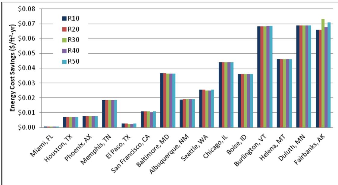
Figure 4.207. Annual energy cost savings for increased roof insulation.
