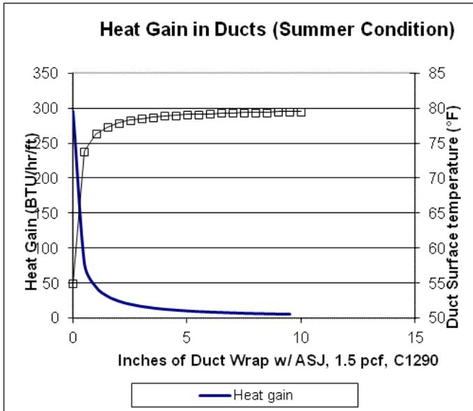
Figure 6.115. Heat gain in ducts and duct surface temperature in summer conditions.
