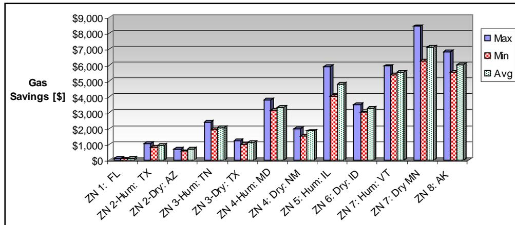
Figure 6.25. Estimated annual gas savings for system achieving 25% reduction of ventilation flow rate.
