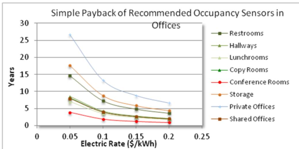
Figure 6.146. Simple payback of recommended occupancy sensors in offices.
