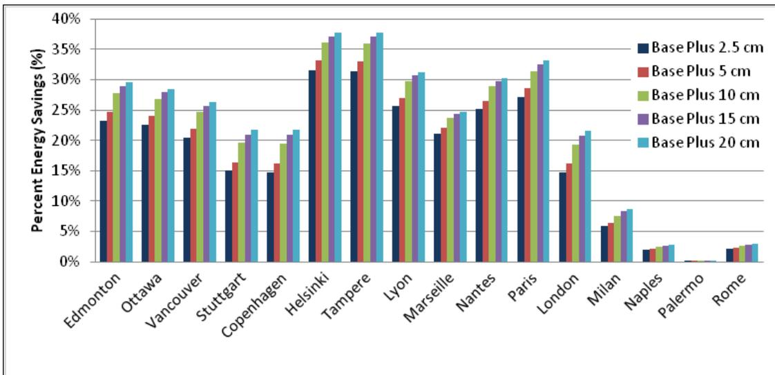
Figure 4.11. Percent energy savings for wall insulation and reduced infiltration over the no-insulation baseline- international locations.
