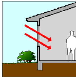
Figure 6.134. Solar heat gain.
