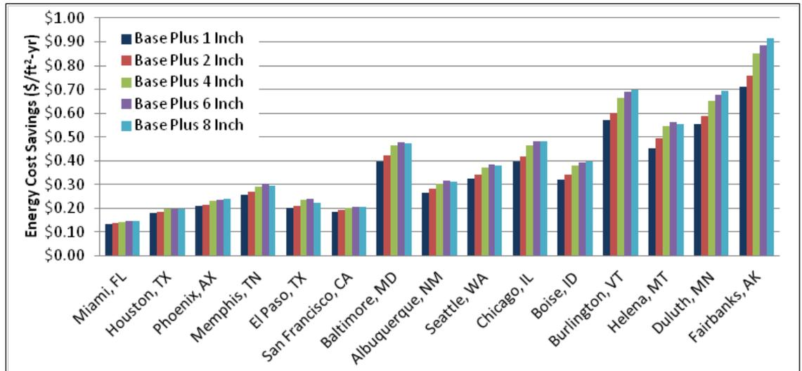
Figure 4.86. Energy cost savings for wall insulation and reduced infiltration over the no-insulation baseline.
