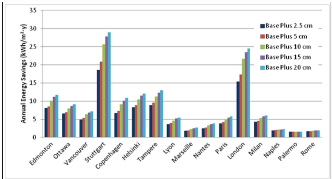
Figure 4.198. Energy savings for wall insulation and reduced infiltration over the standard baseline – international locations.
