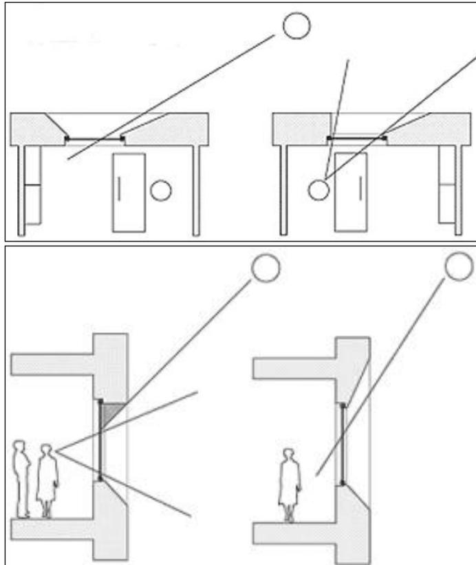
**Figure 7.11. Schemes showing the effectiveness of the tilted sides of the windows.**
