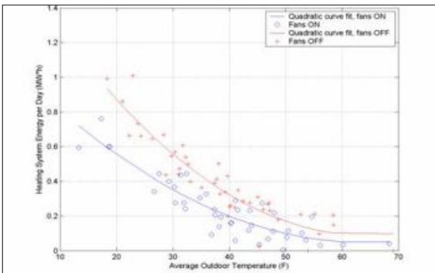
Figure 7.46. Heating system energy usage per average outdoor temperature for Bethesda.
