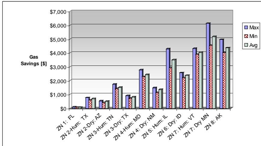
Figure 6.103. Estimated gas savings for 10% airflow reduction case.
