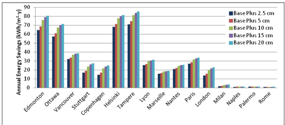
Figure 4.202. Energy savings for wall insulation and reduced infiltration over the no-insulation baseline – international locations.
