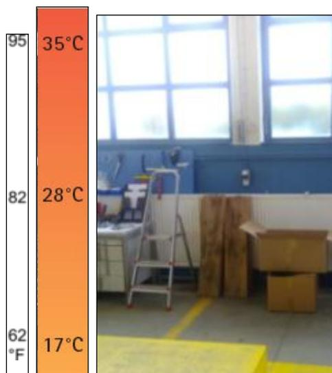
Figure 7.126. Radiators were used for heating prior to the retrofit; as a result, temperature varied greatly between the floor and ceiling.
