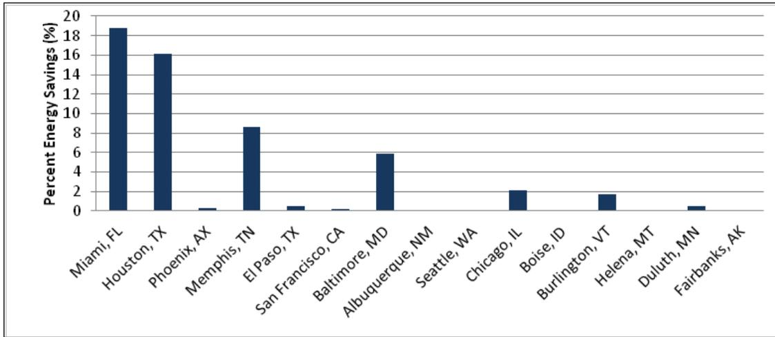
Figure 4.78. Percent energy savings for reheat using condenser waste heat.
