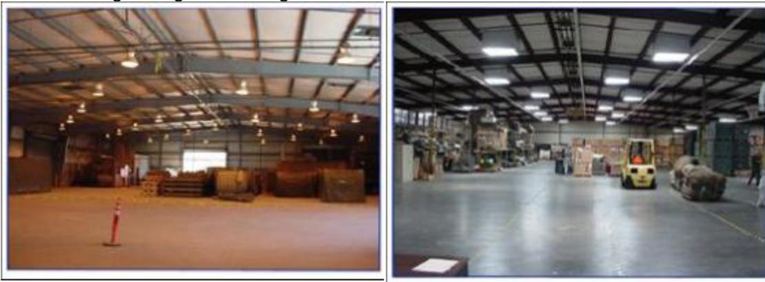
**Figure 6.8. Warehouse application without (left) and with (right) skylights.**
