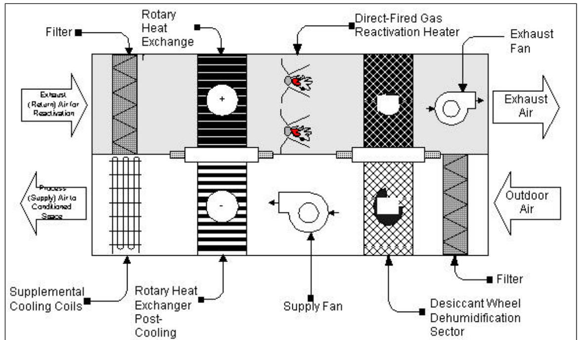
**Figure 7.161. Schematic of the two-wheel desiccant system.**
