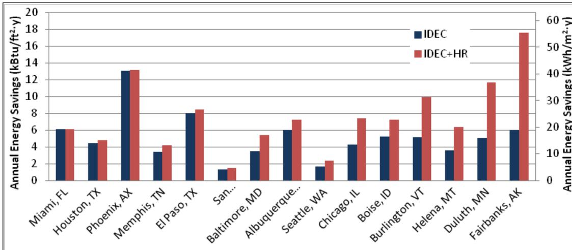
Figure 4.264. Annual energy savings for indirect evaporative cooling and indirect evaporative cooling with heat recovery.
