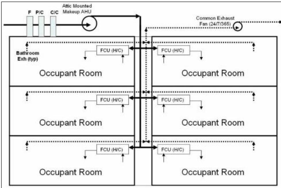
**Figure 7.69. Original system configuration (elevation view).**
