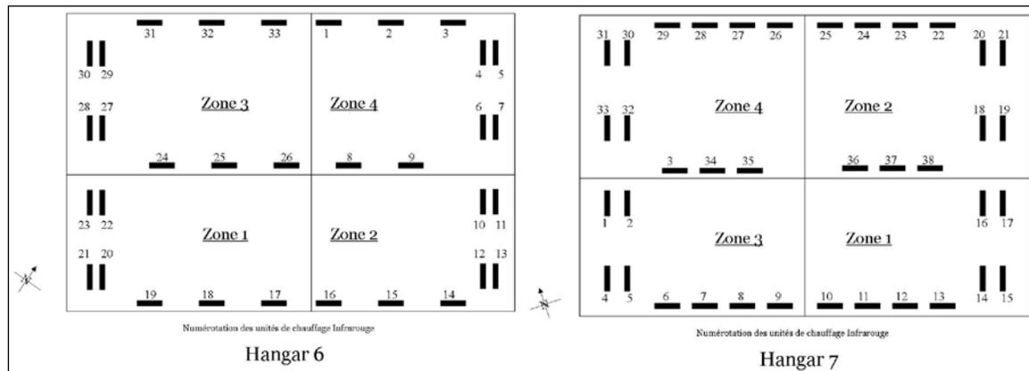
**Figure 7.18. Thirty-three infrared units installed in Hangar 6; 38 installed in Hangar 7.**
