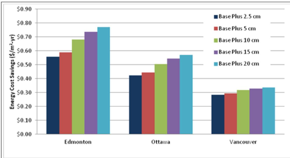
Figure 4.89. Energy cost savings for wall insulation and reduced infiltration over Standard 90.1-1989 baseline – Canadian locations.
