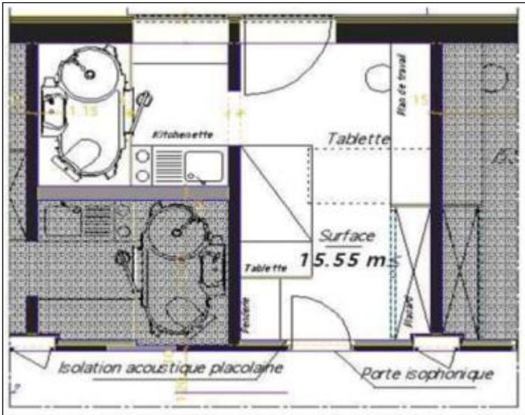
Figure 7.28. Floor plan of one housing unit.
