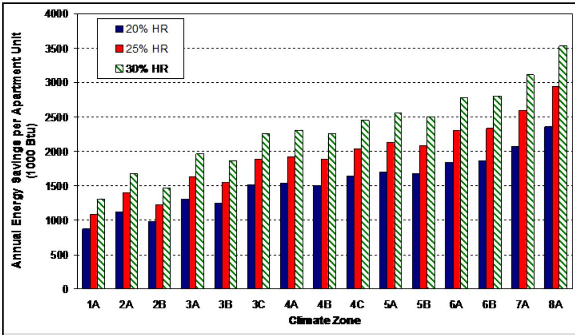
Figure 6.144. Annual energy savings per apartment unit with different heat recovery efficiency.
