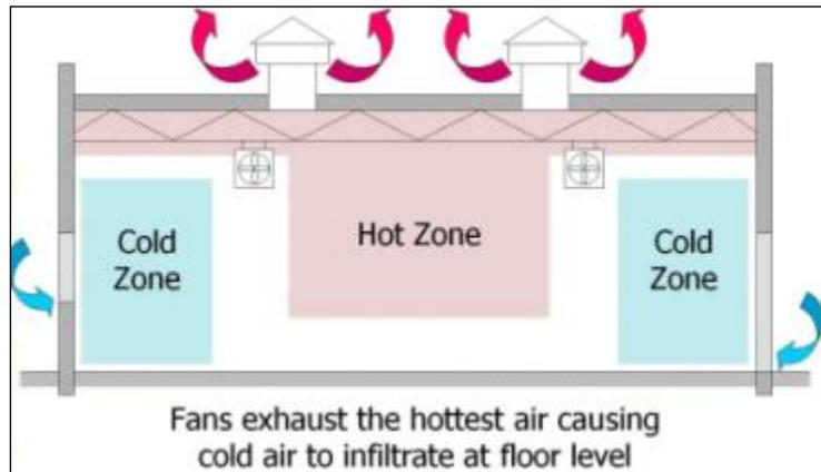
**Figure 7.137. Destratification improves comfort while reducing heat losses.**
