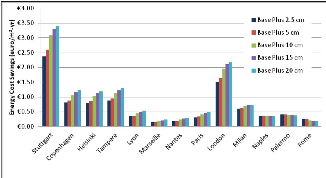
Figure 4.200. Energy cost savings for wall insulation and reduced infiltration over the standard baseline – European locations.
