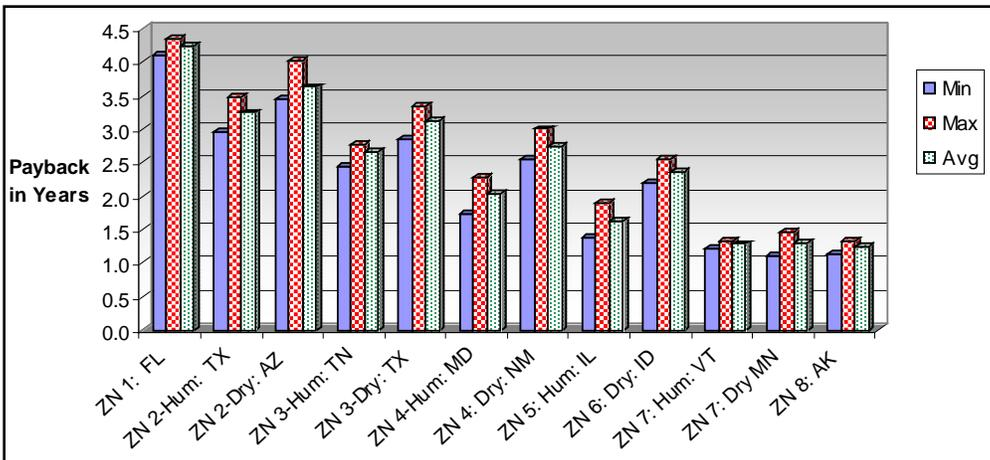
Figure 6.23. Estimated payback for system achieving 25% reduction of ventilation flow rate.
