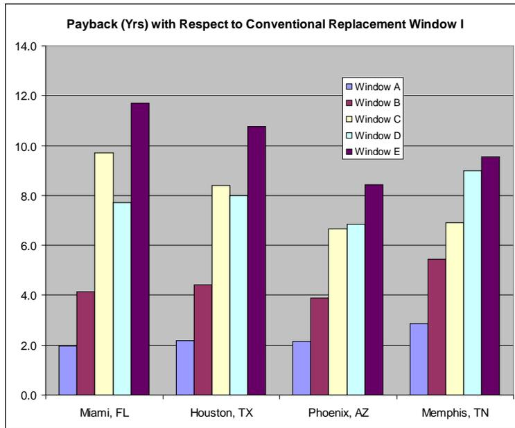
**Figure 6.140. Modeled payback results of upgrading to premium quality replacement windows from current baseline quality replacement windows (Zones 1A, 2A, 2B, and 3A) for a major renovation or repair project.**
