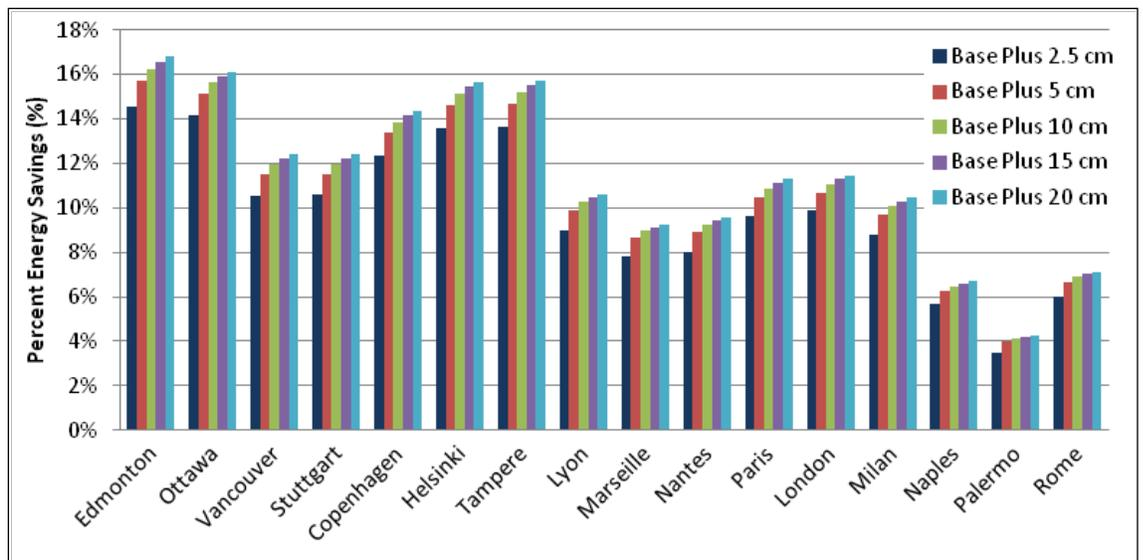
Figure 4.24. Percent energy savings for increased attic insulation and reduced building infiltration over the Standard 90.1-1989 baseline – International locations.
