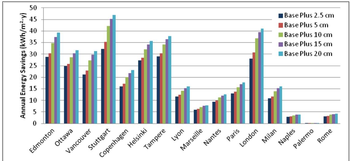
Figure 4.8. Energy savings for wall insulation and reduced infiltration over the Standard 90.1-1989 baseline - international locations.
