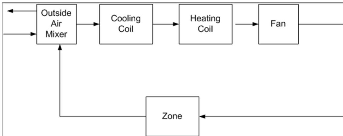
Figure 3.7. Baseline HVAC system diagram for US and Canadian locations.
