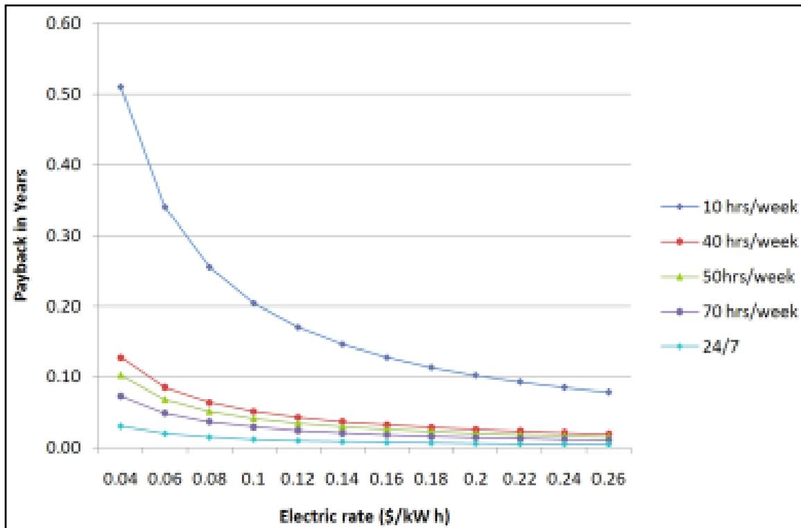
Figure 6.179. Simple payback of incandescent retrofit with CFLs.
