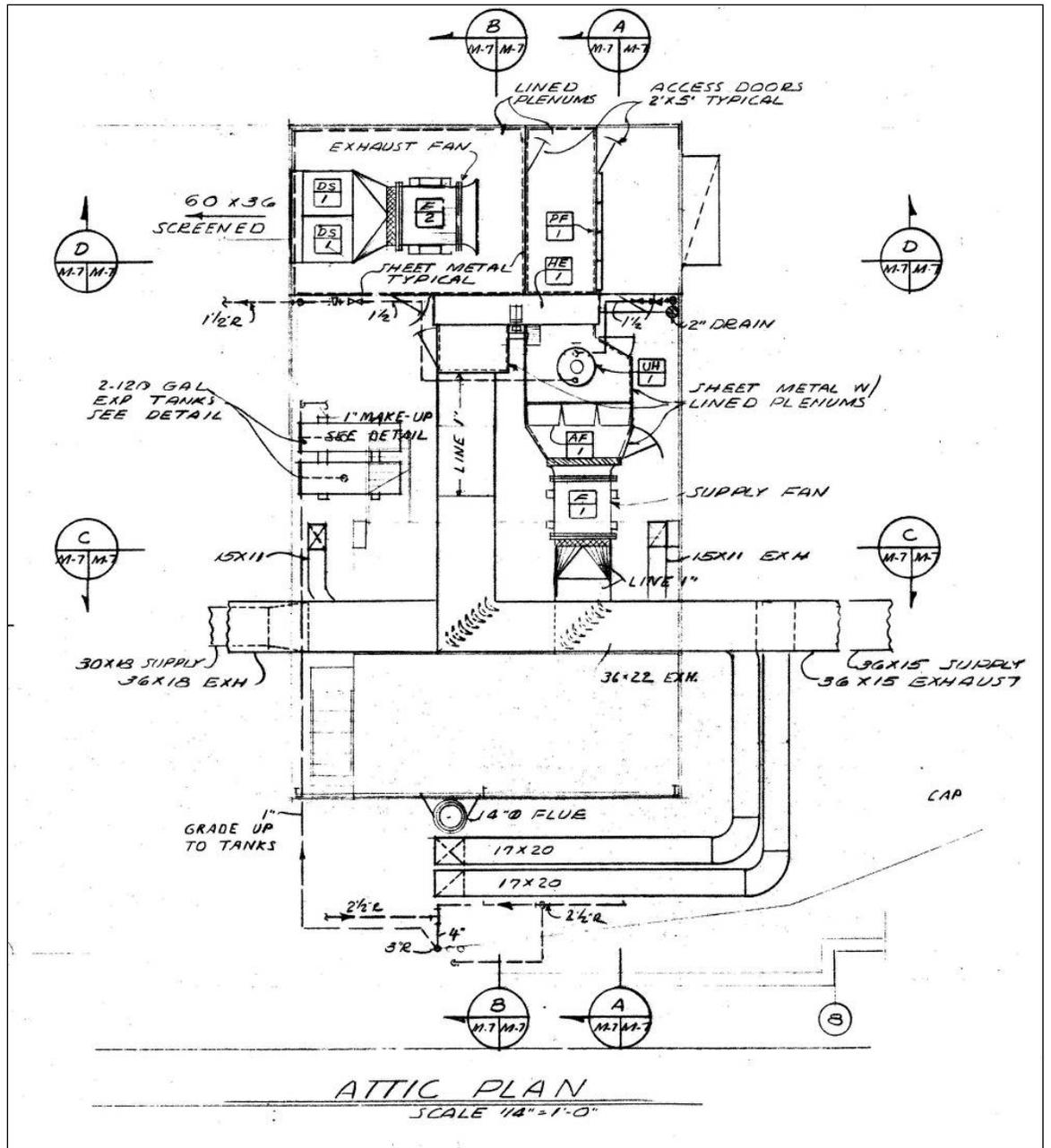
Figure 7.93. Layout of AHU in attic of Bldg. 865.
