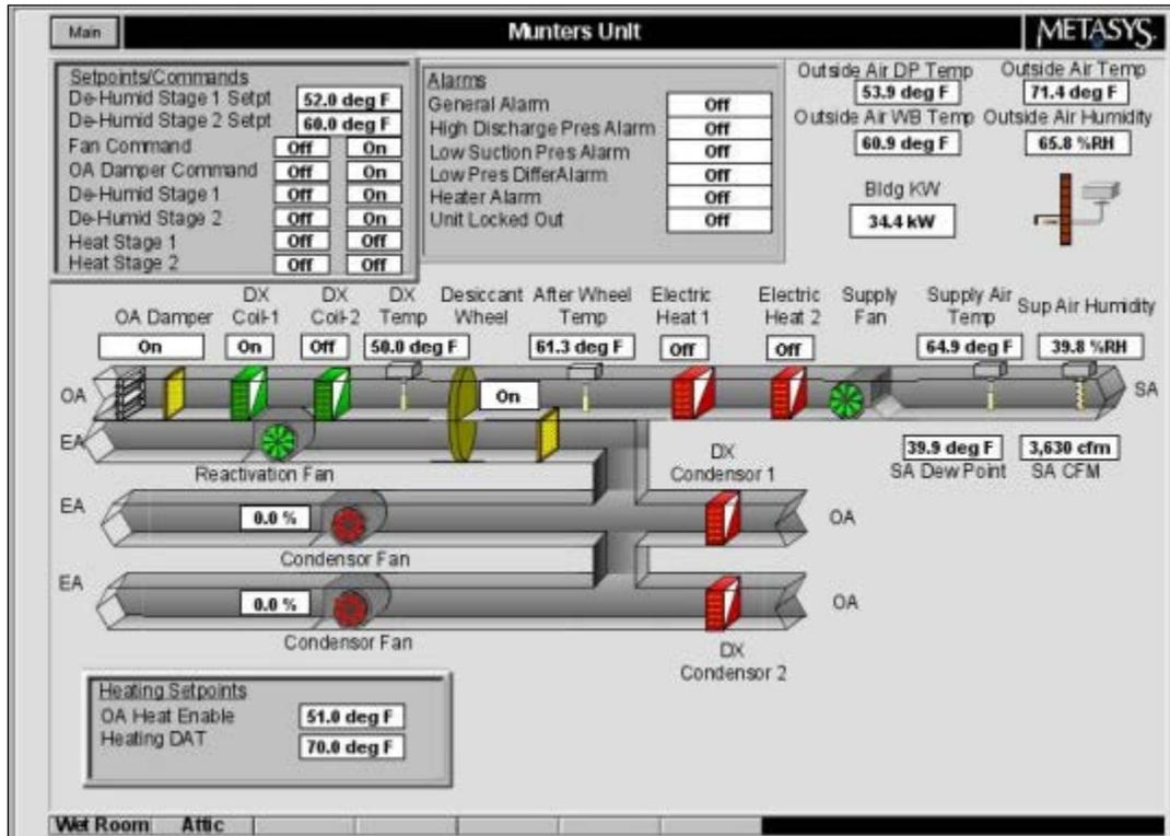
Figure 7.70. Screen capture of Bldg. 637 DX/desiccant DOAS unit schematic.
