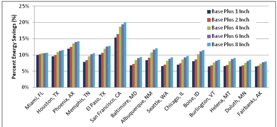
Figure 4.4. Percent energy savings for wall insulation and reduced infiltration over the no-insulation baseline.
