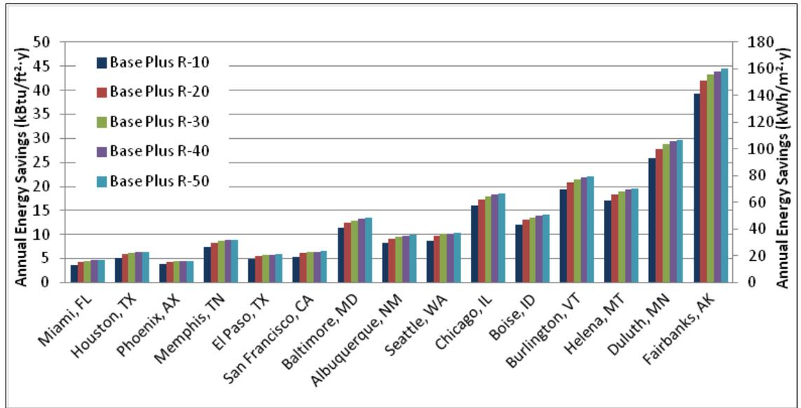
Figure 4.23. Energy savings for increased attic insulation and reduced building infiltration over the Standard 90.1-1989 baseline.
