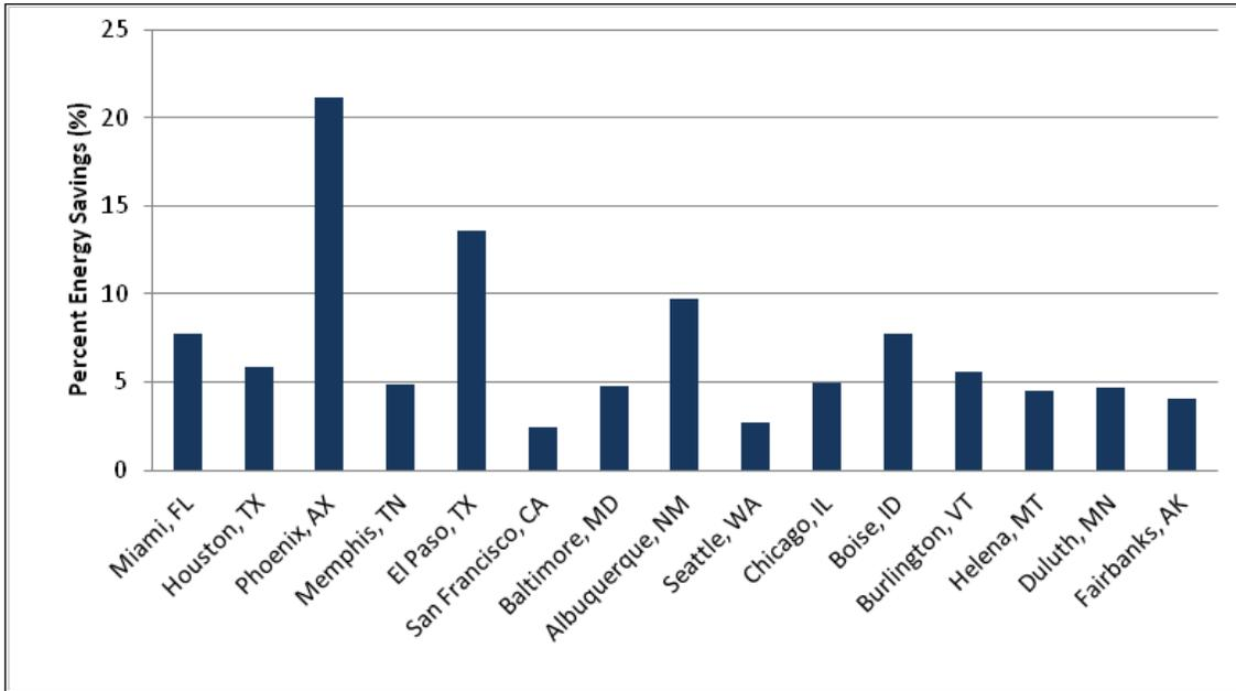
Figure 4.64. Percent energy savings for hybrid evaporative cooling.
