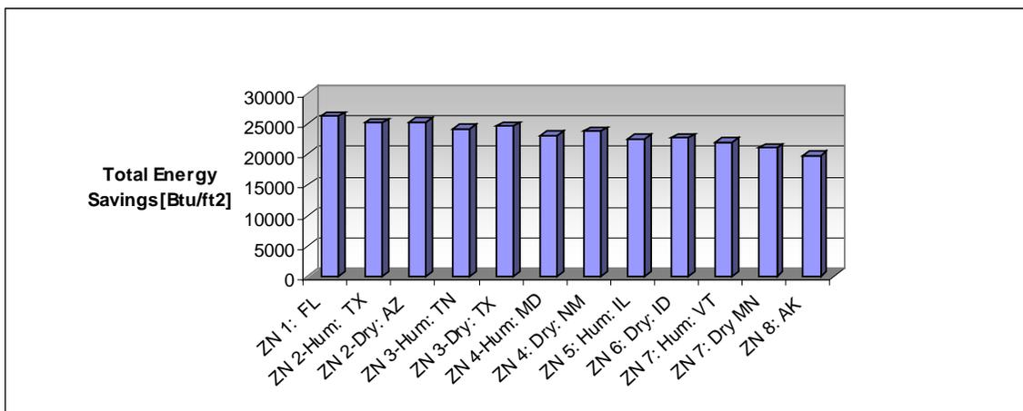
Figure 6.90. Estimated net energy savings for a 10% reduction in electric equipment use.
