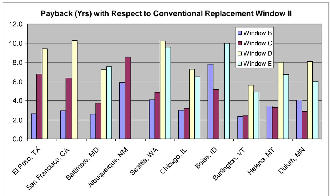
**Figure 6.141. Modeled payback results of upgrading to premium quality replacement windows from current baseline quality replacement windows (Zones 3B, 4A, 4B, 4C, 5A, 5B, 6A, 6B and 7A) for a major renovation or repair project.**
