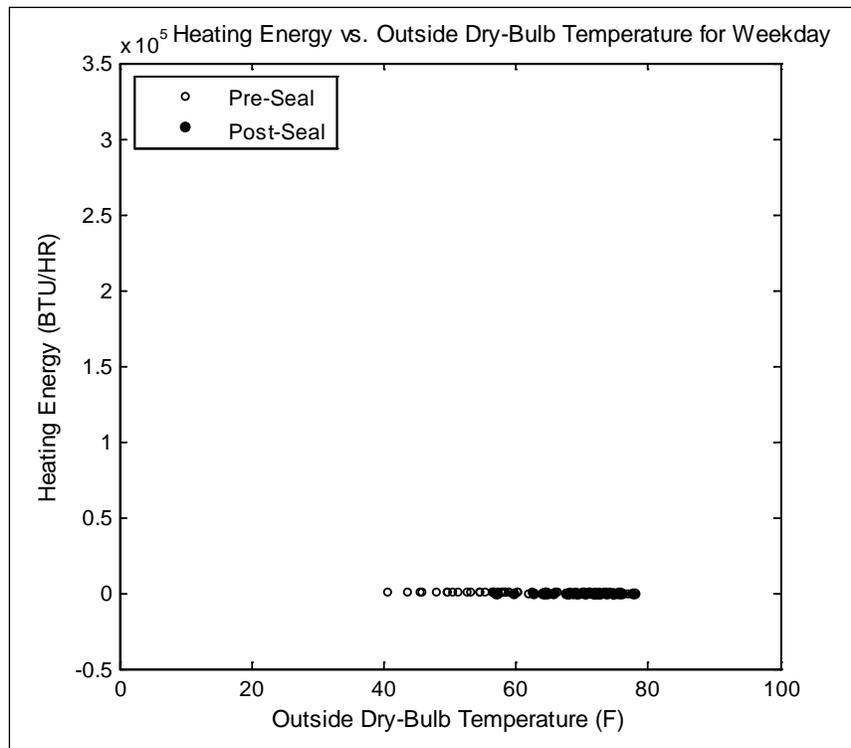
**Figure 7.4. Bldg. 1268 pre- and post-sealant heating energy as a function of outdoor air temperature during the heating season.**
