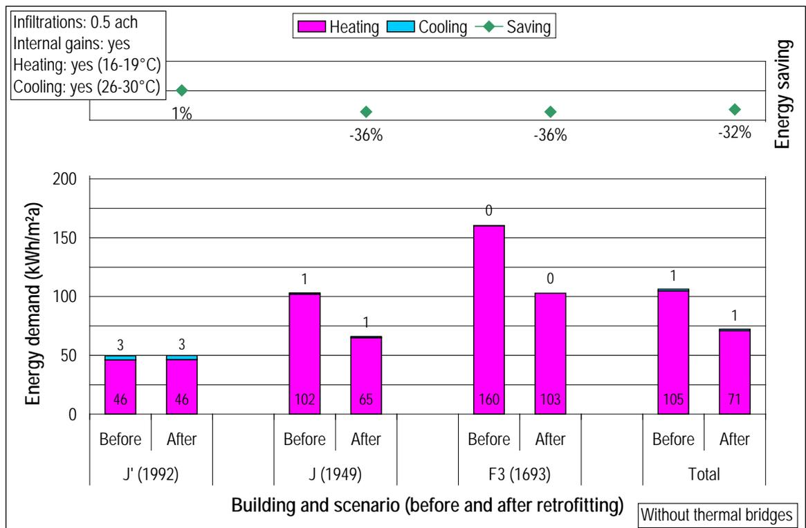
Figure 7.97. Calculated heating and cooling demand before and after retrofitting.
