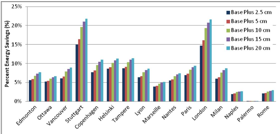
Figure 4.7. Percent energy savings for wall insulation and reduced infiltration over the Standard 90.1-1989 baseline - international locations.
