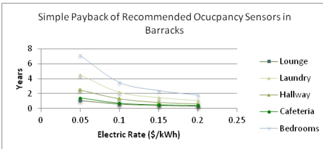
Figure 6.147. Simple payback of recommended occupancy sensors in barracks.
