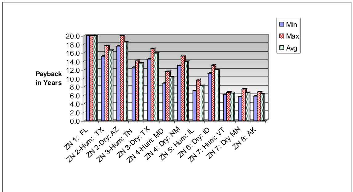
Figure 6.99. Estimated payback for 5% reduction in air flow rate.
