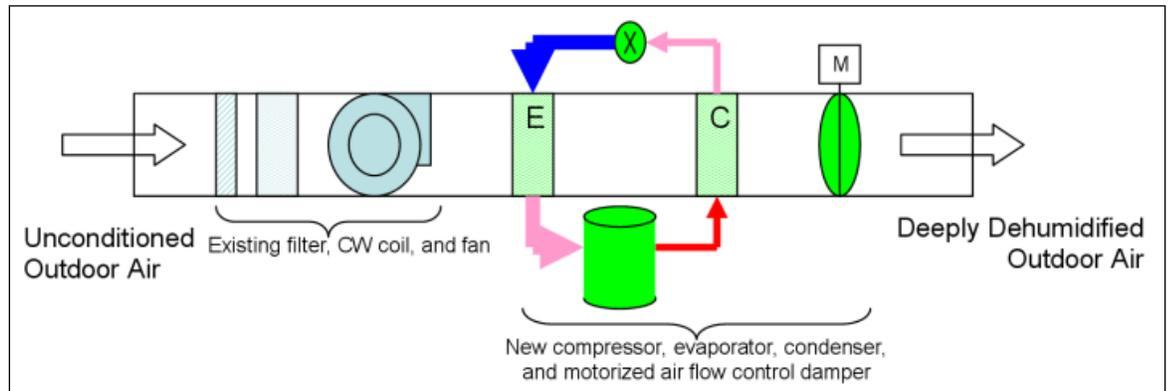
Figure 7.62. DOAS system schematic.
