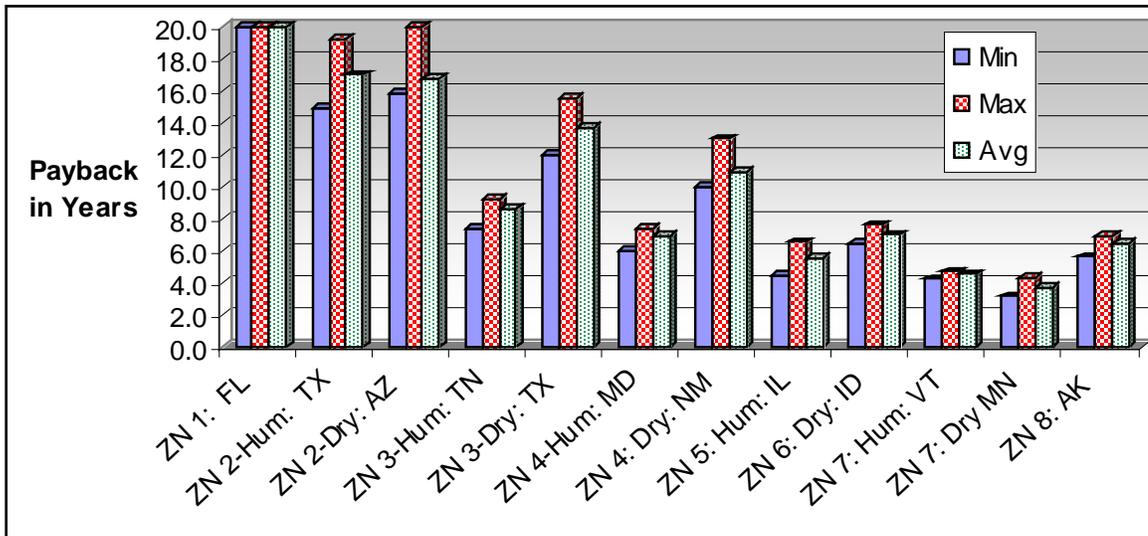
Figure 6.80. Transpired solar wall estimated payback shown for high, medium, and low energy rates.
