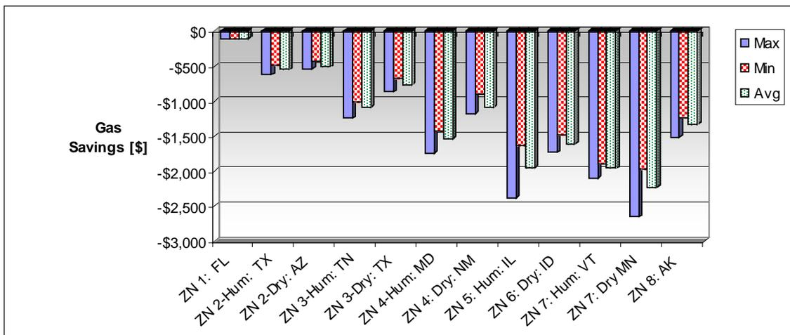
Figure 6.89. Estimated increase in heating cost for a 10% reduction in electric equipment use.
