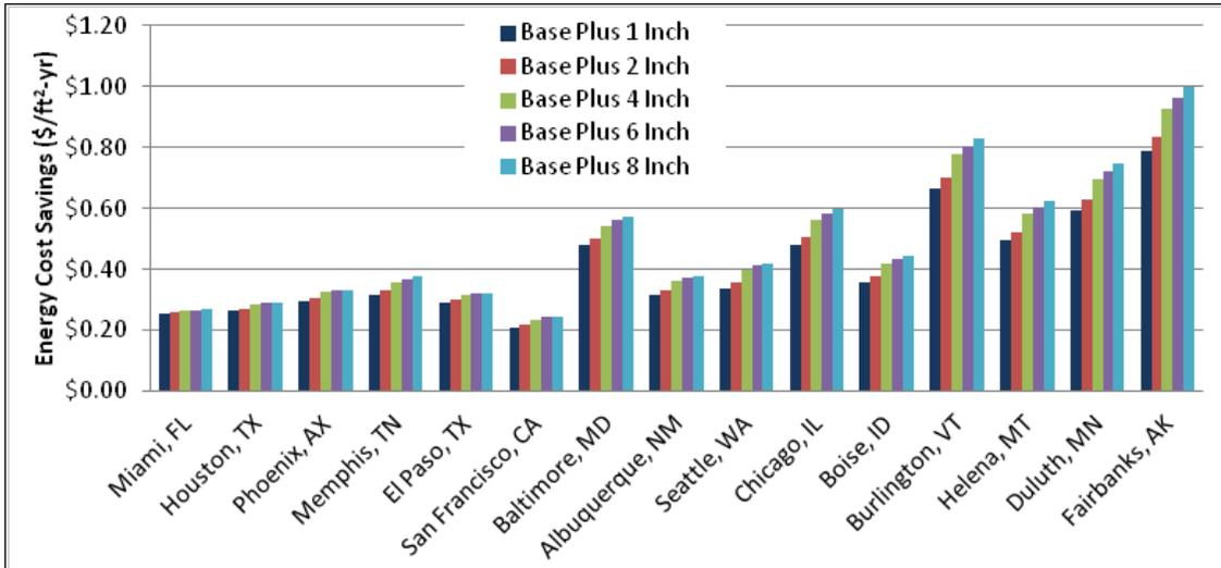
Figure 4.6. Energy cost savings for wall insulation and reduced infiltration over the no-insulation baseline.
