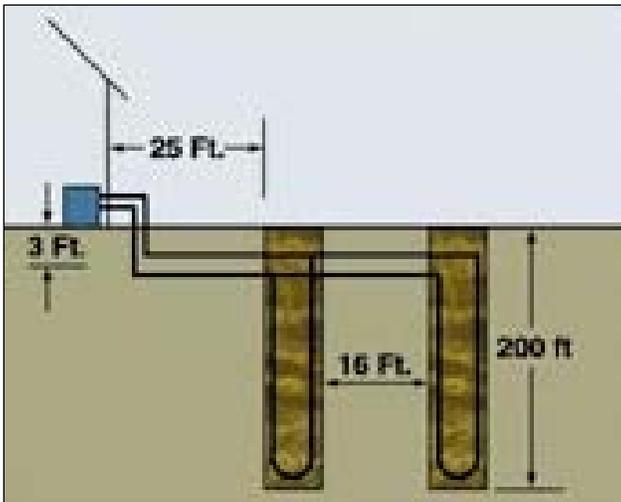
**Figure 7.101.** Each heat pump is linked to two U-shaped ground heat exchangers that are in 4-1/8-in. vertical bores.
