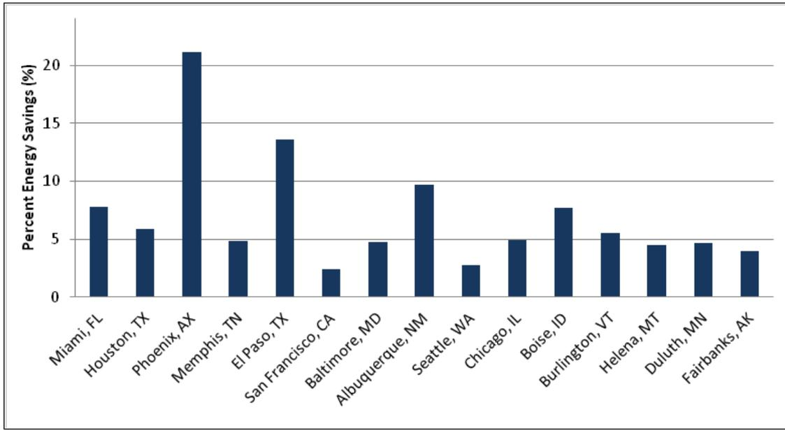
Figure 4.160. Percent energy savings for hybrid evaporative cooling.
