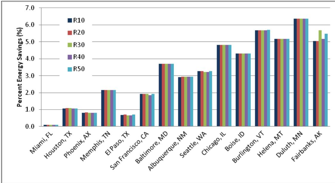
Figure 4.95. Percent energy savings for increased roof insulation.
