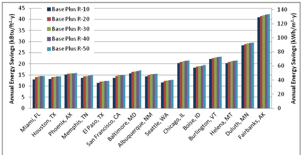
Figure 4.16. Energy savings for increased roof insulation and reduced infiltration over the Standard 90.1-1989 baseline.
