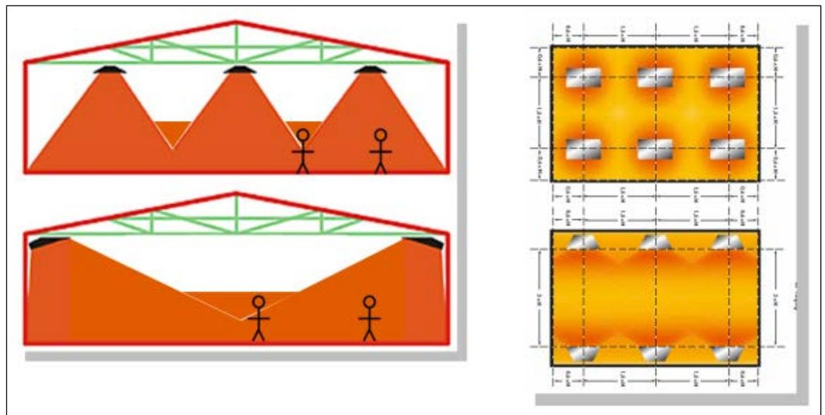
**Figure 7.20. Interior versus perimeter placement.**
