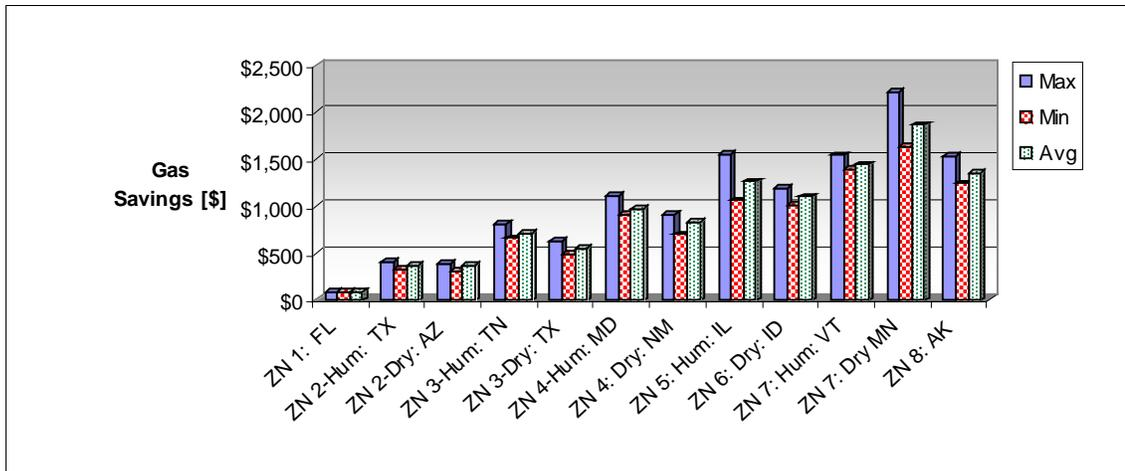
Figure 6.57. Estimated gas savings for high speed roller doors.
