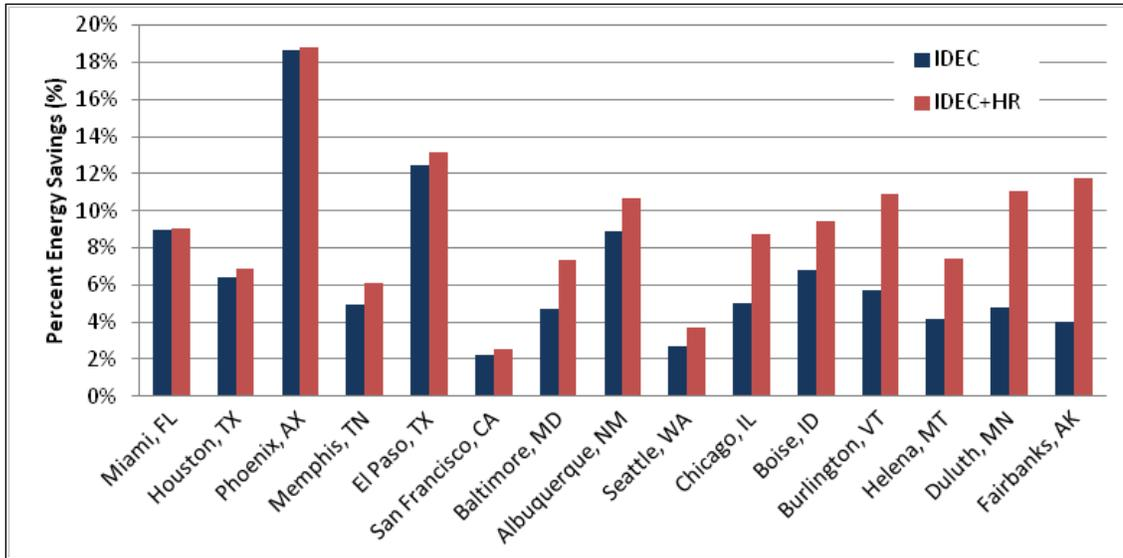
Figure 4.263. Percent energy savings for indirect evaporative cooling and indirect evaporative cooling with heat recovery.
