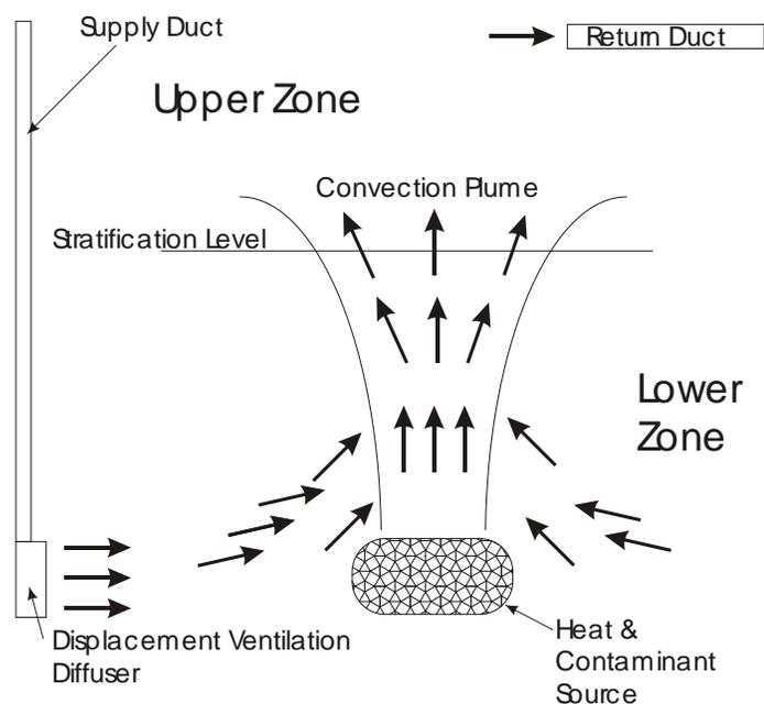
**Figure 6.19. Displacement ventilation concept.**
