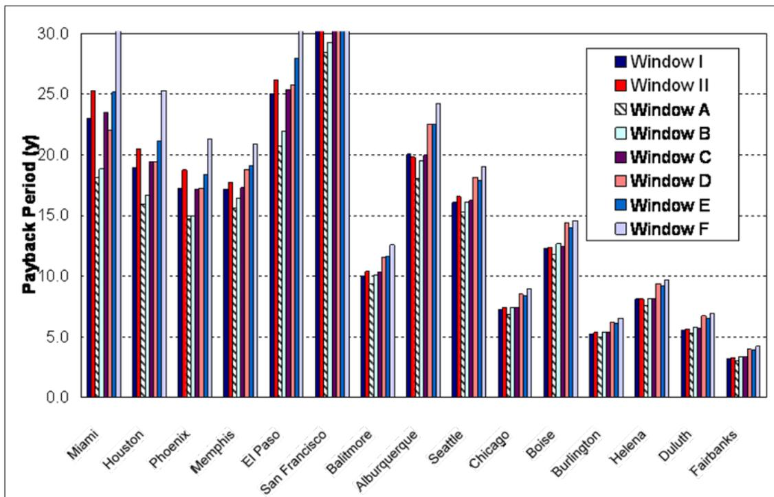
**Figure 6.139. Modeled payback results of an *energy conservation project* using absolute retrofit cost and energy savings compared to a baseline window type.**
