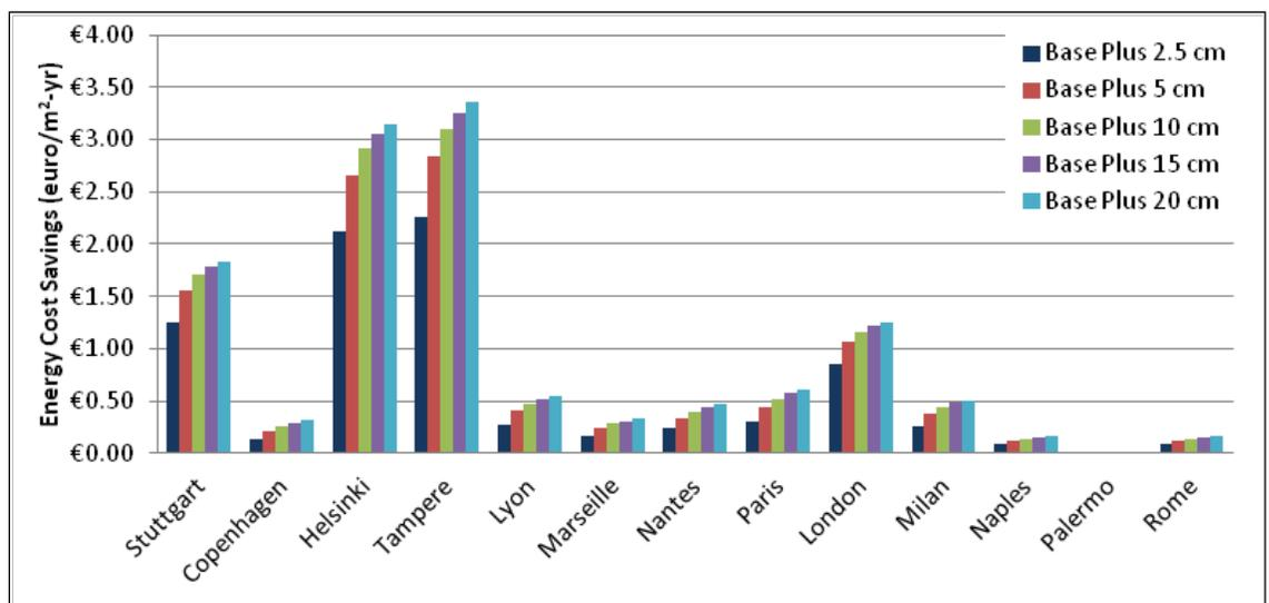
Figure 4.21. Energy cost savings for increased roof insulation and reduced infiltration over the Standard 90.1-1989 baseline – European locations.
