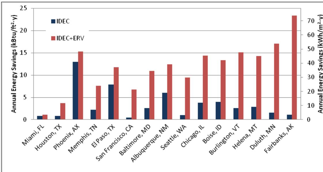
Figure 4.62. Annual energy savings for indirect evaporative cooling and indirect evaporative cooling with energy recovery.
