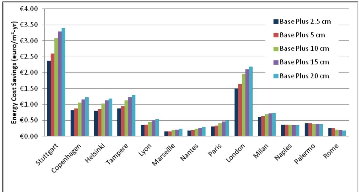
Figure 4.90. Energy cost savings for wall insulation and reduced infiltration over the standard baseline – European locations.
