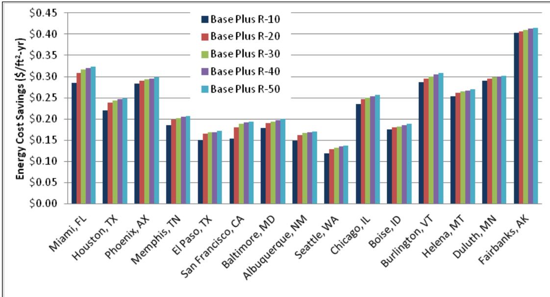
Figure 4.17. Energy cost savings for increased roof insulation and reduced infiltration over the Standard 90.1-1989 baseline.
