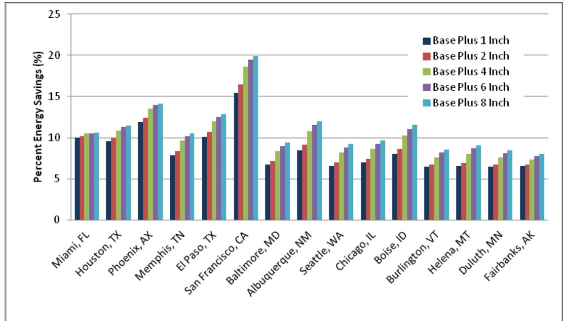
**Figure 4.1. Percent energy savings for wall insulation and reduced infiltration over Standard 90.1-1989 baseline.**
