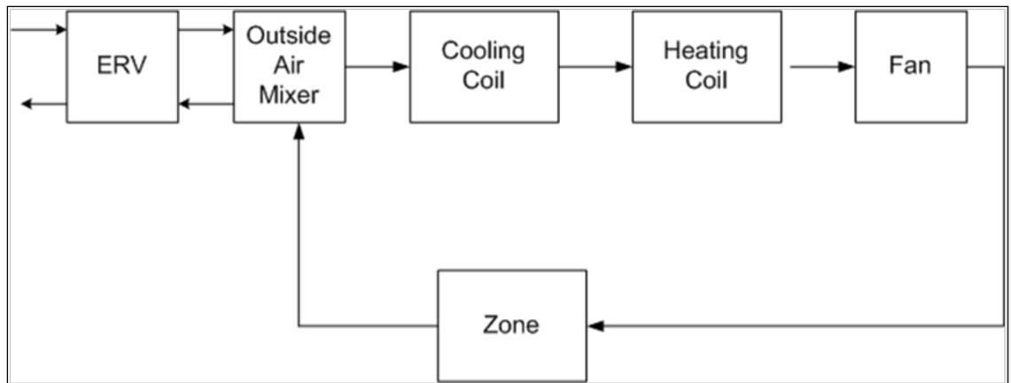
Figure 4.56. Schematic of the energy recovery ventilator model (credit: Kyle Benne).
