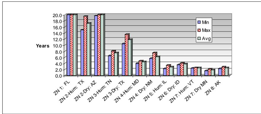
Figure 6.42. Radiant barrier estimated payback for high, low and medium energy rates.
