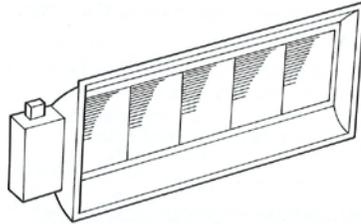
**Figure 6.61. High intensity radiant heater.**
