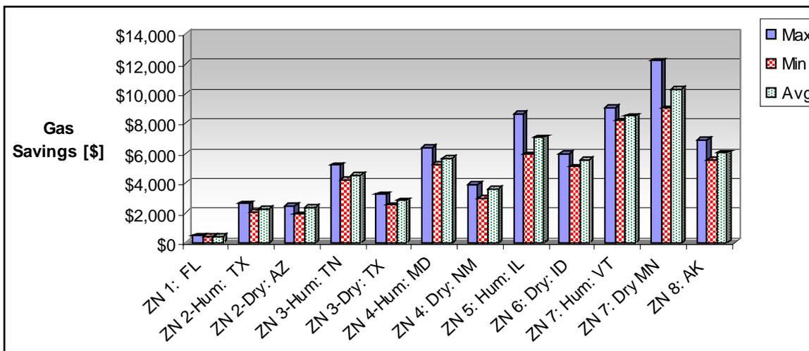
Figure 6.81. Transpired solar wall estimated gas savings shown for high, medium, and low energy rates.
