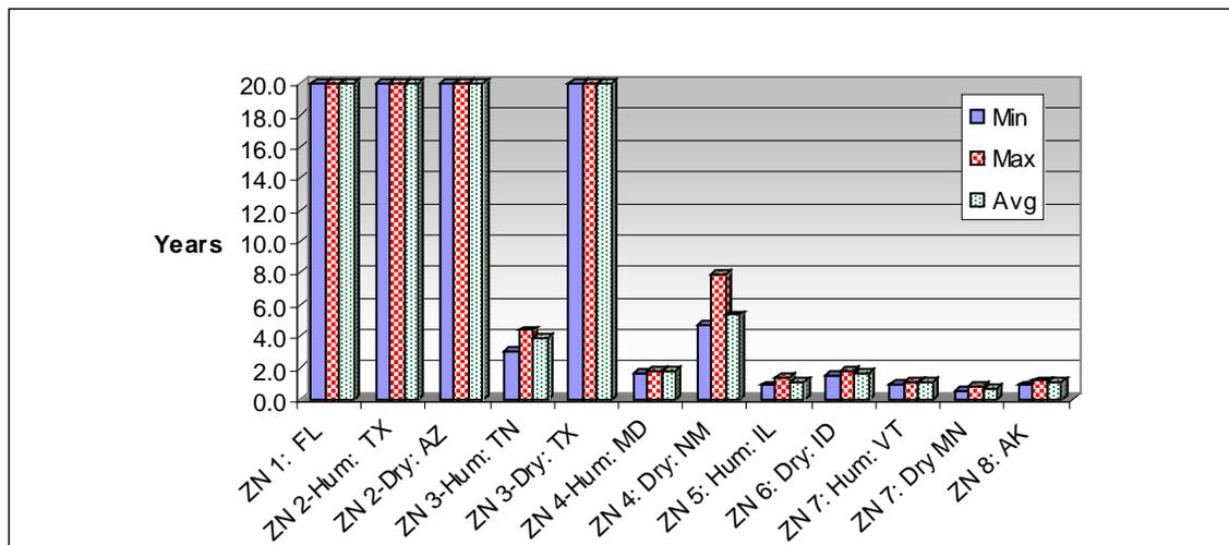
Figure 6.73. Payback potential for the recirculation system with filtration.
