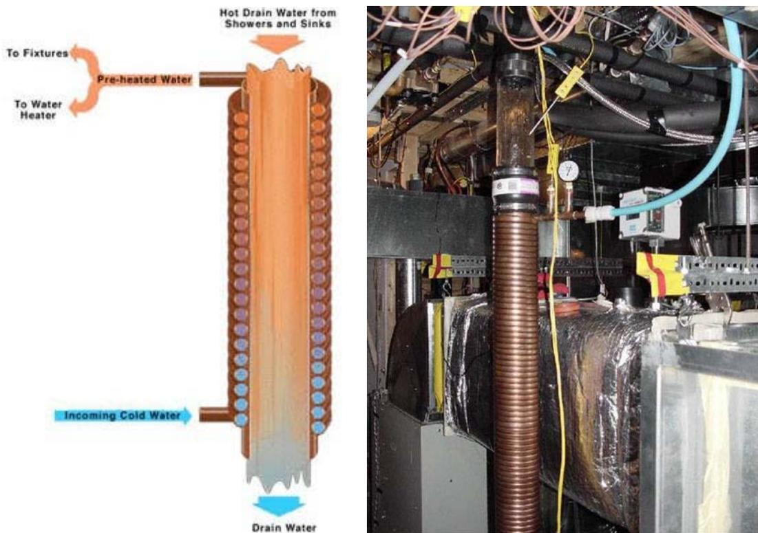
Figure 6.143. GFX system schematics and installation example.
