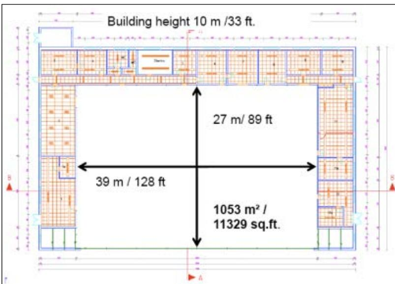
Figure 7.123. Schematic of Hangar 1035.
