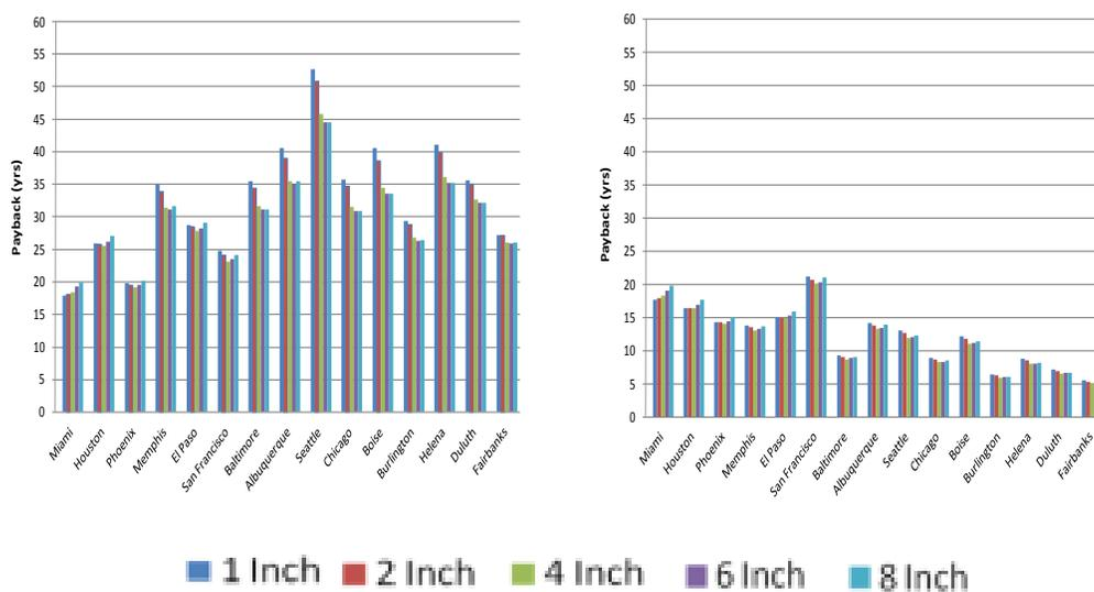
**Figure 6.130. SPB period for Baselines 1 (left) and 2 (right) with drainage system installation.**
