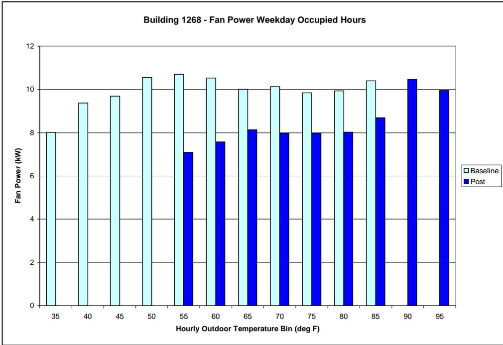
Figure 7.3. Bldg. 1268 pre- and post-sealing total fan power as a function of outdoor air temperature for weekday.
