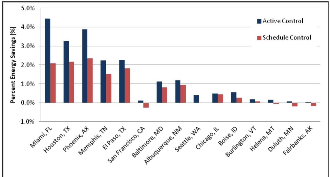
Figure 4.46. Percent energy savings for external roller shades for an east-west orientation.
