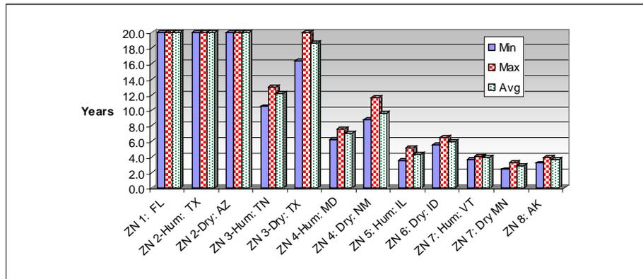
Figure 6.43. Spray foam estimated payback for high, low and medium energy rates.
