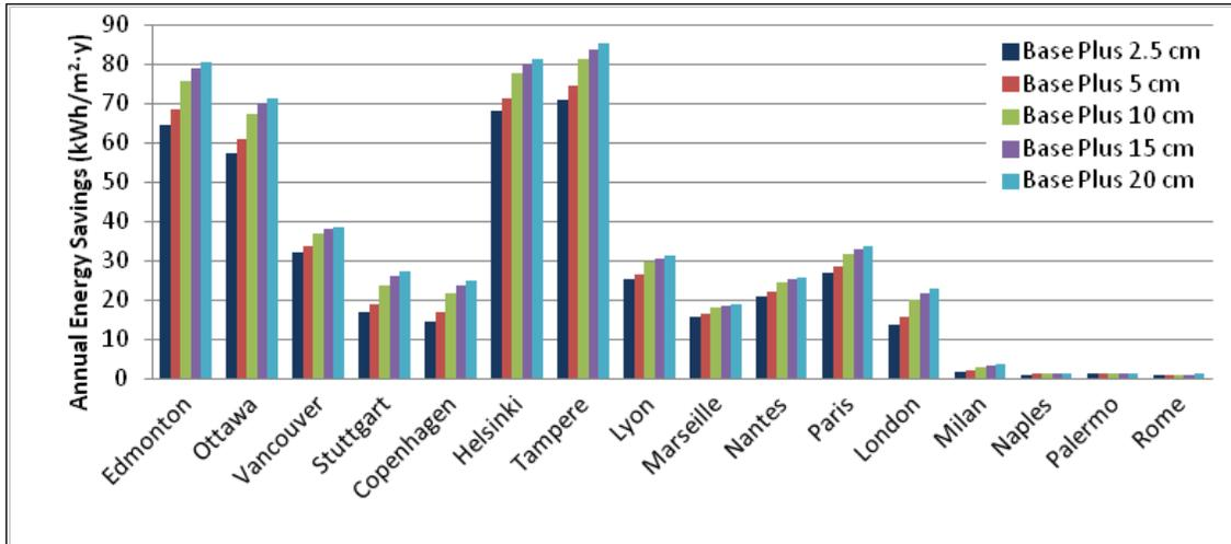
Figure 4.92. Energy savings for wall insulation and reduced infiltration over the no-insulation baseline – international locations.
