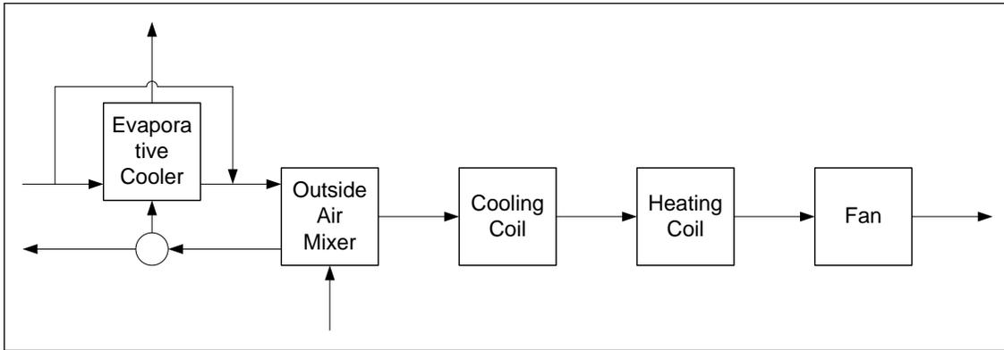
**Figure 4.152. Schematic of the indirect evaporative cooling model (credit: Kyle Benne).**
