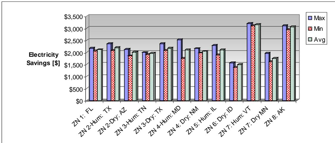
Figure 6.64. Estimated annual electric savings for high temperature radiant system.
