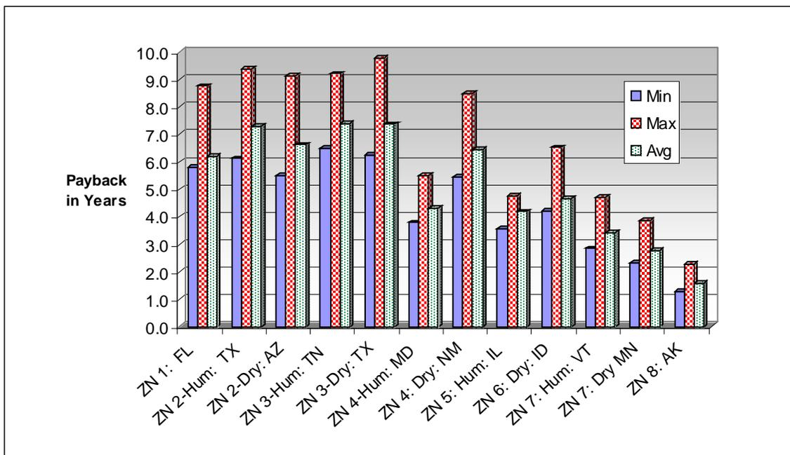
Figure 6.69. Payback for four booths with 15% reduction in system air flow.
