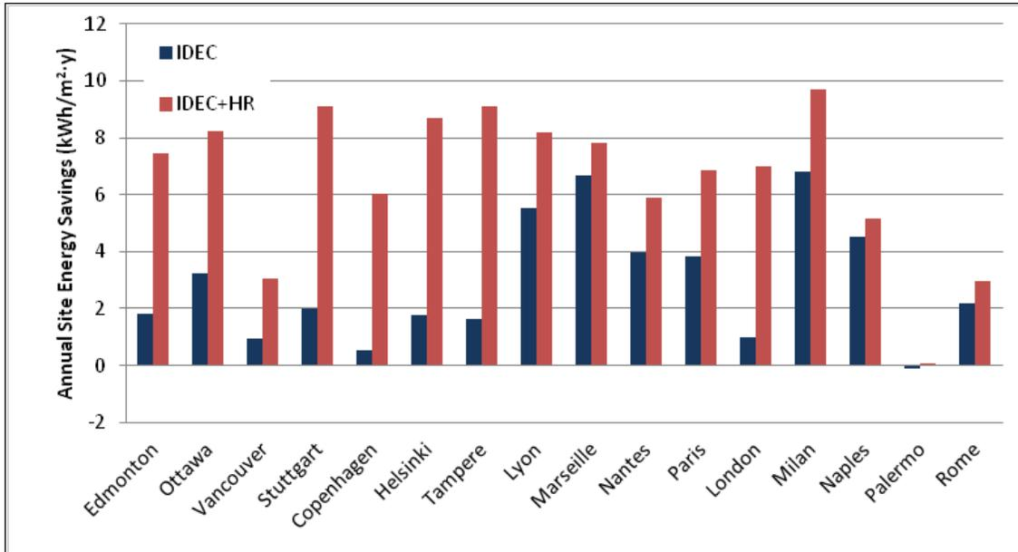
Figure 4.267. Annual energy savings for indirect evaporative cooling and indirect evaporative cooling with heat recovery – International locations.
