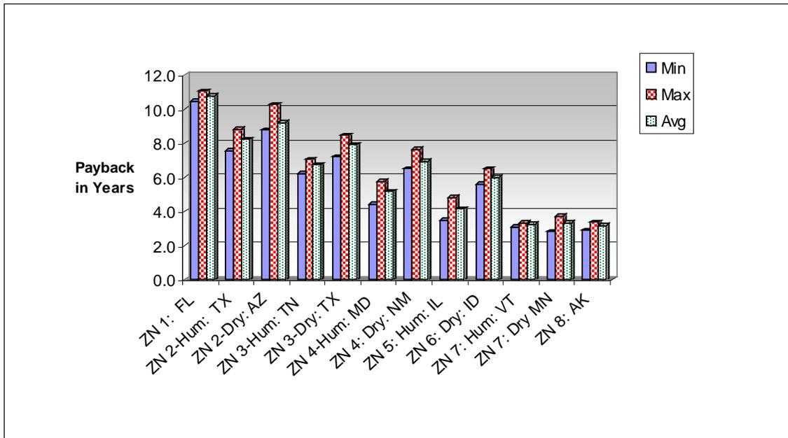
Figure 6.100. Estimated payback for 10% reduction in air flow rate.
