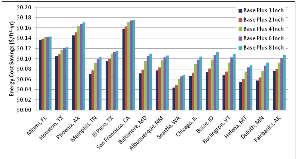
Figure 4.193. Energy cost savings for wall insulation and reduced infiltration over Standard 90.1-1989 baseline.
