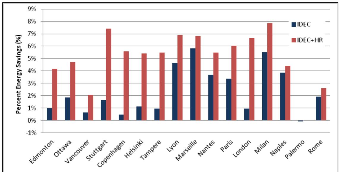
Figure 4.266. Percent energy savings for indirect evaporative cooling and indirect evaporative cooling with heat recovery – International locations.
