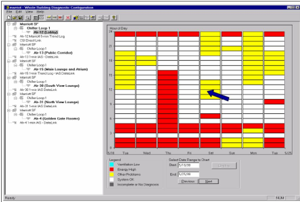
Figure 7.152. Diagnostic results color-coded to show system functioning status.
