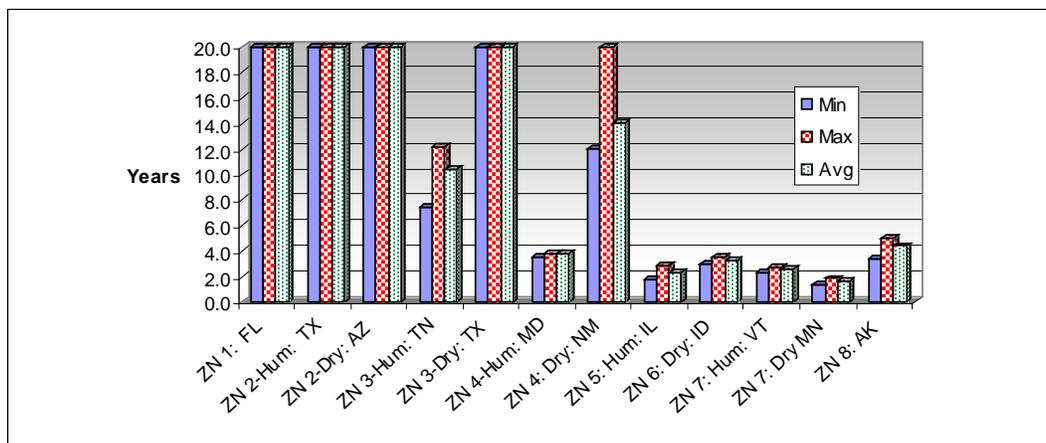
Figure 6.36. Estimated payback for installation of rotary heat exchanger.
