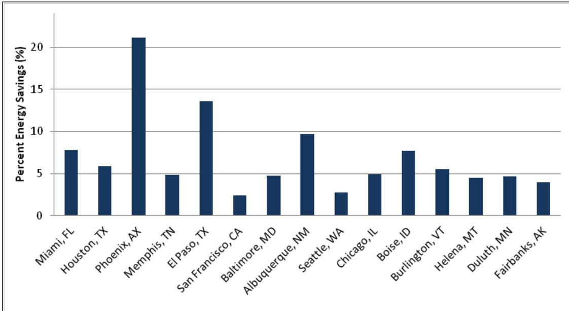
Figure 4.270. Percent energy savings for hybrid evaporative cooling.
