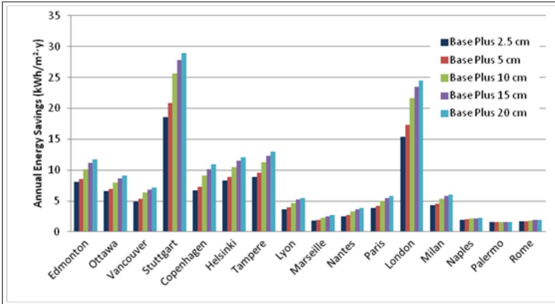
Figure 4.88. Energy savings for wall insulation and reduced infiltration over the standard baseline – international locations.
