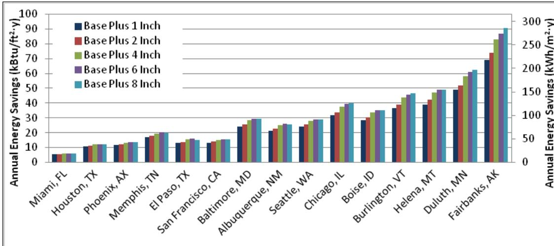
Figure 4.195. Energy savings for wall insulation and reduced infiltration over the no-insulation baseline.
