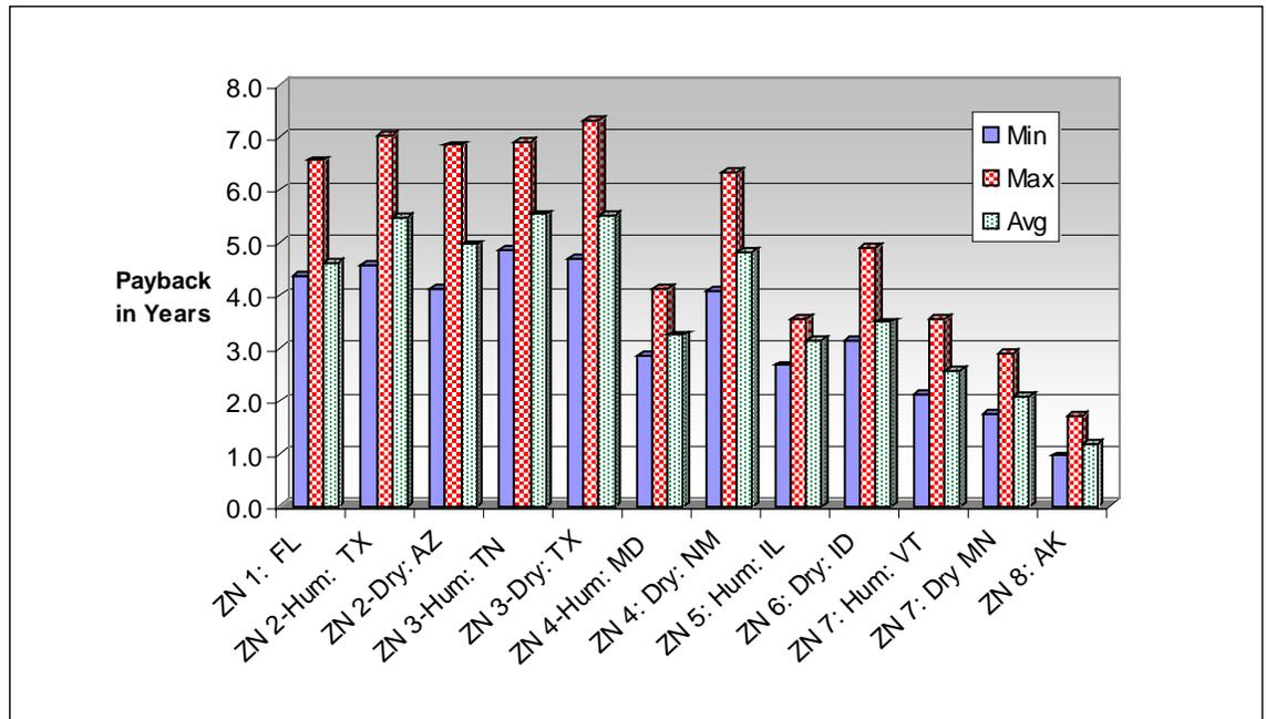
Figure 6.70. Payback for four booths with 20% reduction in system air flow.
