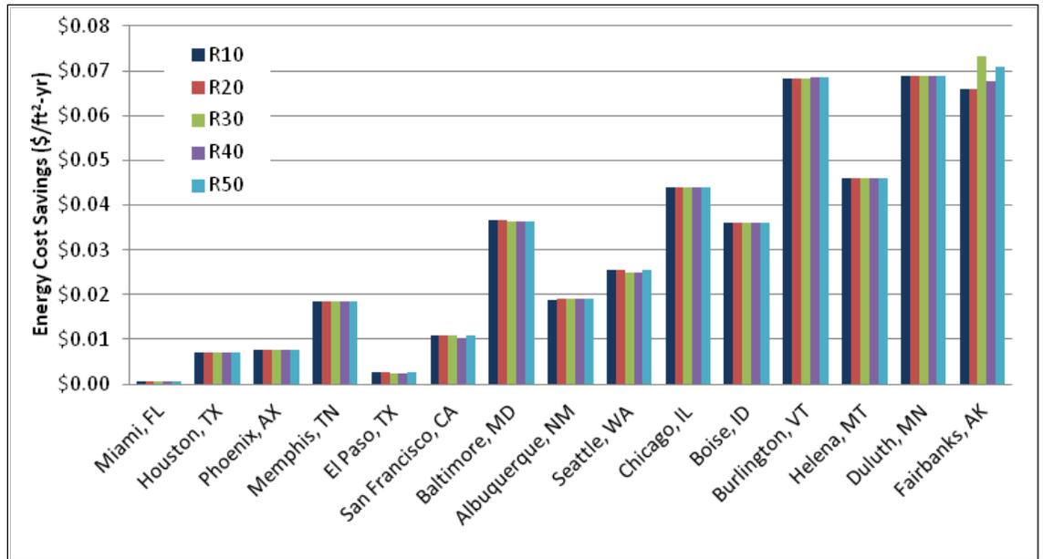
Figure 4.97. Annual energy cost savings for increased roof insulation.
