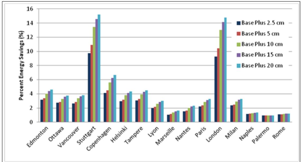
Figure 4.197. Percent energy savings for wall insulation and reduced infiltration over the standard baseline – international locations.
