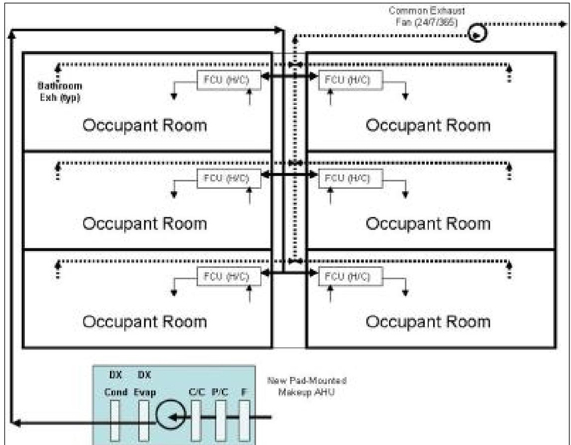
Figure 7.63. New DOAS system configuration (elevation view).
