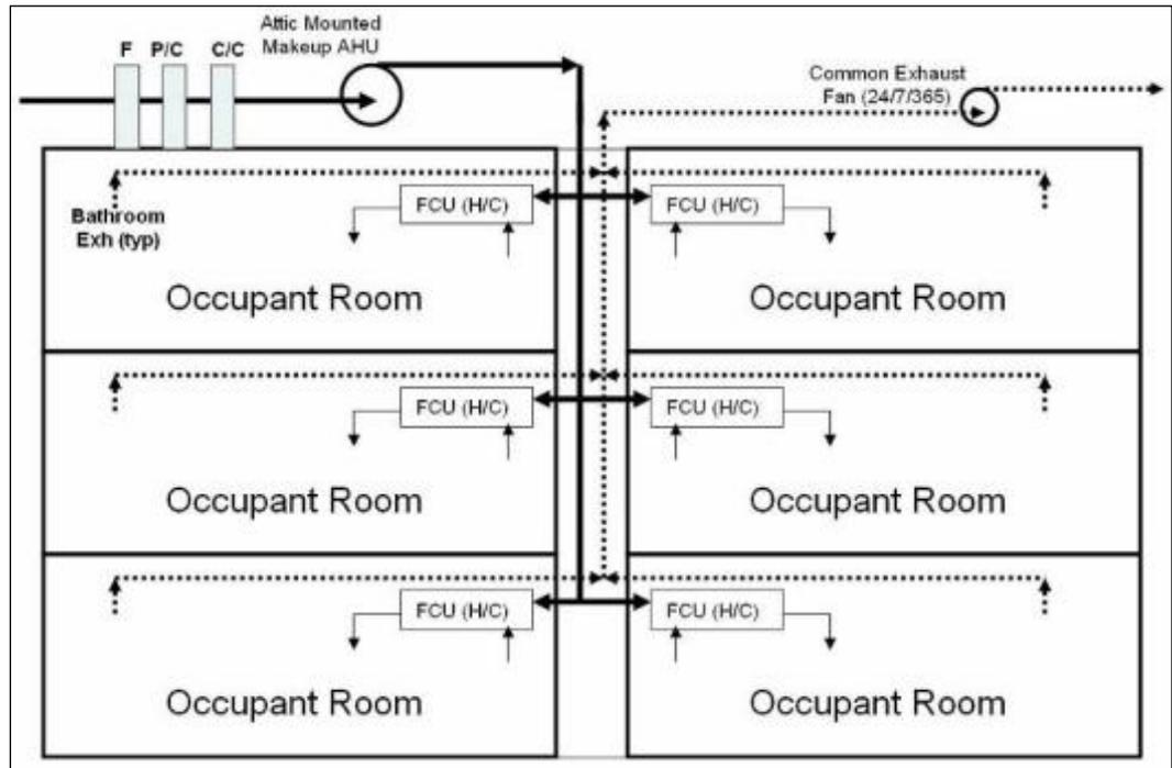
Figure 7.51. Original system configuration (elevation view).
