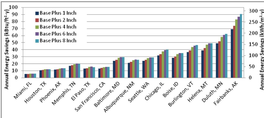
Figure 4.85. Energy savings for wall insulation and reduced infiltration over the no-insulation baseline.
