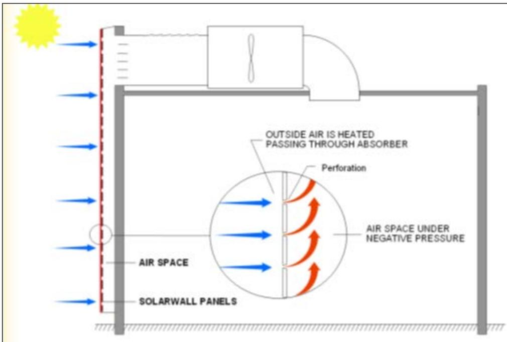
**Figure 7.136. How a SolarWall system preheats ventilation air.**
