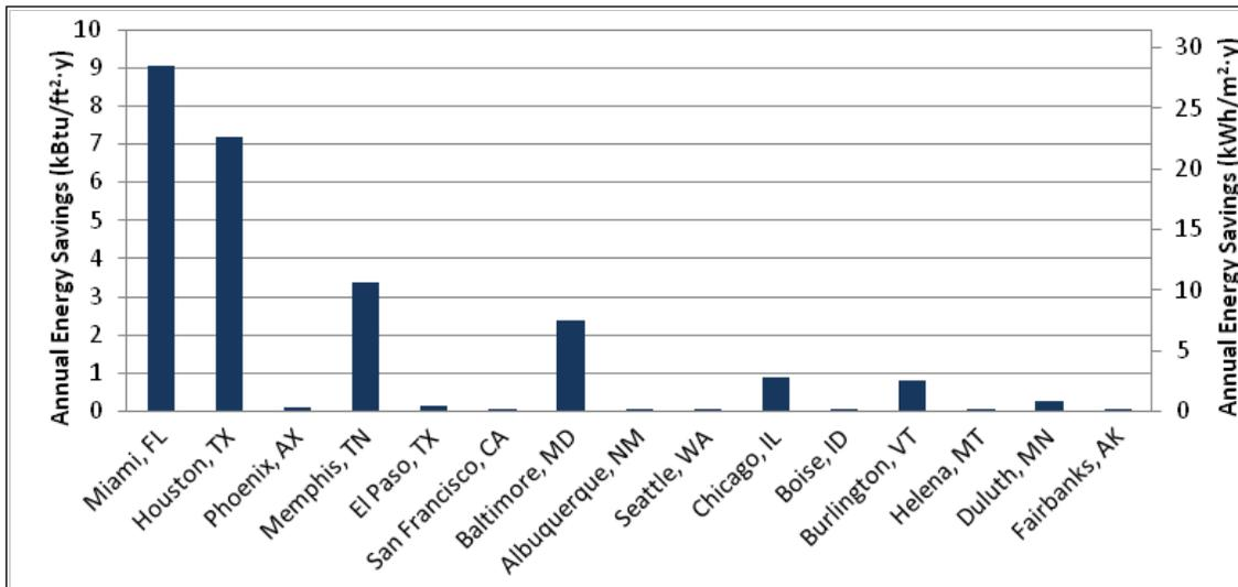
Figure 4.79. Annual energy savings for reheat using condenser waste heat.
