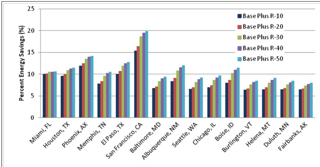
Figure 4.22. Percent energy savings for increased attic insulation and reduced building infiltration over the Standard 90.1-1989 baseline.
