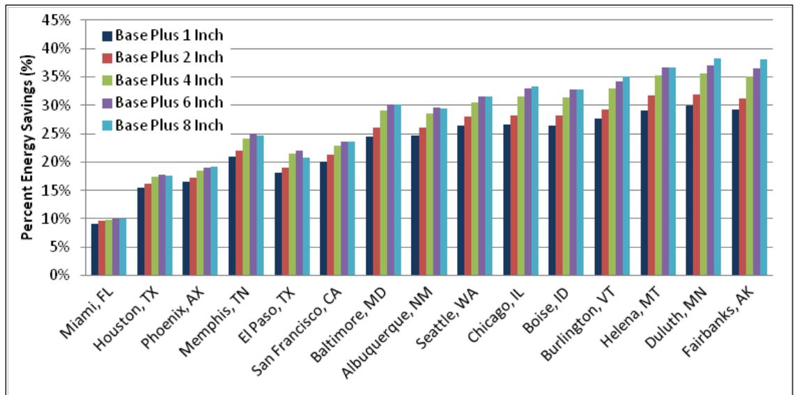
Figure 4.194. Percent energy savings for wall insulation and reduced infiltration over the no-insulation baseline.
