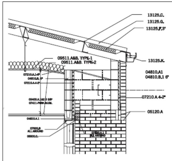
**Figure 7.24. Diagram showing construction of cool roof materials.**
