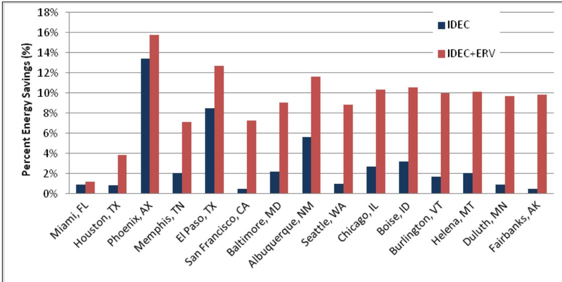
Figure 4.61. Percent energy savings for indirect evaporative cooling and indirect evaporative cooling with energy recovery.
