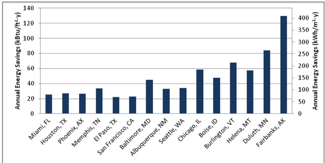
Figure 4.70. Annual energy savings for DOAS with radiant heating and cooling.
