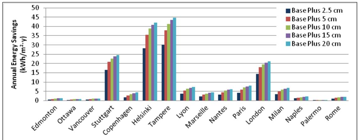
Figure 4.19. Energy savings for increased roof insulation and reduced infiltration over the Standard 90.1-1989 baseline – international locations.
