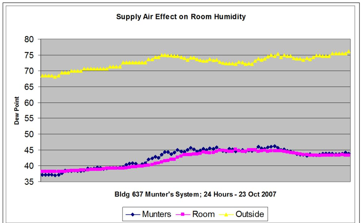
Figure 7.74. Modules A and B; effect of dry outdoor air on occupant room DPTs.
