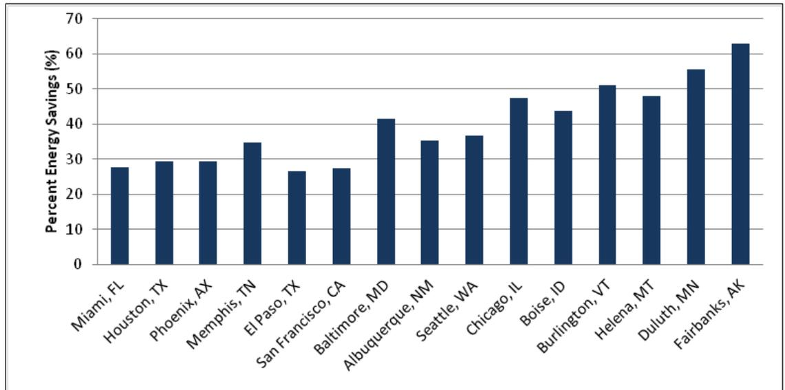
Figure 4.69. Percent energy savings for DOAS with radiant heating and cooling.
