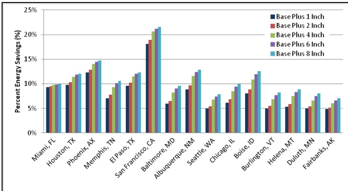
Figure 4.81. Percent energy savings for wall insulation and reduced infiltration over Standard 90.1-1989 baseline.
