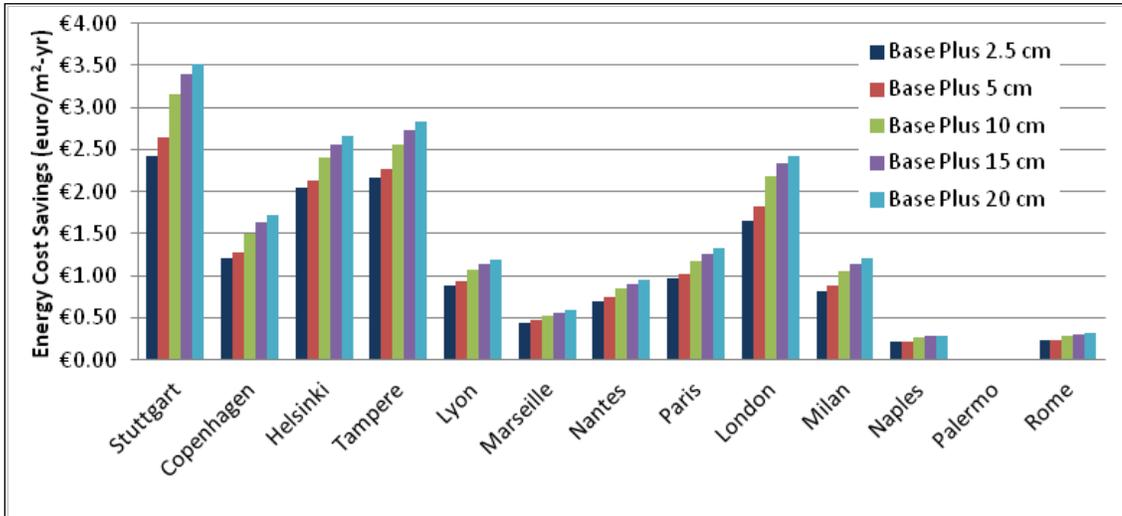
Figure 4.10. Energy cost savings for wall insulation and reduced infiltration over the Standard 90.1-1989 baseline - European locations.
