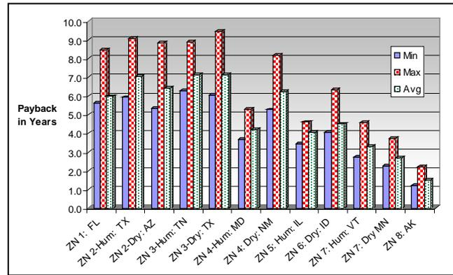
Figure 6.108. Estimated payback based on a 10 workstation system.
