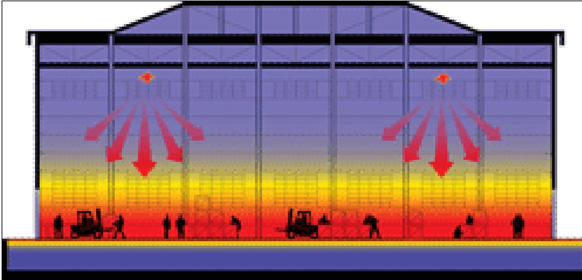
**Figure 7.19. How radiant heats at ground level.**
