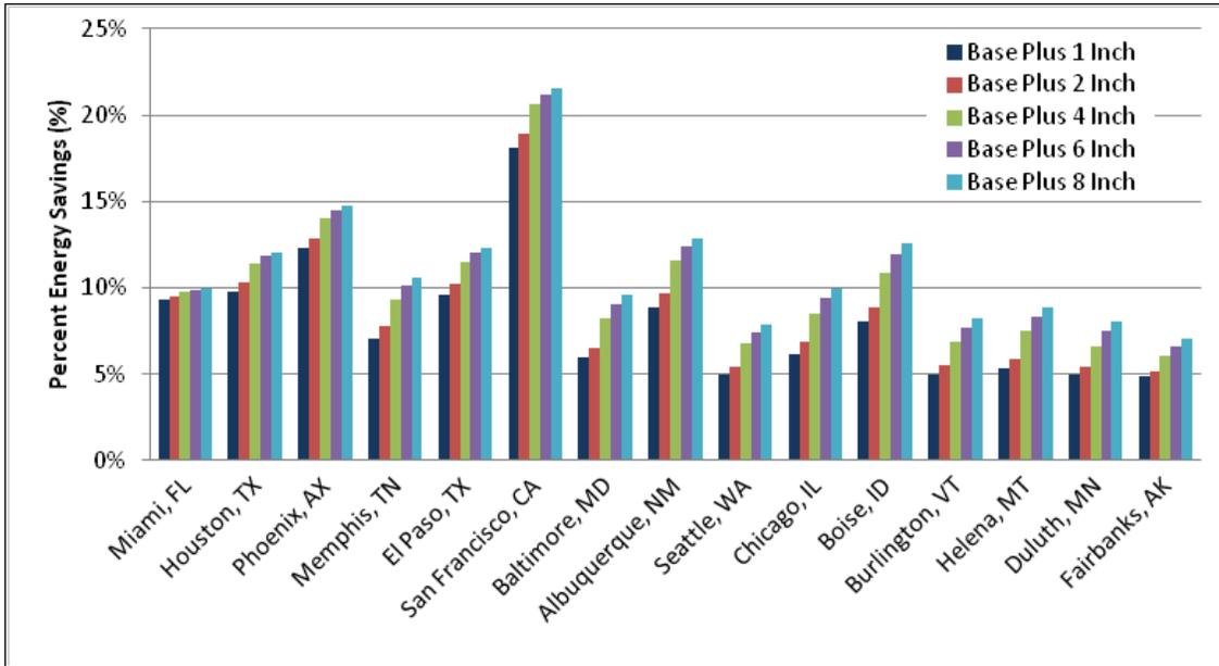
Figure 4.191. Percent energy savings for wall insulation and reduced infiltration over Standard 90.1-1989 baseline.
