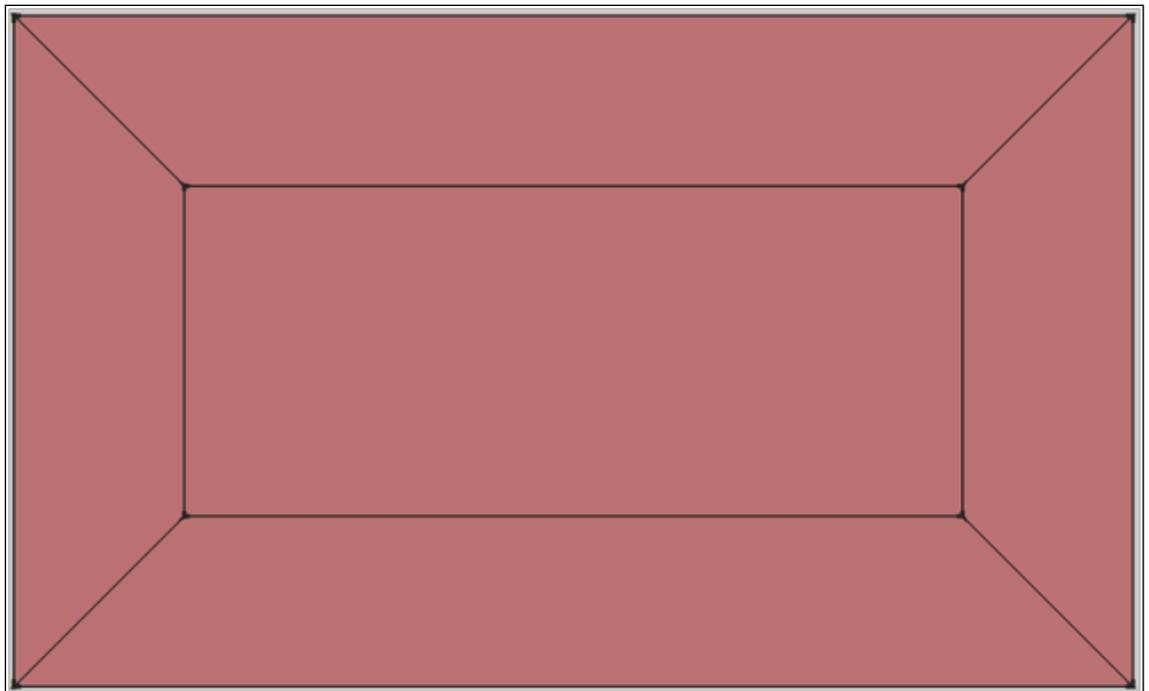
Figure 3.9. Thermal zoning repeated for each floor.
