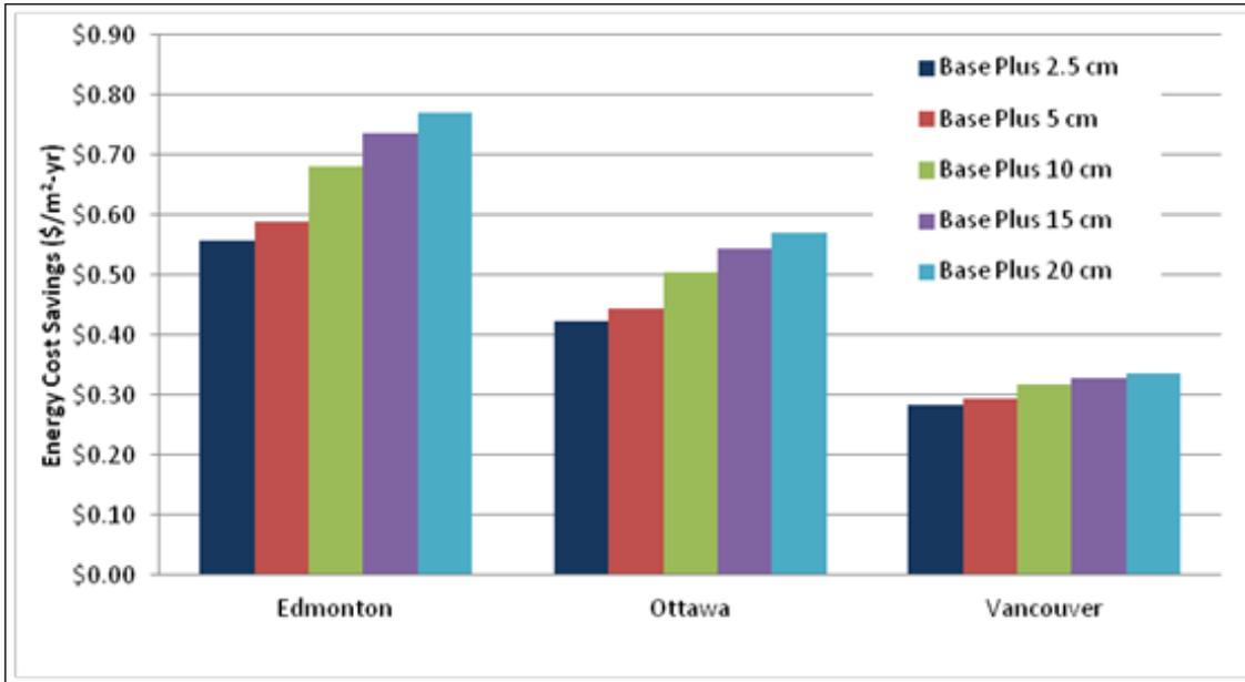
Figure 4.199. Energy cost savings for wall insulation and reduced infiltration over Standard 90.1-1989 baseline – Canadian locations.
