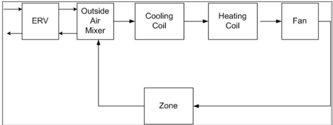
Figure 4.254. Schematic of the energy recovery ventilator model (credit: Kyle Benne).
