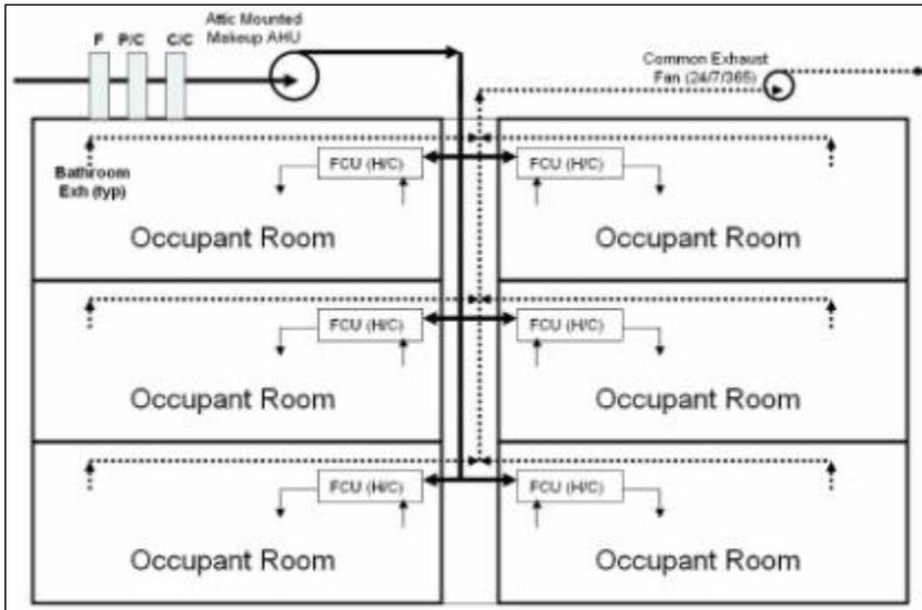
**Figure 7.61. Original system configuration (elevation view).**
