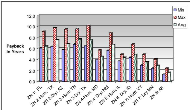
Figure 6.109. Estimated payback based on a 5 workstation system.
