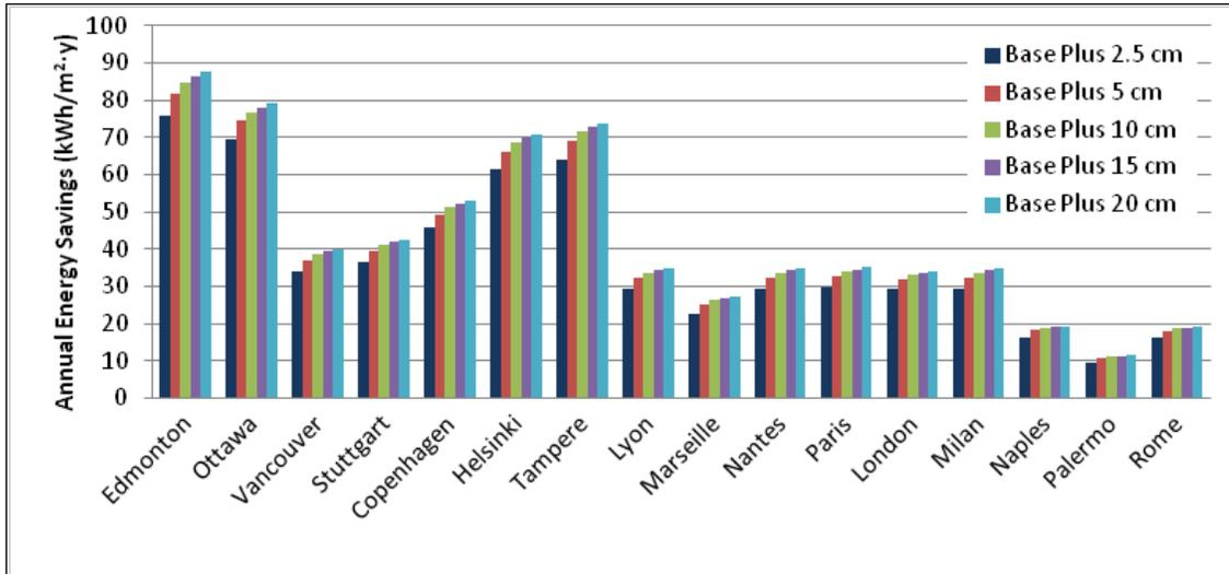
Figure 4.25. Annual energy savings for increased attic insulation and reduced building infiltration over the Standard 90.1-1989 baseline – International locations.
