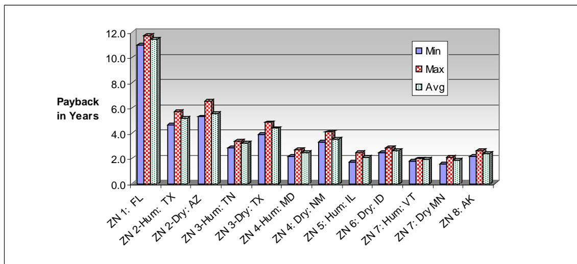
**Figure 6.63. Estimated payback for the radiant system.**
