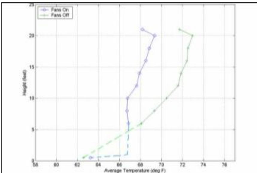
Figure 7.45. Average temperature over test duration versus height for Bethesda.
