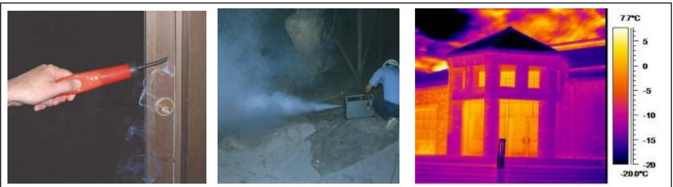
Figure 6.165. Smoke pencil (left) and theatrical fog (center) for leakage pathways; infrared thermography (right) for heat.
