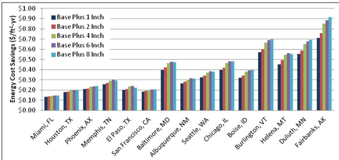
Figure 4.196. Energy cost savings for wall insulation and reduced infiltration over the no-insulation baseline.
