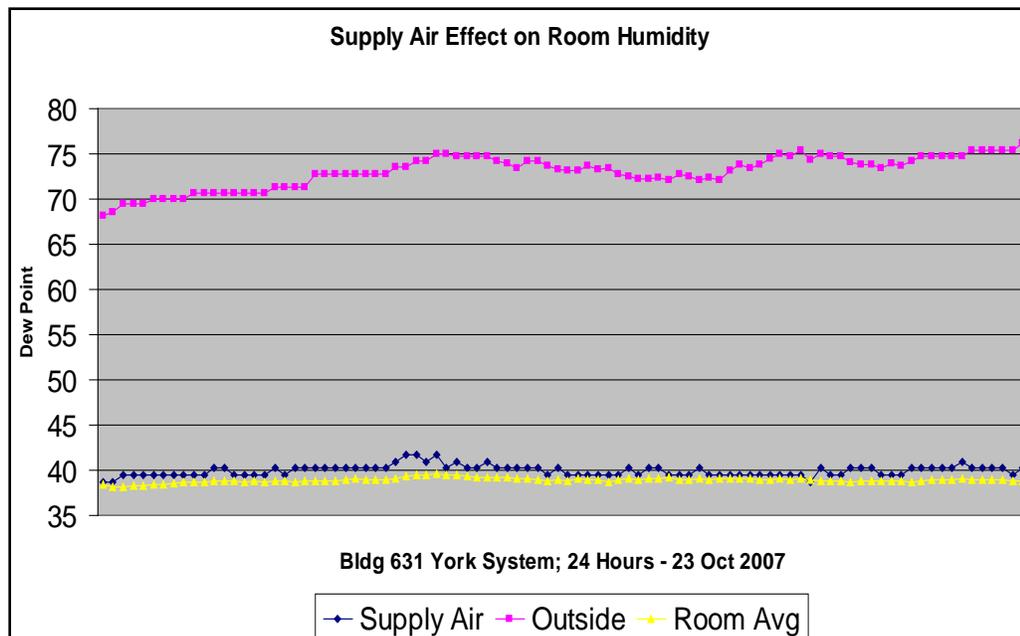
**Figure 7.65. Effect of dry outdoor air on occupant room relative humidity.**
