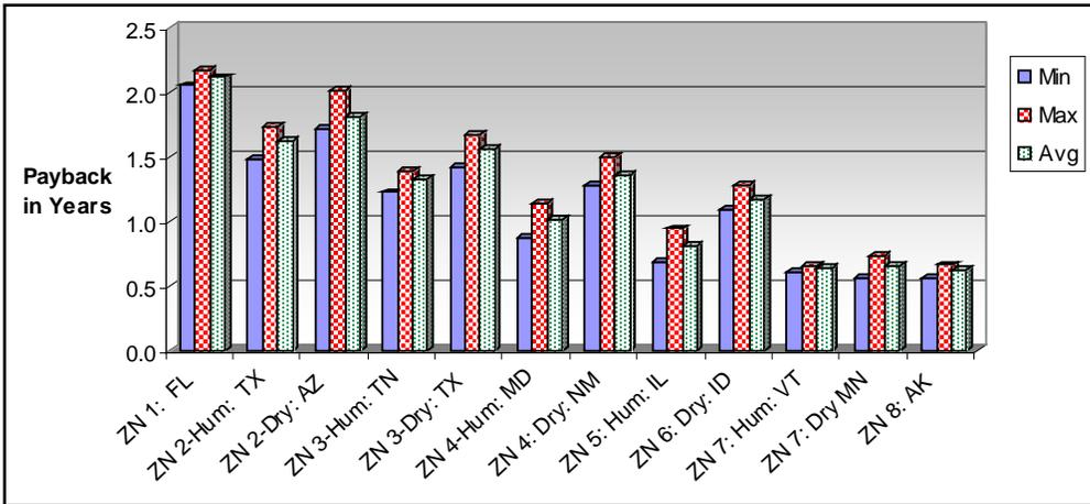
Figure 6.22. Estimated payback for system achieving 50% reduction of ventilation flow rate.
