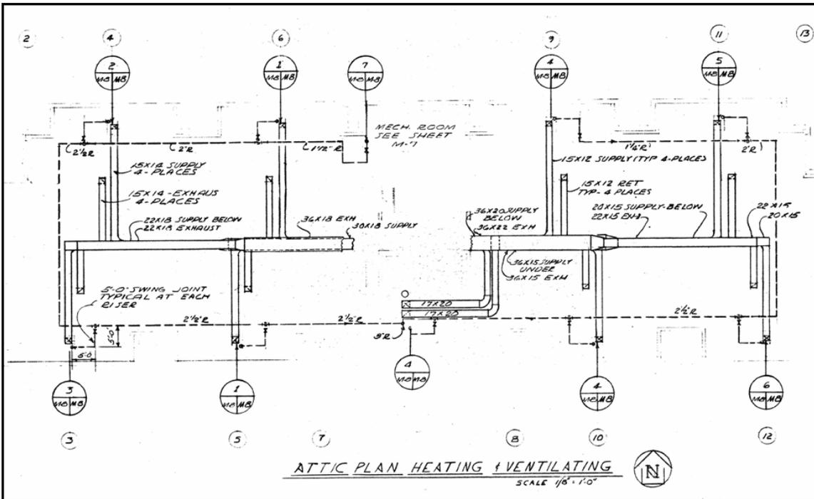
Figure 7.94. Bldg. 865 attic plan for ventilation ducts and hot water heating distribution loop.
