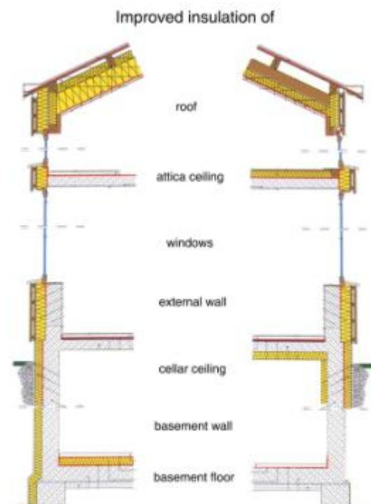
**Figure 6.123. Example of building insulation in Berlin. Two different applications of insulation material (marked in yellow) in the roof are: (left) all insulation in the roof (heated attic); (right) one insulation layer above the attic ceiling, another insulation layer in the below the rafters (attic as a buffer zone). The basement insulation on left includes radiant floor heating whereas on the right the insulation layer is under the basement ceiling (unheated basement).**
