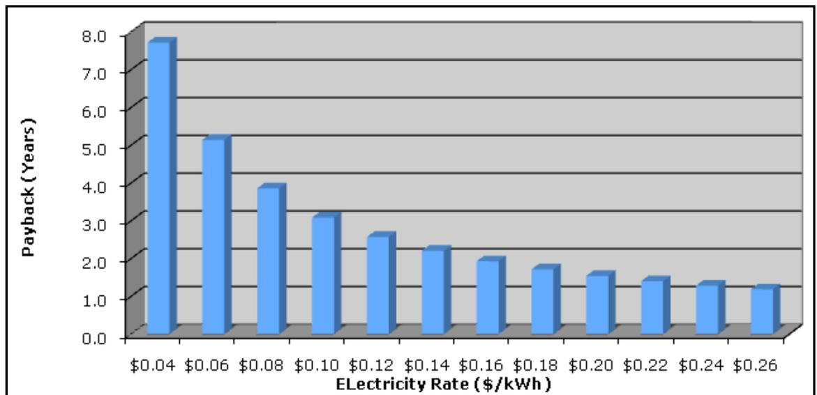
**Figure 6.84. Spectrally enhanced lighting simple payback.**
