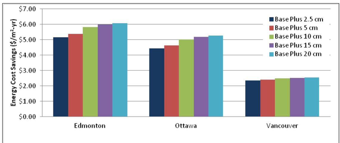
Figure 4.203. Energy cost savings for wall insulation and reduced infiltration over the no-insulation baseline – Canadian locations.
