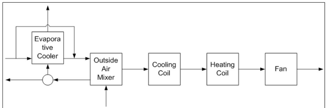
Figure 4.60. Schematic of the indirect evaporative cooling model (credit: Kyle Benne).
