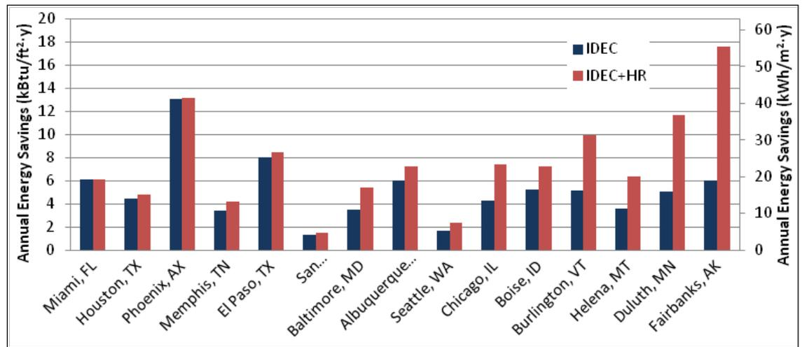
Figure 4.154. Annual energy savings for indirect evaporative cooling and indirect evaporative cooling with heat recovery.
