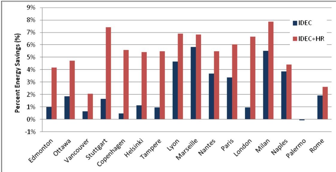
Figure 4.156. Percent energy savings for indirect evaporative cooling and indirect evaporative cooling with heat recovery – International locations.
