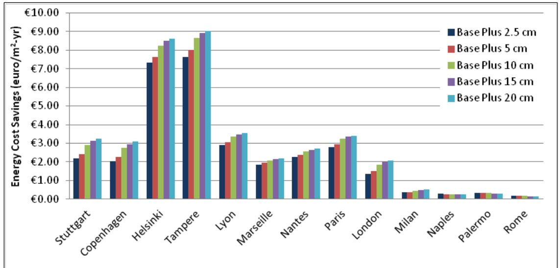
Figure 4.94. Energy cost savings for wall insulation and reduced infiltration over the no-insulation baseline – European locations.
