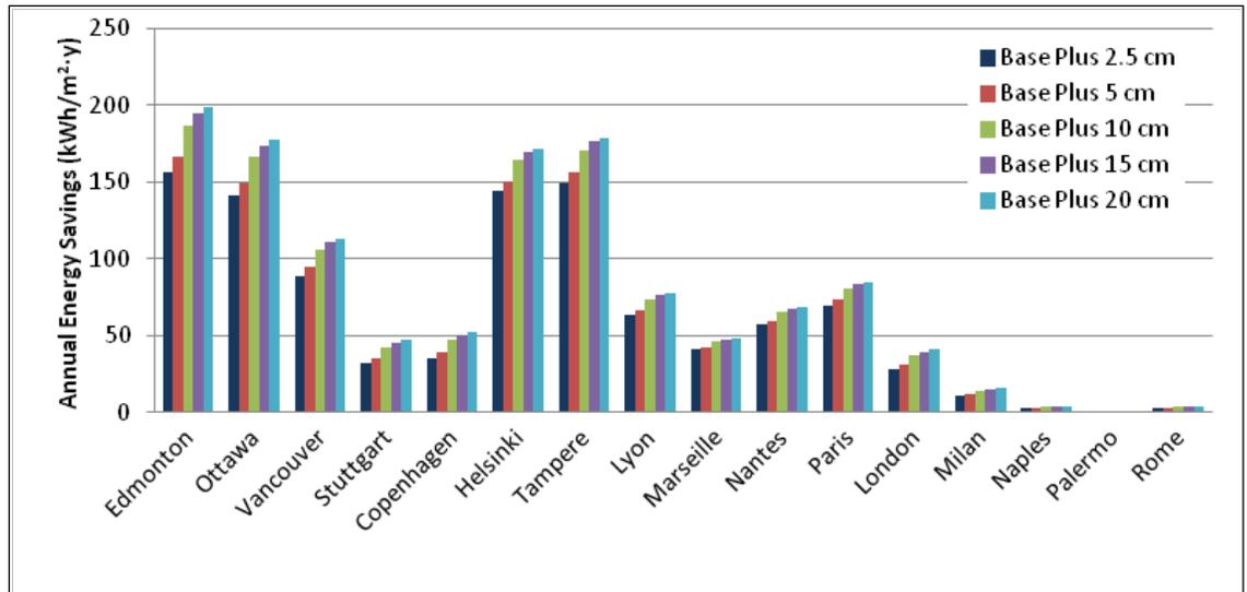
Figure 4.12. Energy savings for wall insulation and reduced infiltration over the no-insulation baseline- international locations.
