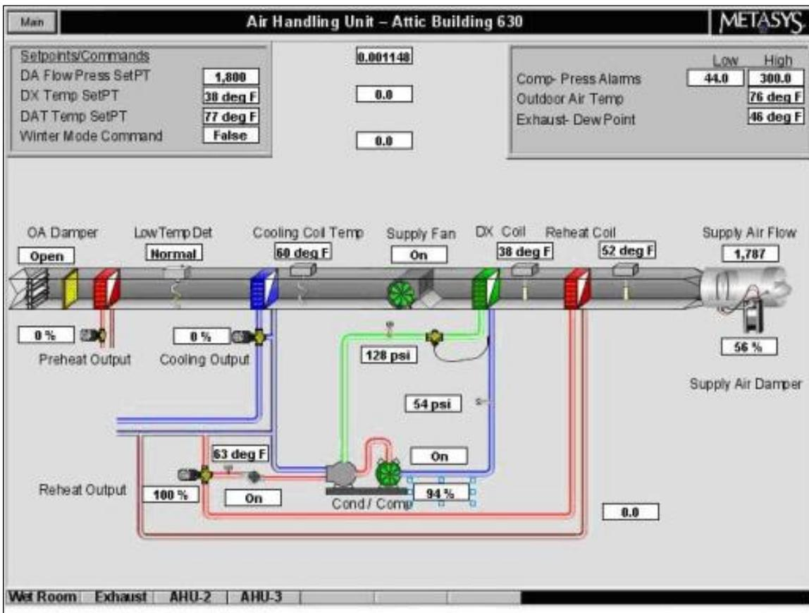
Figure 7.52. Screen capture of Bldg. 630 augmented DOAS makeup air unit schematic. Typical of three units installed in the attic of Bldg. 630.
