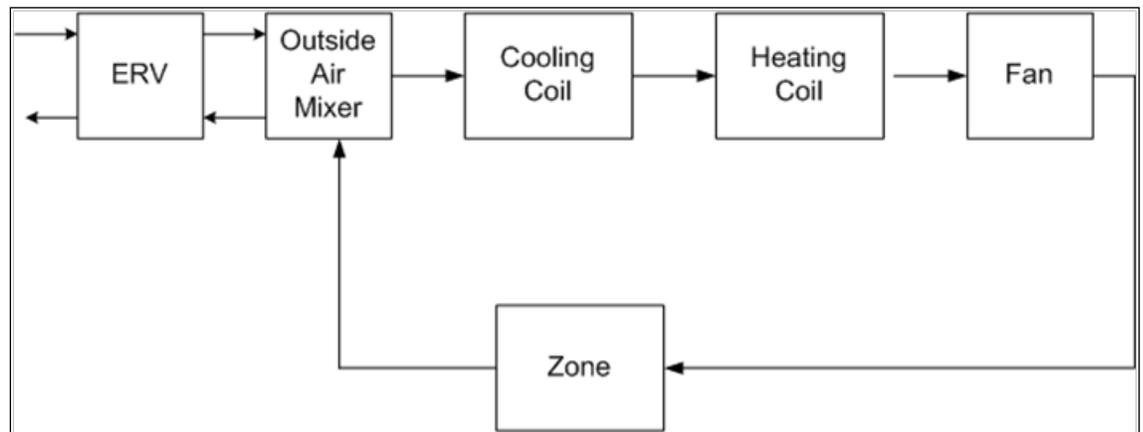
Figure 4.144. Schematic of the energy recovery ventilator model (credit: Kyle Benne).
