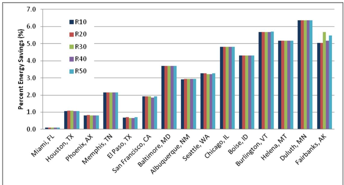
Figure 4.205. Percent energy savings for increased roof insulation.
