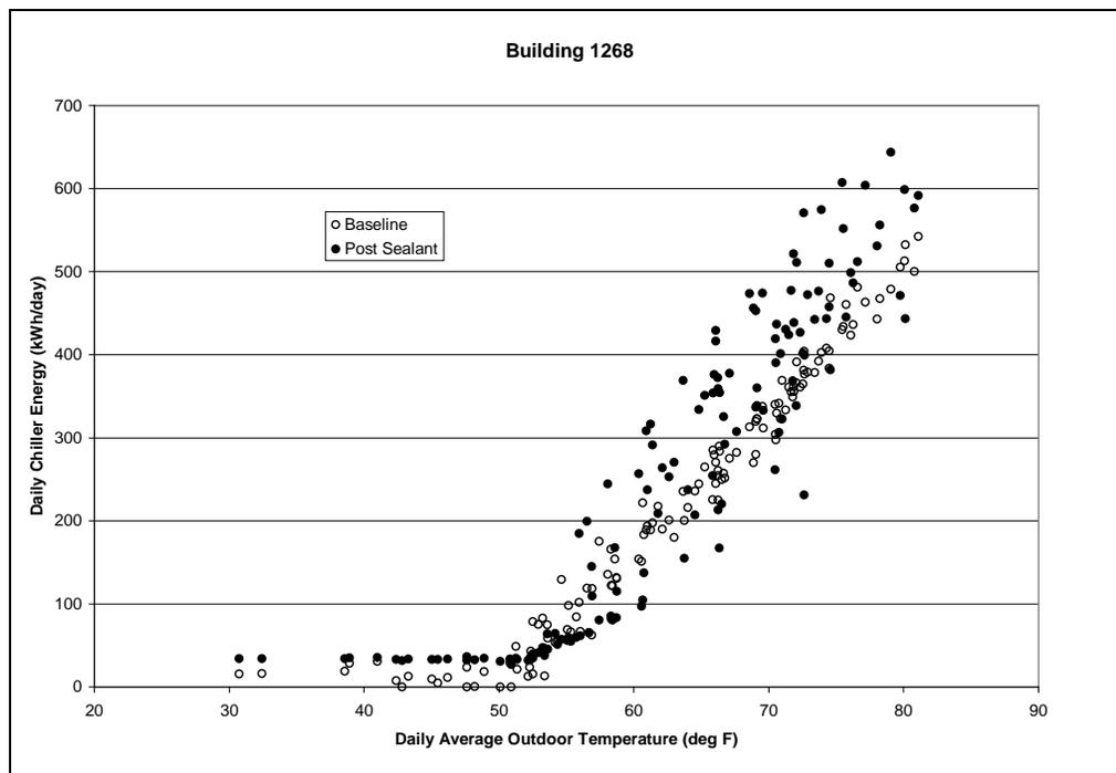
Figure 7.2. Bldg. 1268 chiller energy as a function of outdoor air temperature.
