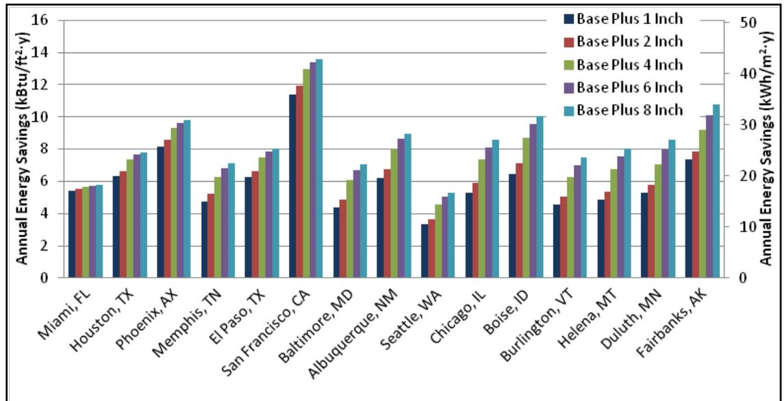
Figure 4.82. Energy savings for wall insulation and reduced infiltration over Standard 90.1-1989 baseline.
