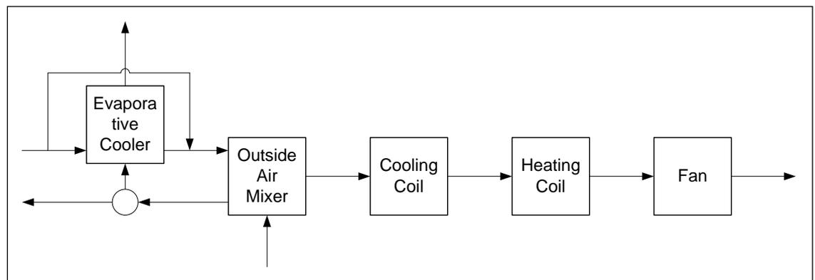
Figure 4.262. Schematic of the indirect evaporative cooling model (credit: Kyle Benne).
