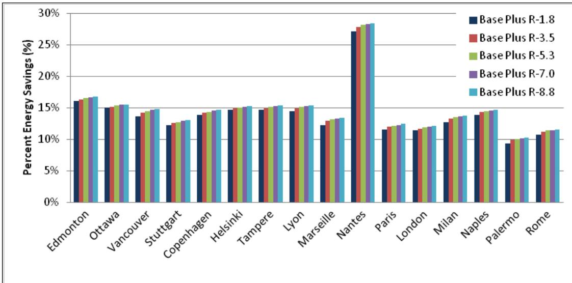
Figure 4.18. Percent energy savings for increased roof insulation and reduced infiltration over the Standard 90.1-1989 baseline – international locations.
