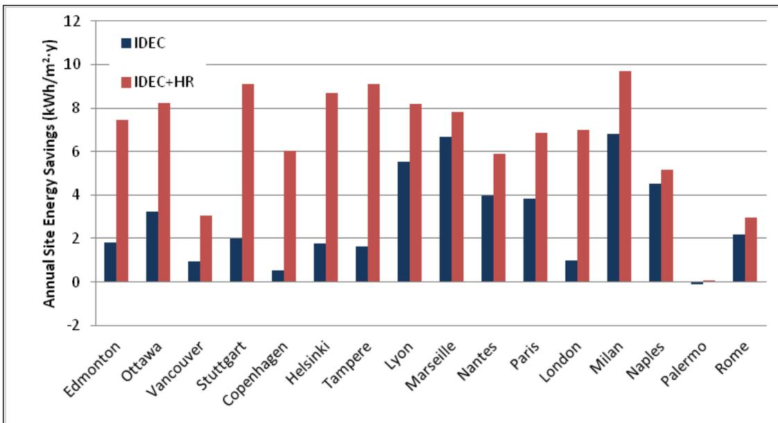
Figure 4.157. Annual energy savings for indirect evaporative cooling and indirect evaporative cooling with heat recovery – International locations.
