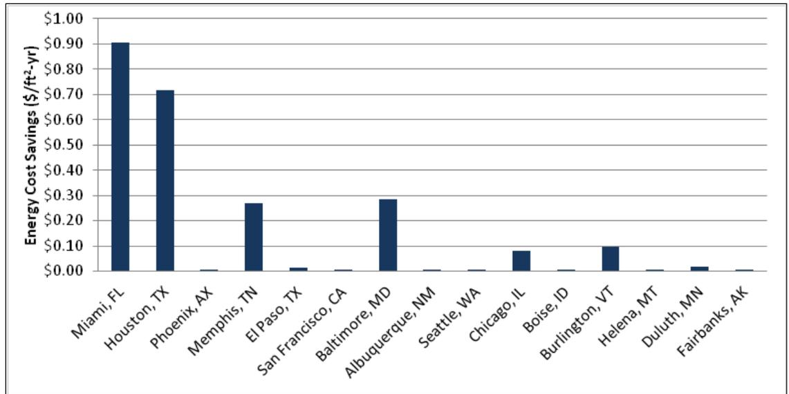
Figure 4.80. Annual energy cost savings for reheat using condenser waste heat.
