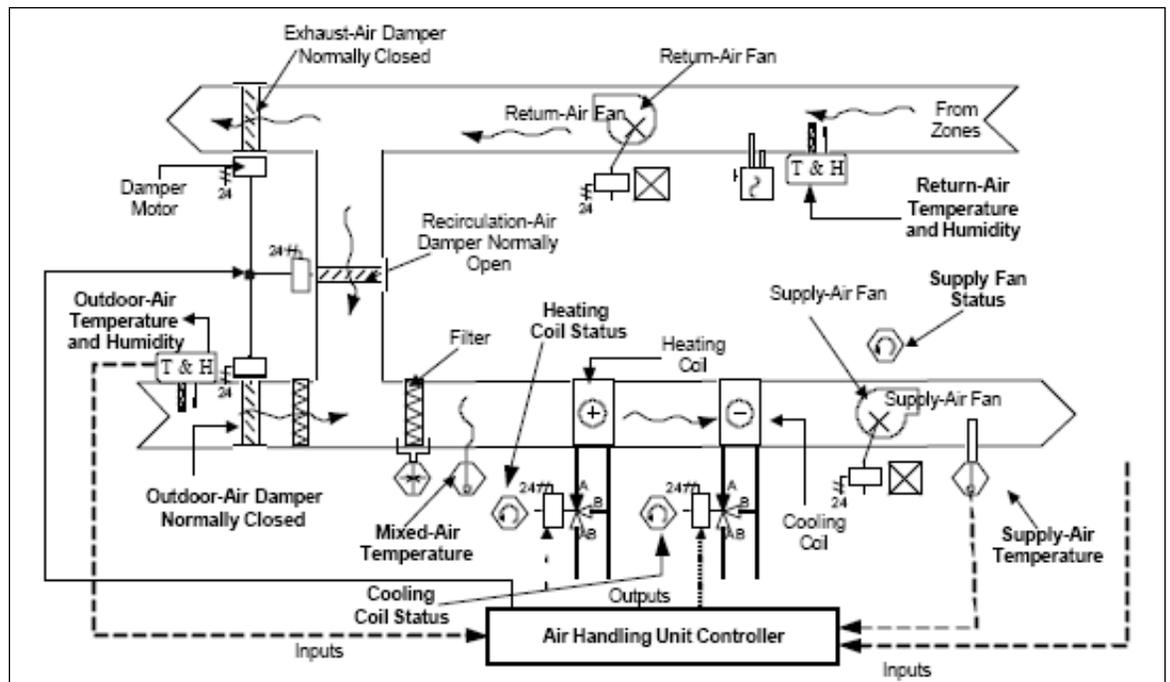
Figure 7.153. Air handler showing the sensor locations.
