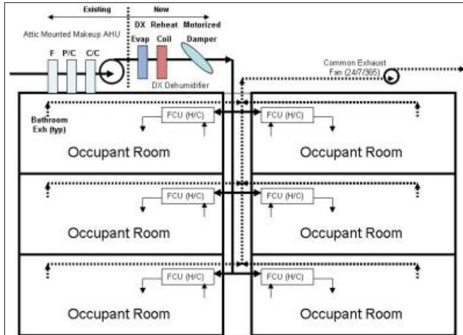
Figure 7.53. New Bldg. 630 DOAS system configuration (elevation view).
