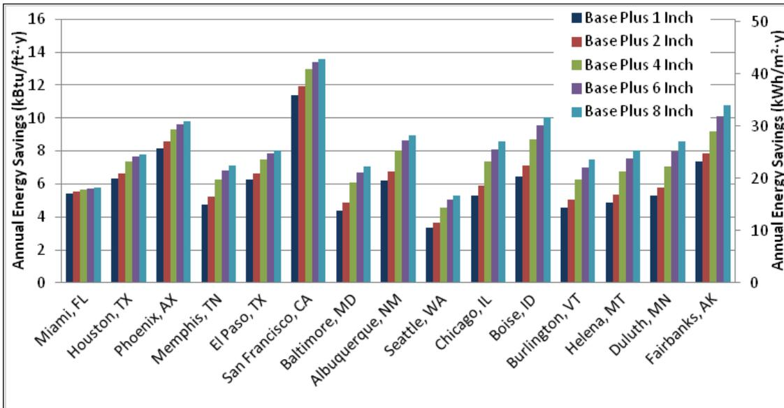
Figure 4.192. Energy savings for wall insulation and reduced infiltration over Standard 90.1-1989 baseline.
