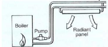
**Figure 6.59. Low intensity radiant heater.**
