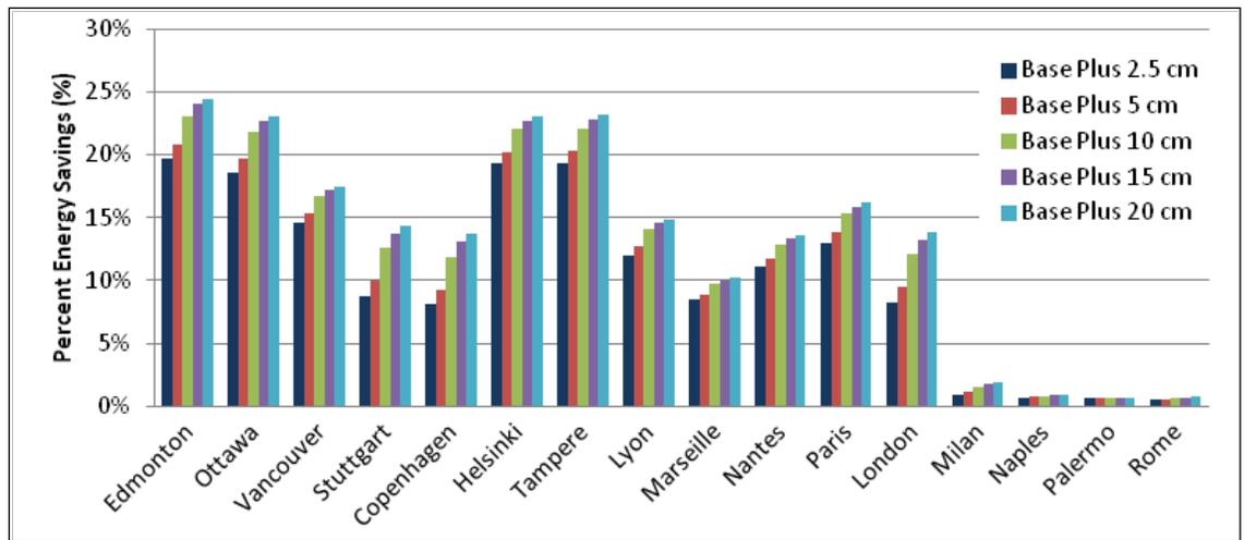
Figure 4.201. Percent energy savings for wall insulation and reduced infiltration over the no-insulation baseline – International locations.
