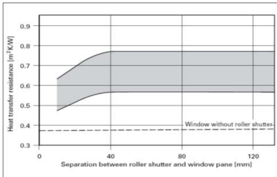
**Figure 6.150. Thermal resistance versus window-shutter gap (outer edge of window pane to inner edge of shutter).**
