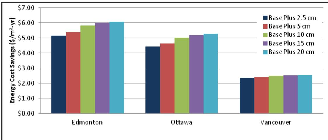
Figure 4.93. Energy cost savings for wall insulation and reduced infiltration over the no-insulation baseline – Canadian locations.
