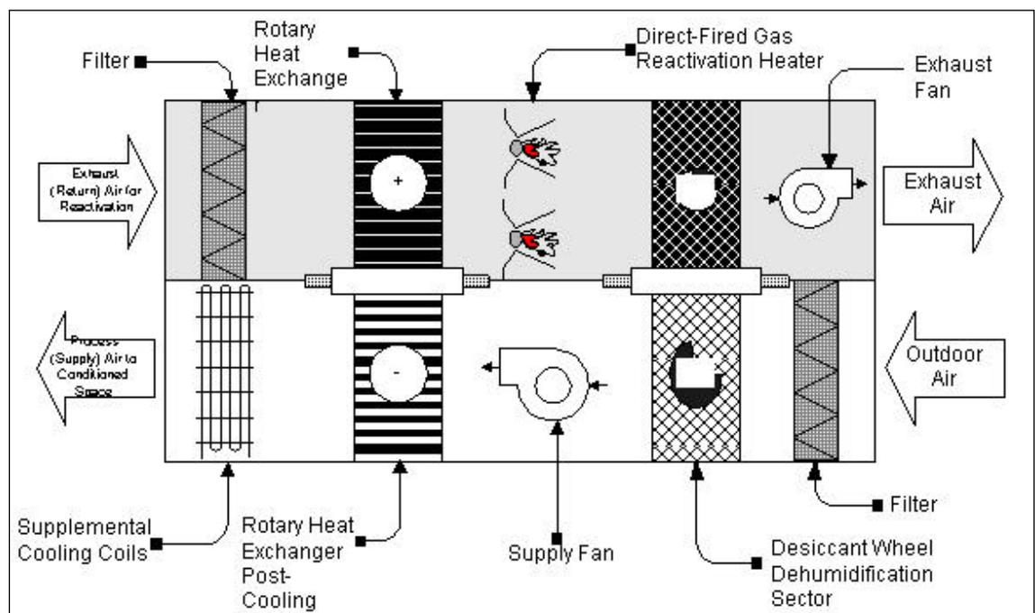
**Figure 7.40. Schematic of the two-wheel desiccant system.**
