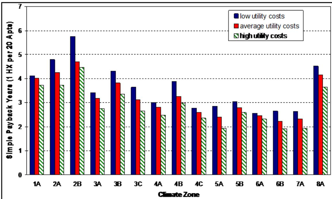
Figure 6.145. Simple payback, years with low, average and high utility rates for the heat recovery system servicing 20 apartments.
