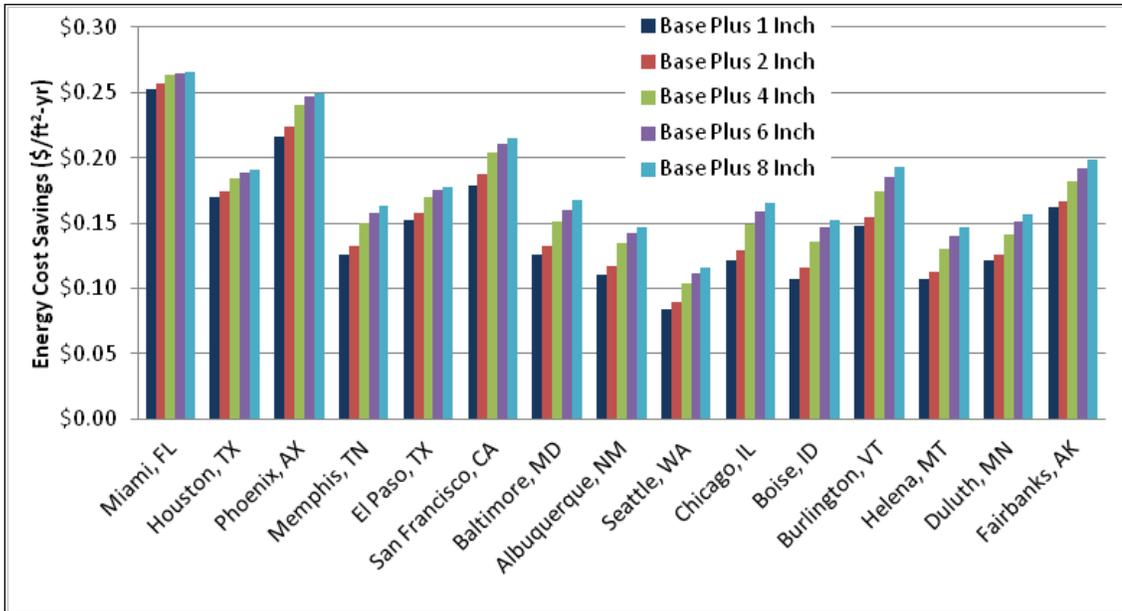
Figure 4.3. Energy cost savings for wall insulation and reduced infiltration over Standard 90.1-1989 baseline.
