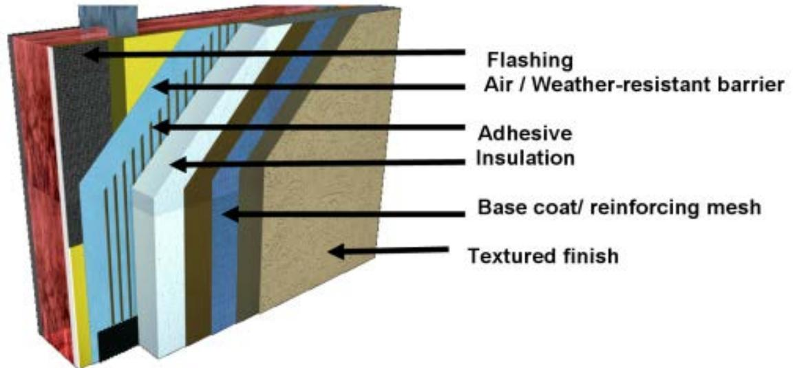
Figure 6.124. EIFS construction with drainage.
