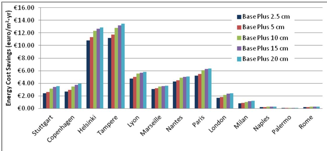
Figure 4.14. Energy cost savings for wall insulation and reduced infiltration over the no-insulation baseline- European locations.
