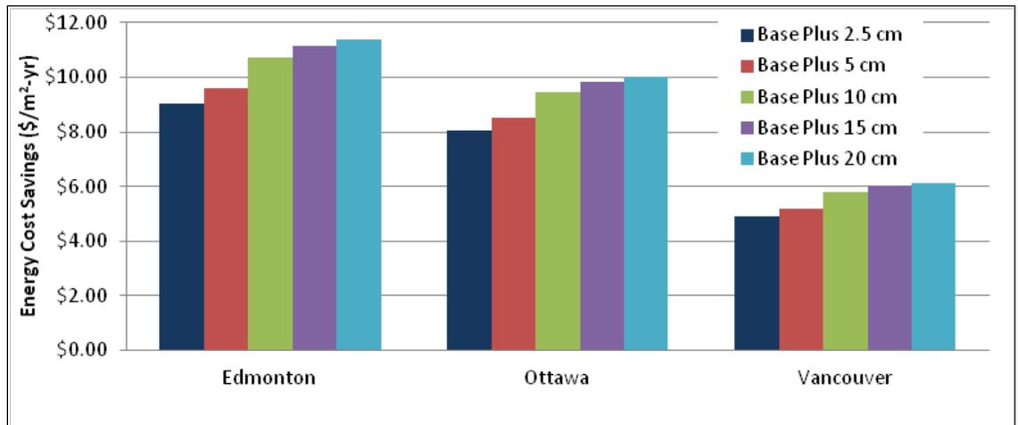
Figure 4.13. Energy cost savings for wall insulation and reduced infiltration over the no-insulation baseline- Canadian locations.
