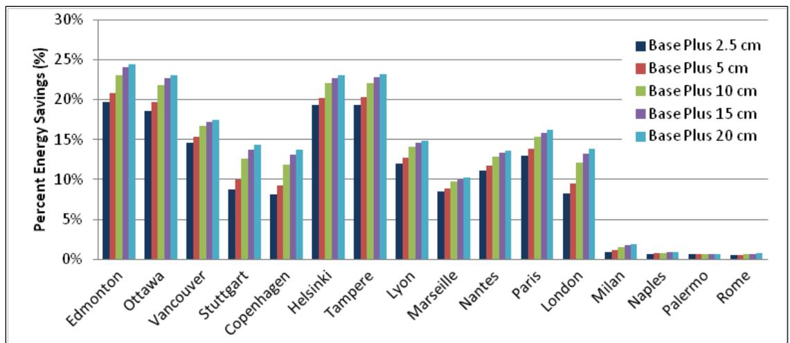
Figure 4.91. Percent energy savings for wall insulation and reduced infiltration over the no-insulation baseline – International locations.
