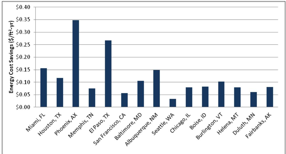
Figure 4.162. Annual energy cost savings for hybrid evaporative cooling.
