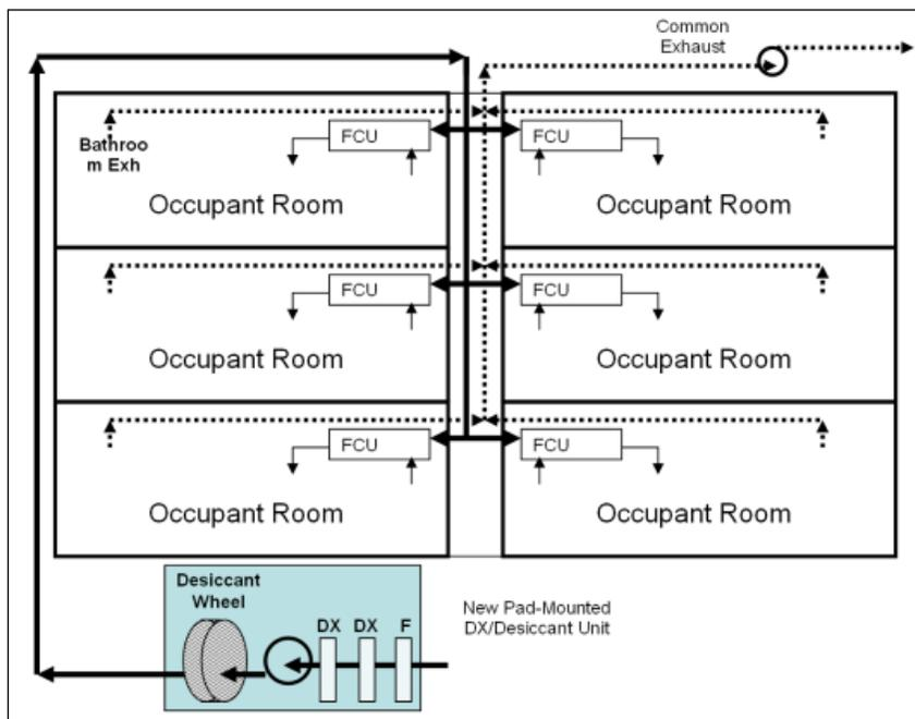
Figure 7.71. New Bldg. 637 DOAS system configuration (elevation view).
