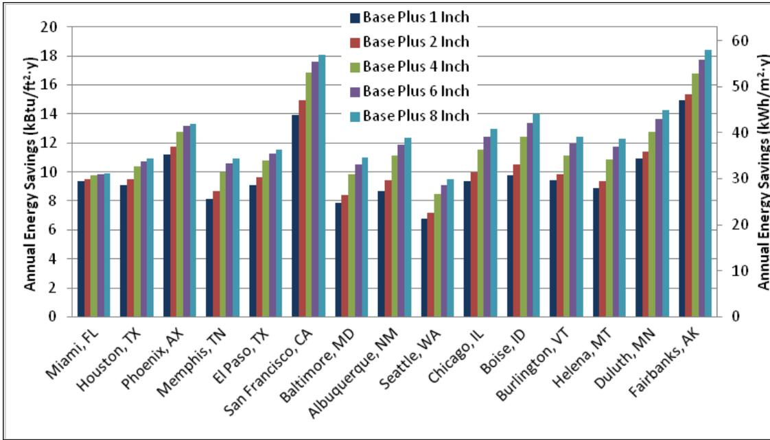
Figure 4.2. Energy savings for wall insulation and reduced infiltration over Standard 90.1-1989 baseline.
