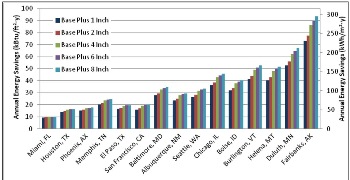
Figure 4.5. Energy savings for wall insulation and reduced infiltration over the no-insulation baseline.
