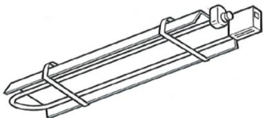
**Figure 6.60. Low intensity radiant heater.**
