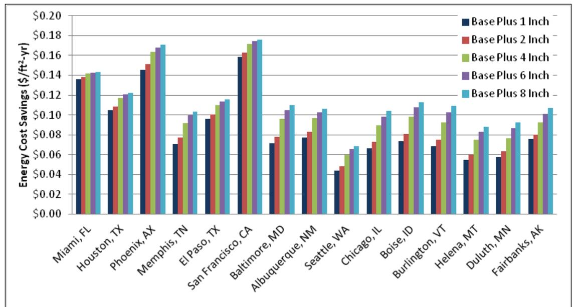
Figure 4.83. Energy cost savings for wall insulation and reduced infiltration over Standard 90.1-1989 baseline.
