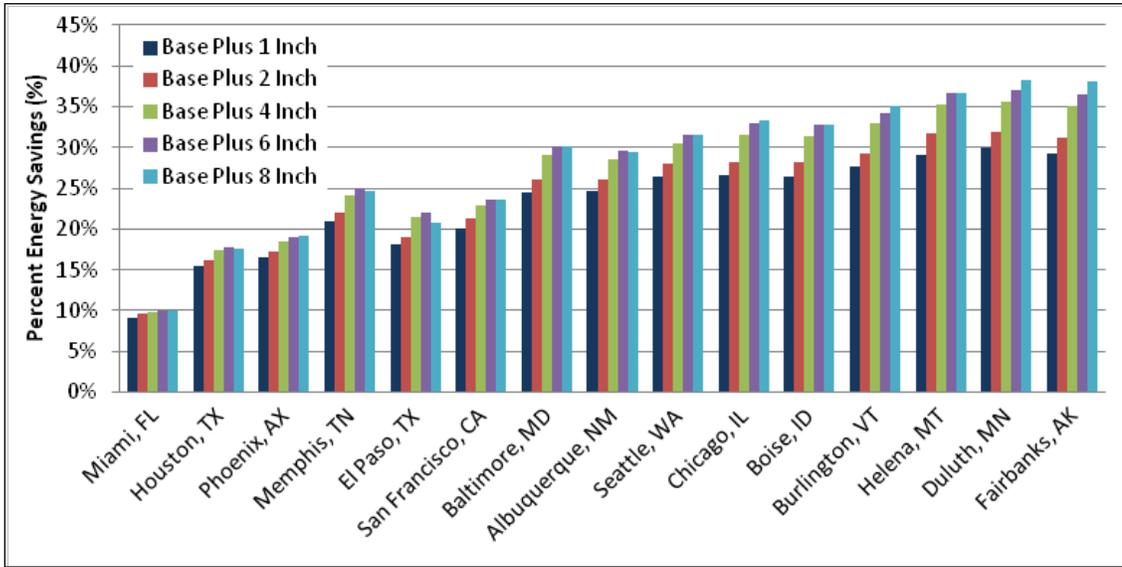
Figure 4.84. Percent energy savings for wall insulation and reduced infiltration over the no-insulation baseline.
