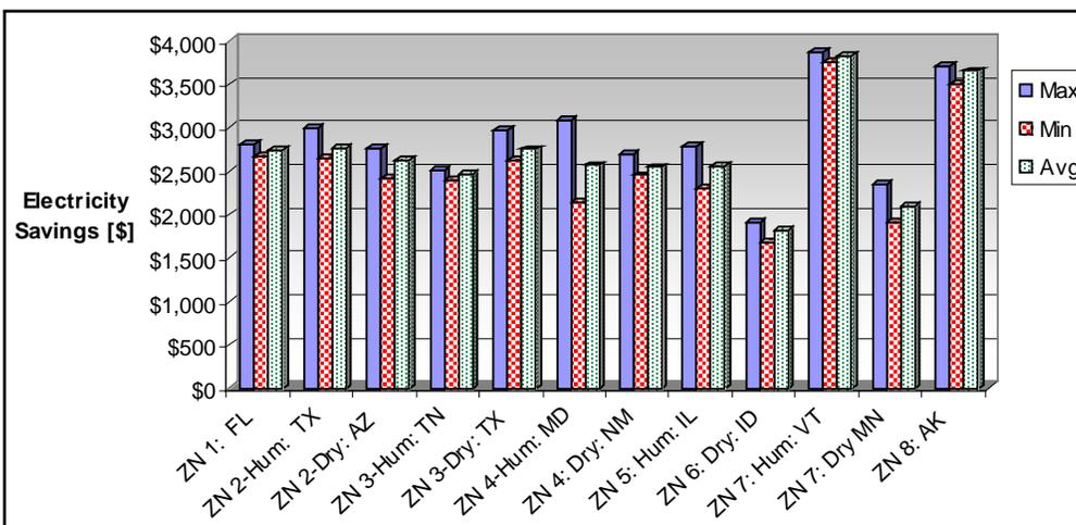
Figure 6.24. Estimated annual electricity savings for system achieving 25% reduction of ventilation flow rate.
