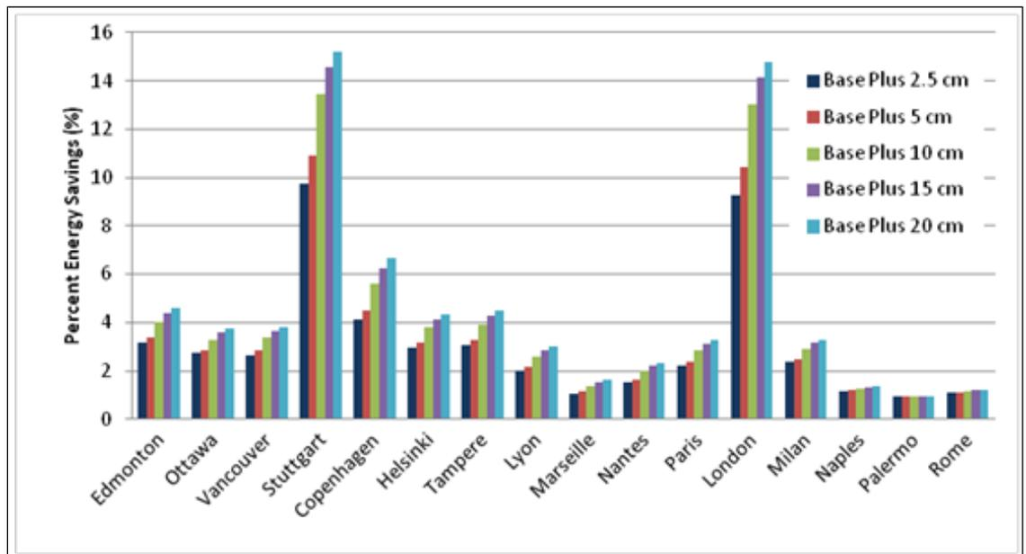
Figure 4.87. Percent energy savings for wall insulation and reduced infiltration over the standard baseline – international locations.
