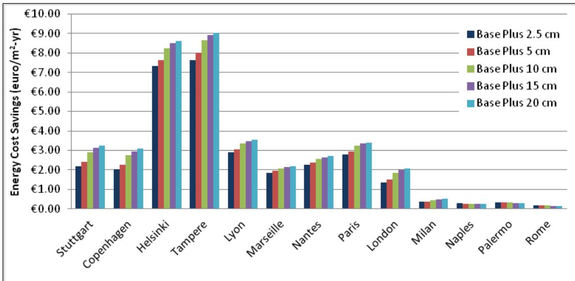
Figure 4.204. Energy cost savings for wall insulation and reduced infiltration over the no-insulation baseline – European locations.
