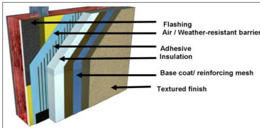
**Figure 6.171. EIFS construction with drainage.**
