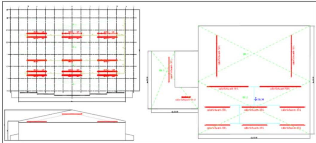
**Figure 7.99.** Layout of heater placement in Hangar 2310 and warehouse in Kaiserslautern.
