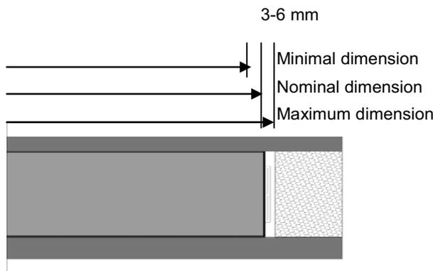
*Figure 76: Tolerances in VIP integrated building components*
