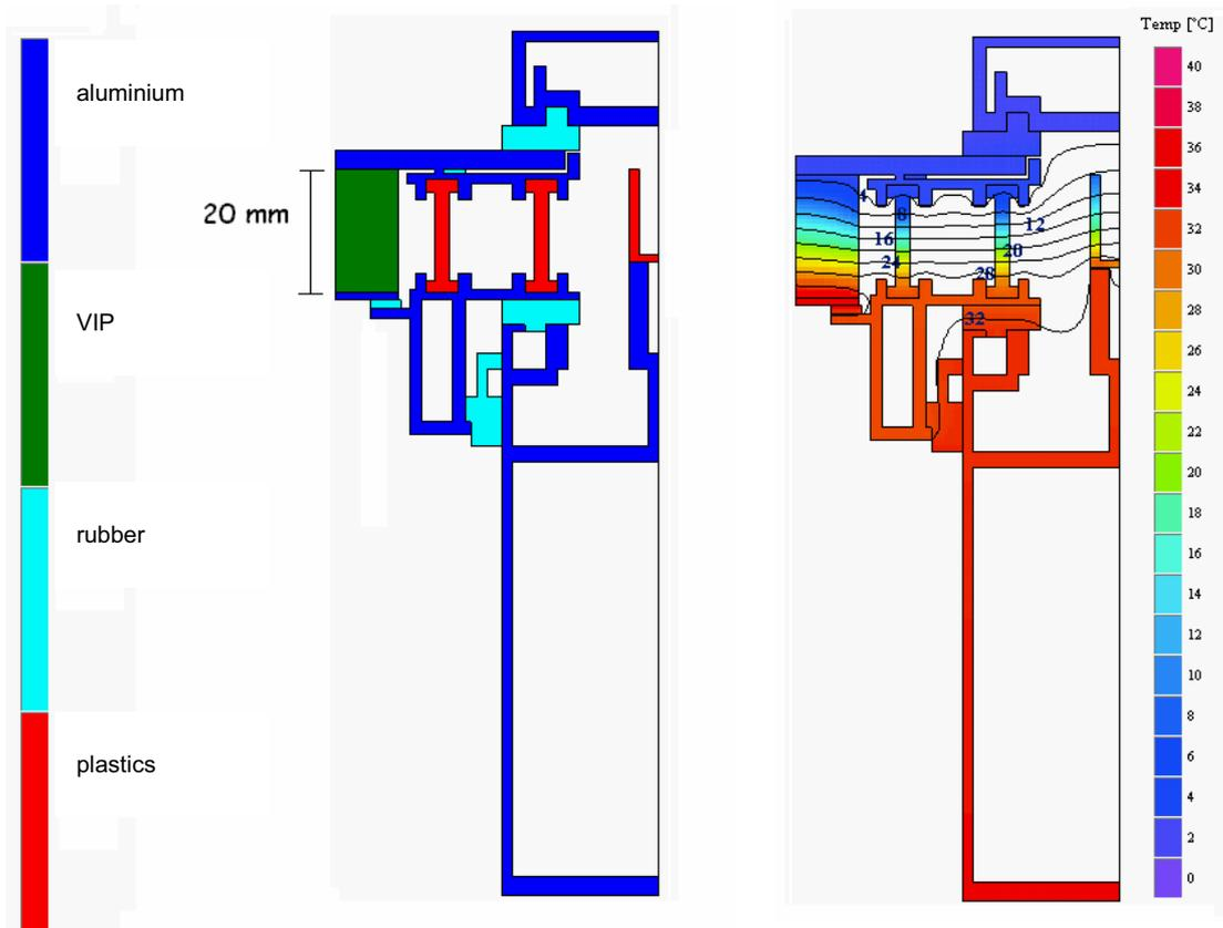
Figure 59: Left: Cross-section of the façade element without the radiator. The jamb-crossbar construction can be seen on the right hand side. The VIP is cut off on the left side. Right: A Finite-Element-Program was used to simulate the temperatures shown in this cross-section. The temperatures are colour-coded and the isotherms drawn in.
