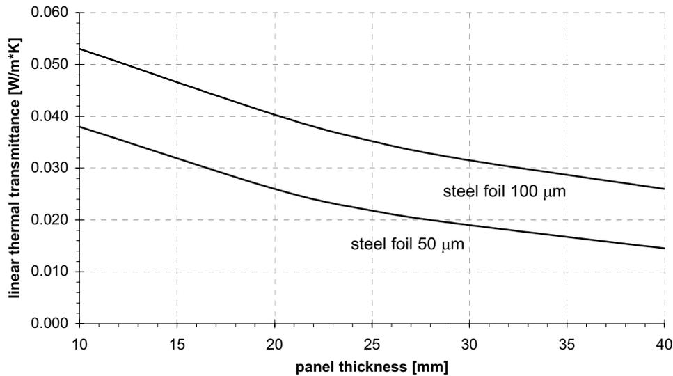
Figure 9: The effects of panel thickness and foil thickness on the linear thermal transmittance due to thermal bridging for a stainless steel foil ( $\lambda_{foi} = 25 \text{ W/(m}\cdot\text{K)}$ ;
