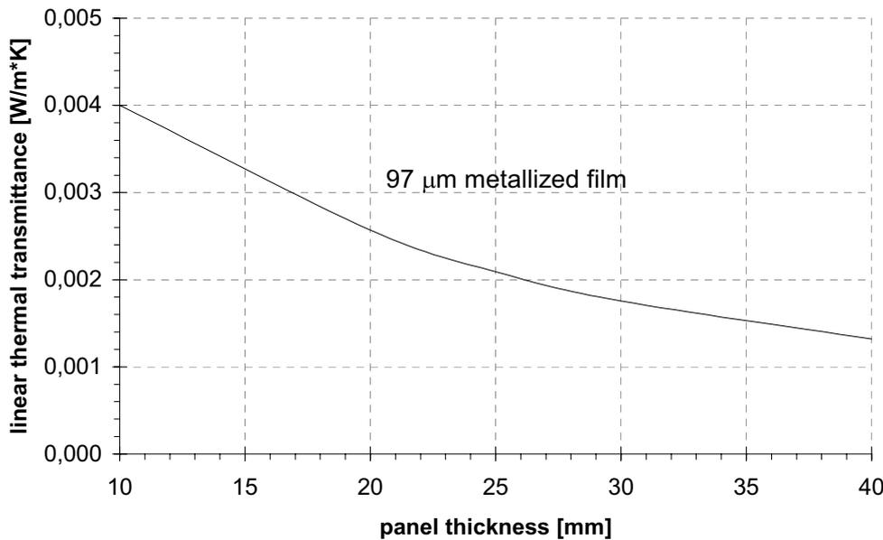
Figure 10: The effects of panel thickness on the linear thermal transmittance due to thermal bridging for a three layer metallized film;  $\lambda_{cop} = 4 \cdot 10^{-3} \text{ W/(m}\cdot\text{K)}$ ), based on numerical calculation
