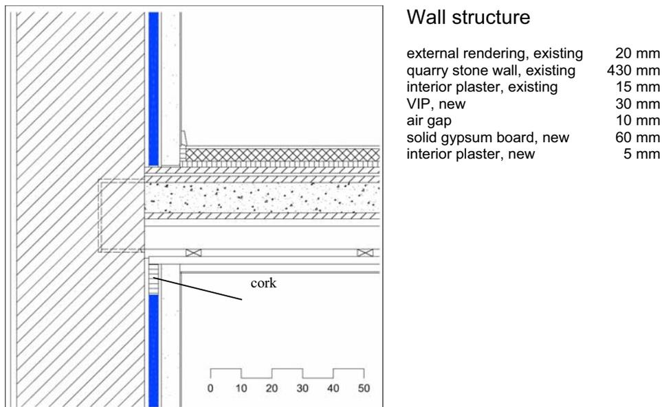
Figure 71: Section through the support of the ceiling
