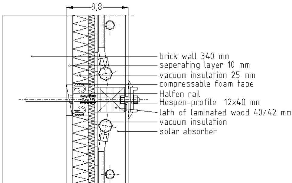
Figure 49: Cross-section of the south wall
